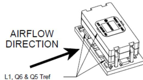
**Figure 50. Preferred airflow direction and location of hotspot of the module (T<sub>ref</sub>).**
