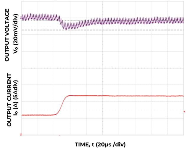
Figure 4. Transient Response to Dynamic Load Change from 50% to 100% on one output at 12V<sub>in</sub>, C<sub>out</sub>=2x47μF+7x330μF, C<sub>Tune</sub>=12nF, R<sub>Tune</sub>=300Ω
