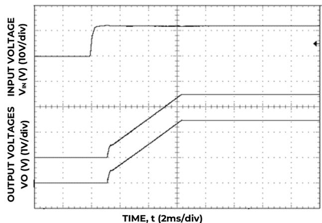
Figure 24. Typical Start-up Using Input Voltage (V<sub>IN</sub> = 12V, I<sub>o</sub> = I<sub>o1,max</sub>, I<sub>o2,max</sub>).
