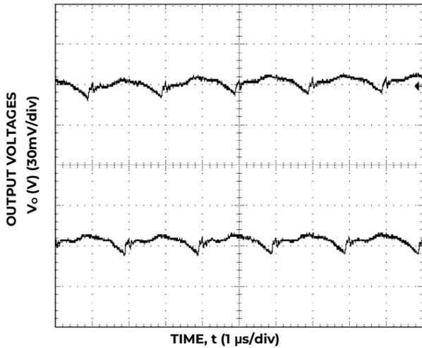
Figure 3. Typical output ripple and noise (C<sub>o</sub>= 2×0.1μF+2×47μF ceramic, V<sub>IN</sub> = 12V, I<sub>o</sub> = I<sub>o1,max</sub>, I<sub>o2,max</sub>).
