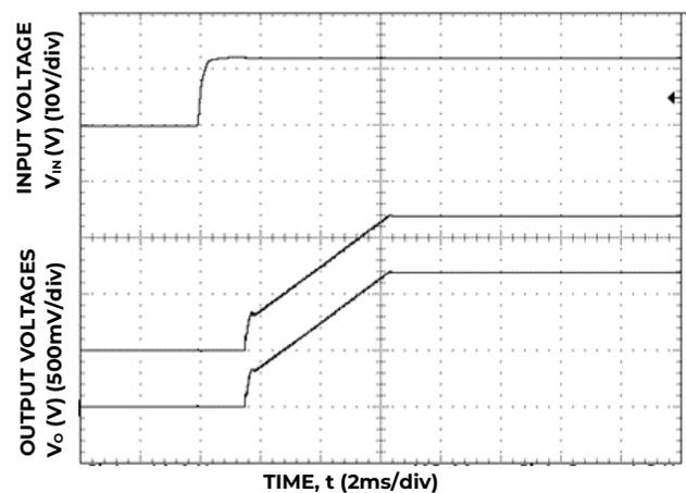
Figure 12. Typical Start-up Using Input Voltage (V<sub>in</sub> = 12V, I<sub>o</sub> = I<sub>o1,max</sub>, I<sub>o2,max</sub>).
