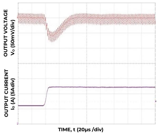
Figure 28 Transient Response to Dynamic Load Change on one output from 50% to 100% at 12Vin,  $C_{out} = 3 \times 47\mu\text{F} + 1 \times 330\mu\text{F}$ ,  $C_{Tune} = 1200\text{pF}$  &  $R_{Tune} = 300\Omega$
