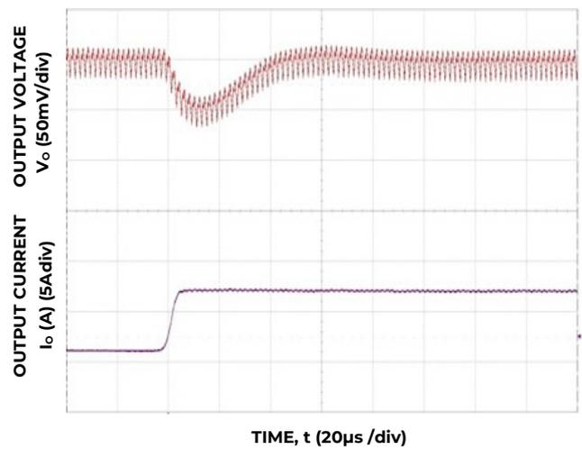
Figure 22. Transient Response to Dynamic Load Change from 50% to 100% on one output at 12V<sub>in</sub>, C<sub>out</sub>=3x47uF+3x330uF, C<sub>Tune</sub>=1500pF & R<sub>Tune</sub>=300Ω
