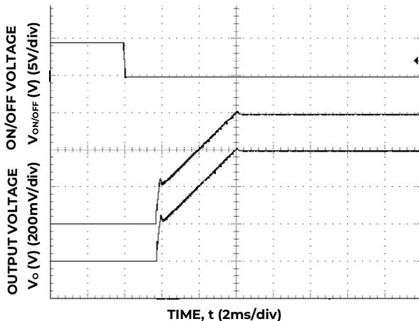
Figure 5. Typical Start-up Using On/Off Voltage (V<sub>in</sub>=12V, I<sub>o</sub> = I<sub>o1,max</sub>, I<sub>o2,max</sub>).
