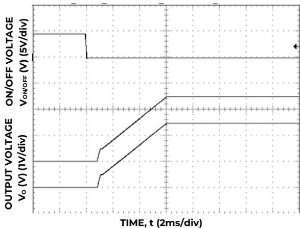
Figure 23. Typical Start-up Using On/Off Voltage (V<sub>IN</sub>=12V, I<sub>o</sub> = I<sub>o1,max</sub>, I<sub>o2,max</sub>).
