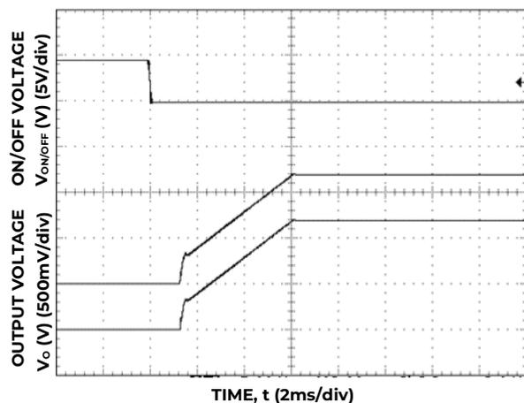
Figure 11. Typical Start-up Using On/Off Voltage (V<sub>in</sub>=12V, I<sub>o</sub> = I<sub>o1,max</sub>, I<sub>o2,max</sub>).
