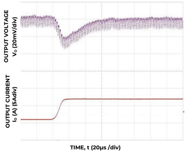
Figure 10. Transient Response to Dynamic Load Change from 50% to 100% on one output at 12V<sub>in</sub>, C<sub>out</sub>=3x47uF+3x330uF, C<sub>Tune</sub>=2700pF & R<sub>Tune</sub>=300Ω
