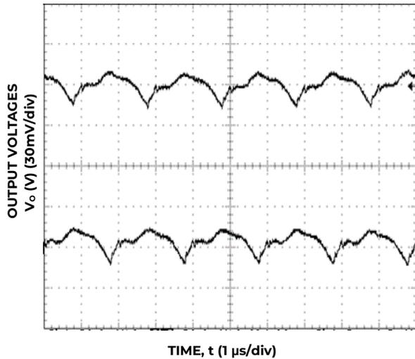
Figure 9. Typical output ripple and noise (C<sub>o</sub>= 2×0.1uF+2×47uF ceramic, V<sub>in</sub> = 12V, I<sub>o</sub> = I<sub>o1,max</sub>, I<sub>o2,max</sub>).
