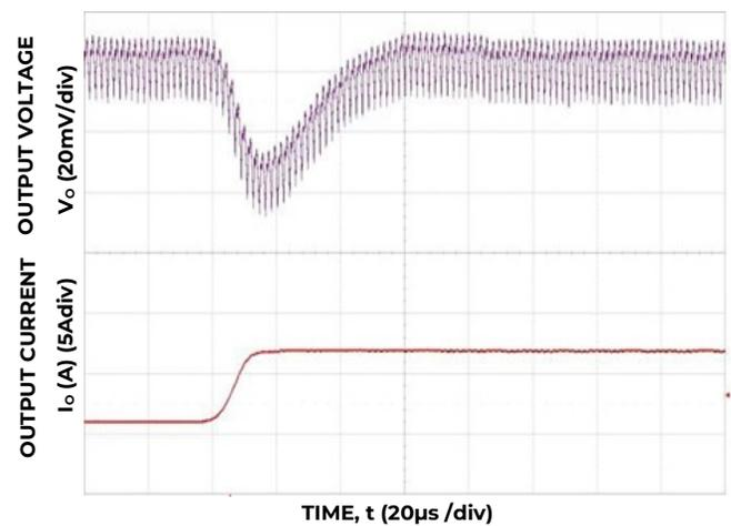
Figure 16. Transient Response to Dynamic Load Change from 50% to 100% on one output at 12V<sub>in</sub>,  $C_{out}=3 \times 47\mu\text{F}+3 \times 330\mu\text{F}$ ,  $C_{Tune}=1800\text{pF}$  &  $R_{Tune}=300\Omega$
