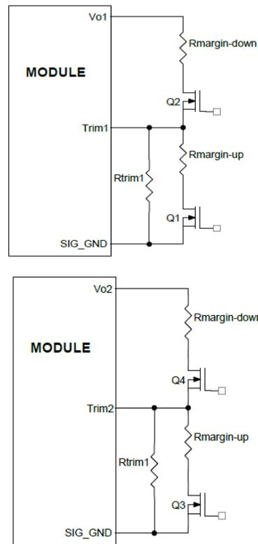
**Figure 43. Circuit Configuration for margining Output voltage.**
