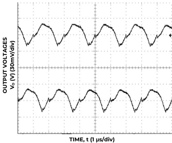
Figure 21. Typical output ripple and noise (C<sub>o</sub>= 2×0.1uF+2×47uF ceramic, V<sub>IN</sub> = 12V, I<sub>o</sub> = I<sub>o1,max</sub>, I<sub>o2,max</sub>).
