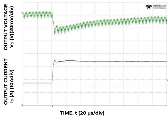
Figure 10. Transient Response to Dynamic Load Change on one output from 50% to 100% at 12V<sub>in</sub>, C<sub>out</sub> = 8x47uF + 14x330uF, C<sub>Tune</sub> = 10nF & R<sub>Tune</sub> = 300Ω
