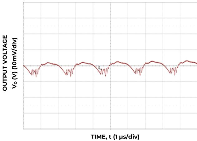
Figure 9. Typical output ripple
