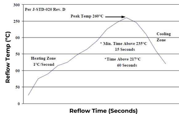
Figure 44. Recommended linear reflow profile using Sn/Ag/Cu solder.
