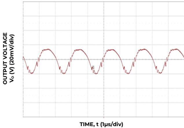
Figure 27. Typical output ripple and noise (C<sub>o</sub> = 7×22µF ceramic, V<sub>IN</sub> = 12V, I<sub>o</sub> = I<sub>o,max</sub>).
