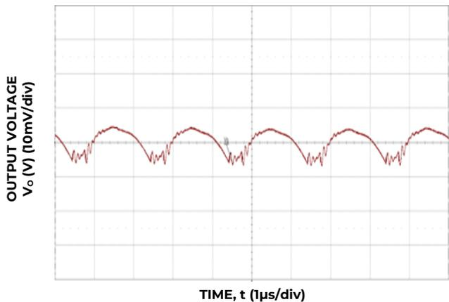
Figure 15. Typical output ripple and noise (C<sub>o</sub> = 8×47µF ceramic, V<sub>IN</sub> = 12V, I<sub>o</sub> = I<sub>o,max</sub>).
