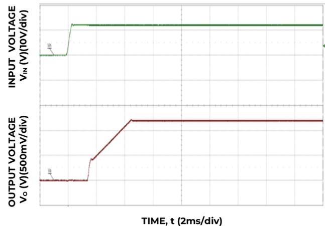
Figure 12. Typical Start-up Using Input Voltage
