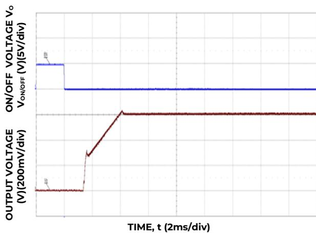
Figure 5. Typical Start-up Using On/Off Voltage (I<sub>o</sub> = I<sub>o,max</sub>).
