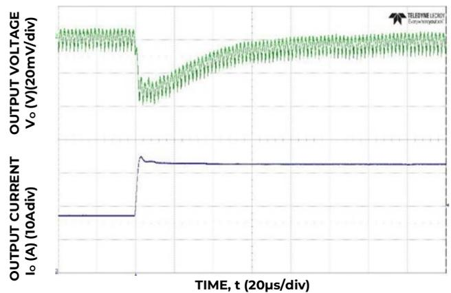
Figure 16. Transient Response to Dynamic Load Change on one output from 50% to 100% at 12V<sub>in</sub>, C<sub>out</sub> = 8×47µF + 7×330µF, C<sub>Tune</sub> = 4.7nF & R<sub>Tune</sub> = 221Ω
