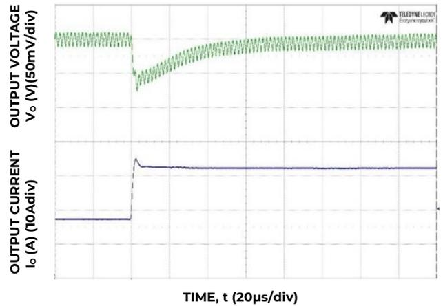
Figure 28. Transient Response to Dynamic Load Change on one output from 50% to 100% at 12V<sub>in</sub>, C<sub>out</sub> = 8x47µF + 2x330µF, C<sub>Tune</sub> = 2700pF & R<sub>Tune</sub> = 221Ω
