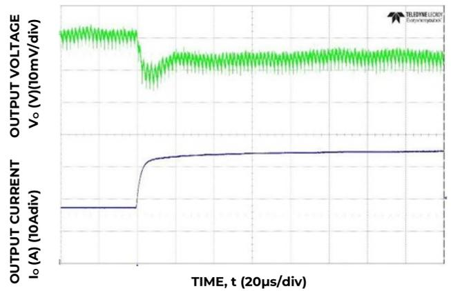
Figure 4. Transient Response to Dynamic Load Change from 50% to 100% at 12V<sub>in</sub>, C<sub>out</sub>=8x47uF+24x330uF, C<sub>Tune</sub>=18nF, R<sub>Tune</sub>=300Ω
