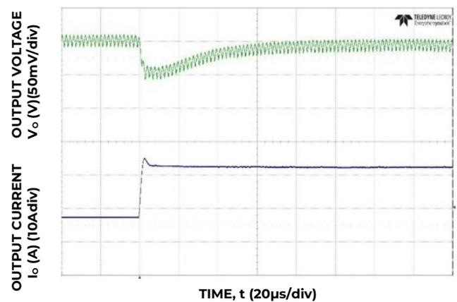
Figure 22. Transient Response to Dynamic Load Change on one output from 50% to 100% at 12V<sub>in</sub>, C<sub>out</sub> = 8×47uF + 4×330uF, C<sub>Tune</sub> = 3300pF & R<sub>Tune</sub> = 221Ω
