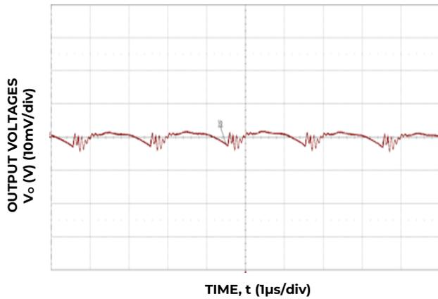
Figure 3. Typical output ripple
