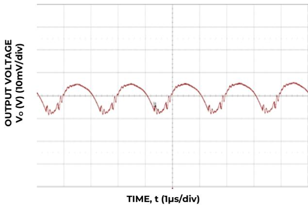
Figure 21. Typical output ripple and noise (C<sub>o</sub> = 8×47μF ceramic, V<sub>IN</sub> = 12V, I<sub>o</sub> = I<sub>o,max</sub>).
