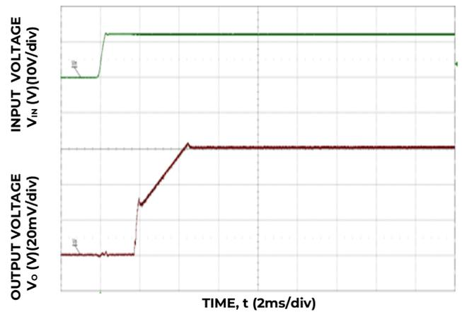
Figure 6. Typical Start-up Using Input Voltage
