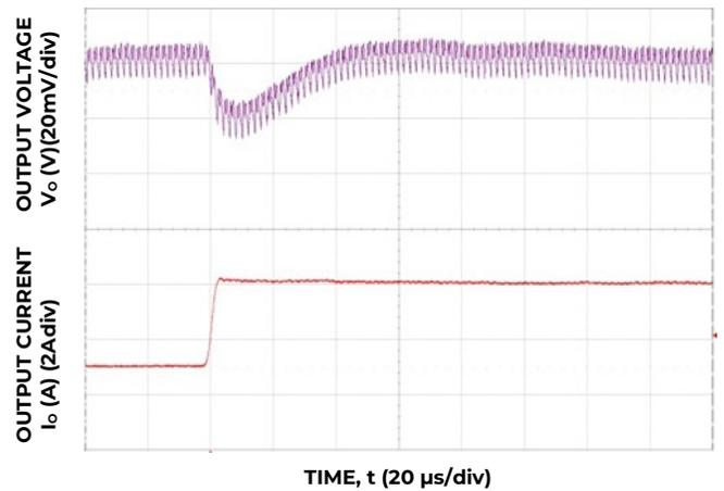
Figure 10. Transient Response to Dynamic Load Change on one output from 50% to 100% at 12V<sub>in</sub>,  $C_{out} = 3 \times 47\mu\text{F} + 2 \times 330\mu\text{F}$ ,  $C_{Tune} = 2700\text{pF}$  &  $R_{Tune} = 300\Omega$
