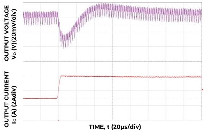
Figure 16. Transient Response to Dynamic Load Change on one output from 50% to 100% at 12V<sub>in</sub>,  $C_{out} = 3 \times 47\mu F + 2 \times 330\mu F$ ,  $C_{Tune} = 1800pF$  &  $R_{Tune} = 300\Omega$
