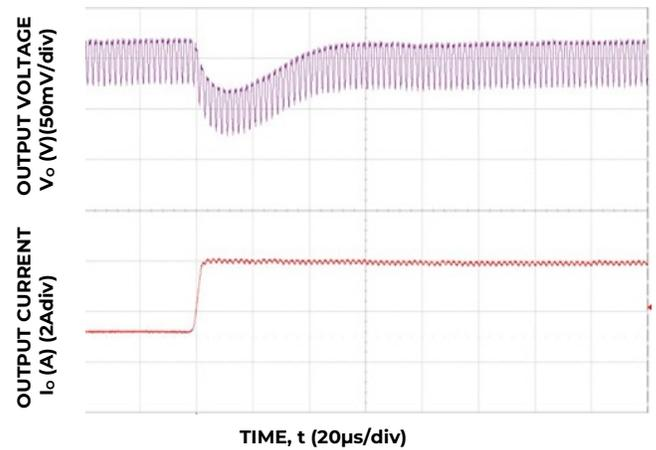
Figure 28. Transient Response to Dynamic Load Change on one output from 50% to 100% at 12V<sub>in</sub>.  $C_{out} = 2 \times 47\mu F + 1 \times 330\mu F$ ,  $C_{Tune} = 1200pF$  &  $R_{Tune} = 300\Omega$
