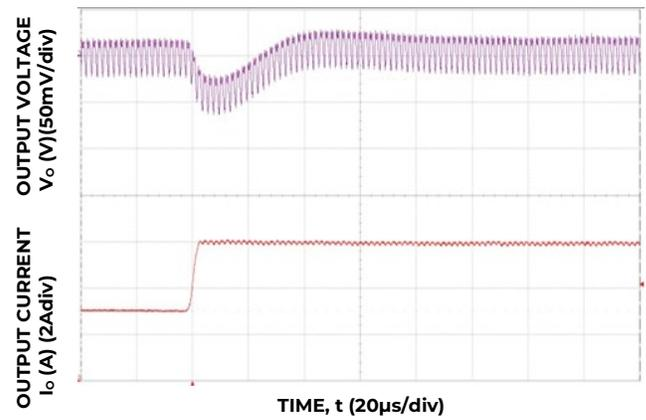
Figure 22. Transient Response to Dynamic Load Change on one output from 50% to 100% at 12V<sub>in</sub>,  $C_{out} = 2 \times 47\mu F + 1 \times 330\mu F$ ,  $C_{Tune} = 1500pF$  &  $R_{Tune} = 300\Omega$
