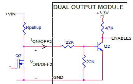
Figure 40. Circuit configuration for using negative On/Off logic.
