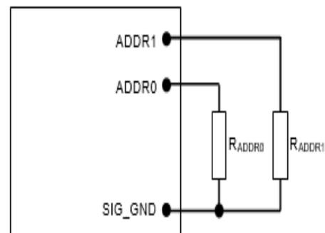
Figure 46. Circuit showing connection of resistors used to set the PMBus address of the module.
