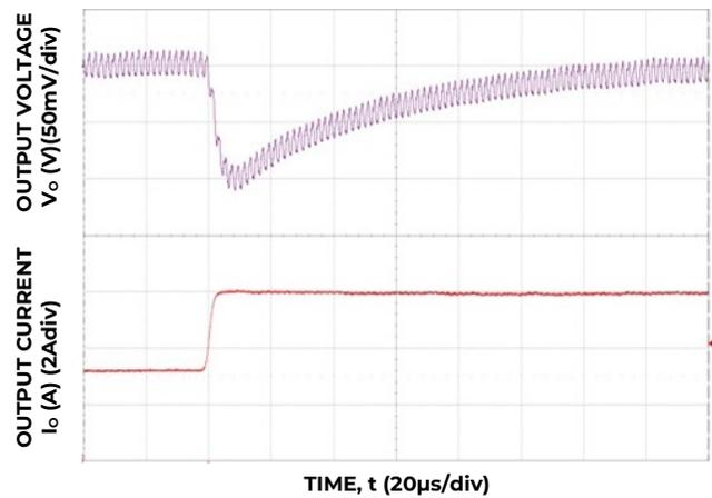
Figure 34. Transient Response to Dynamic Load Change on one output from 50% to 100% at 12V<sub>in</sub>,  $C_{out} = 4 \times 47\mu F + 1 \times 330\mu F$ ,  $C_{Tune} = 470pF$  &  $R_{Tune} = 300\Omega$
