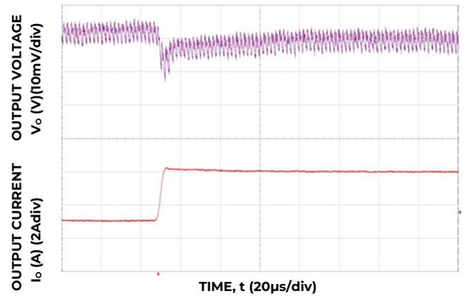
Figure 4. Transient Response to Dynamic Load Change from 50% to 100% on one output at 12V<sub>in</sub>,  $C_{out} = 3 \times 47\mu F + 3 \times 330\mu F$ ,  $C_{Tune} = 12nF$ ,  $R_{Tune} = 300\Omega$
