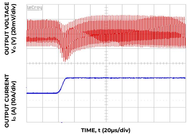
Figure 10. Transient Response to Dynamic Load Change from 50% to 100% at 12V<sub>in</sub>, C<sub>out</sub> = 1x47uF +5x330uF C<sub>Tune</sub>=10nF, R<sub>Tune</sub>=178 ohms
