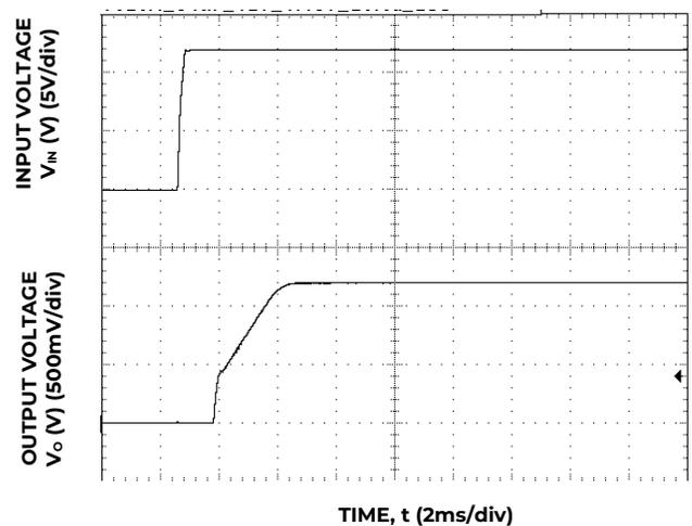
Figure 12. Typical Start-up Using Input Voltage (V<sub>IN</sub> = 12V, I<sub>o</sub> = I<sub>o,max</sub>).
