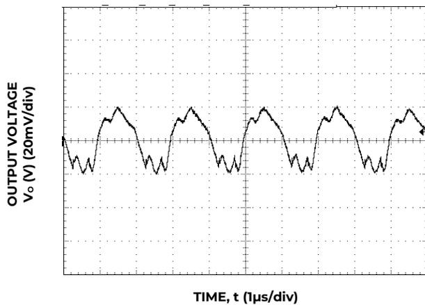
Figure 21. Typical output ripple and noise (C<sub>o</sub>=2x47µF ceramic, V<sub>IN</sub> = 12V, I<sub>o</sub> = I<sub>o,max</sub>).
