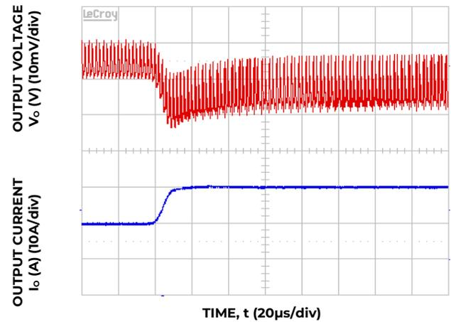
Figure 4. Transient Response to Dynamic Load Change from 50% to 100% at 12V<sub>in</sub>, C<sub>out</sub>= 1x47uF +11x330uF C<sub>Tune</sub>=47nF, R<sub>Tune</sub>=178 ohms
