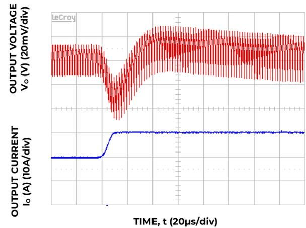
Figure 16. Transient Response to Dynamic Load Change from 50% to 100% at 12V<sub>in</sub>, C<sub>out</sub> = 2x47uF + 3x330uF C<sub>Tune</sub>=5600nF, R<sub>Tune</sub>=220 ohms
