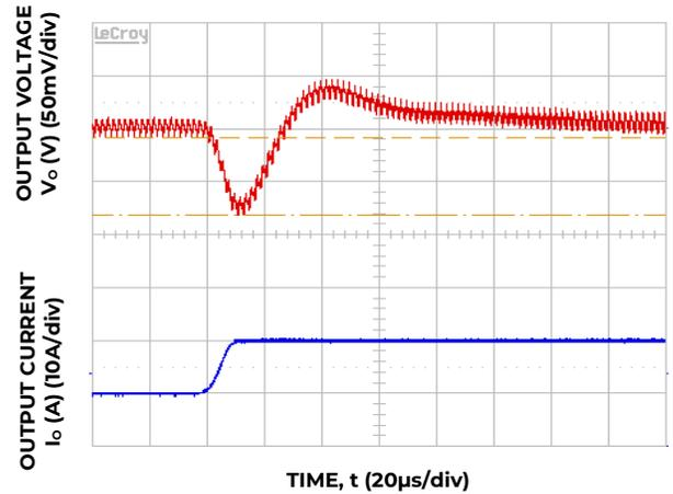
Figure 28 Transient Response to Dynamic Load Change from 50% to 100% at 12V<sub>in</sub>, C<sub>out</sub>= 5x47µF +1x330µF, C<sub>Tune</sub>=2200pF & R<sub>Tune</sub>=220 ohms
