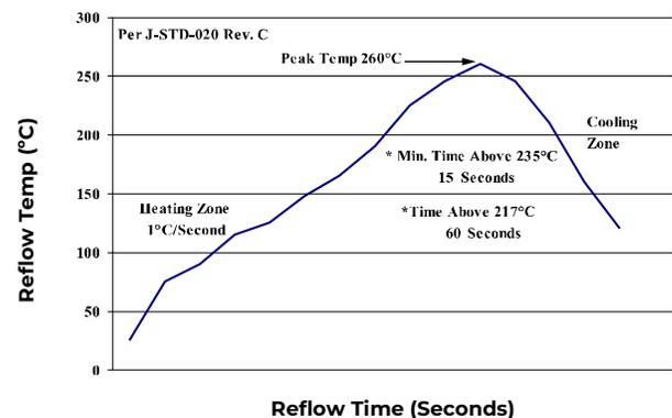
Figure 50. Recommended linear reflow profile using Sn/Ag/Cu
