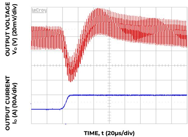
Figure 22. Transient Response to Dynamic Load Change from 50% to 100% at 12V<sub>in</sub>, C<sub>out</sub>= 2x47µF +2x330µF, C<sub>Tune</sub>=3300pF & R<sub>Tune</sub>=220 ohms
