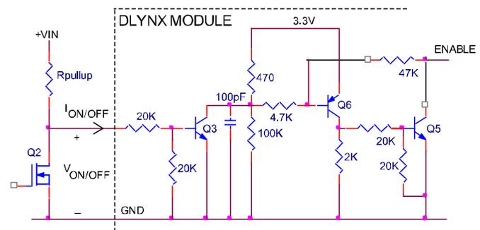
Figure 40. Circuit configuration for using negative On/Off logic.
