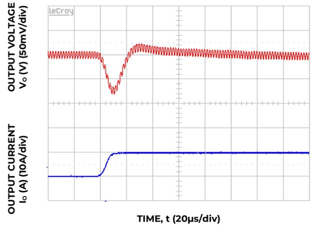
Figure 34. Transient Response to Dynamic Load Change from 50% to 100% at 12V<sub>in</sub>, C<sub>out</sub>= 8x47µF, C<sub>Tune</sub>=1500pF & R<sub>Tune</sub>=220 ohms
