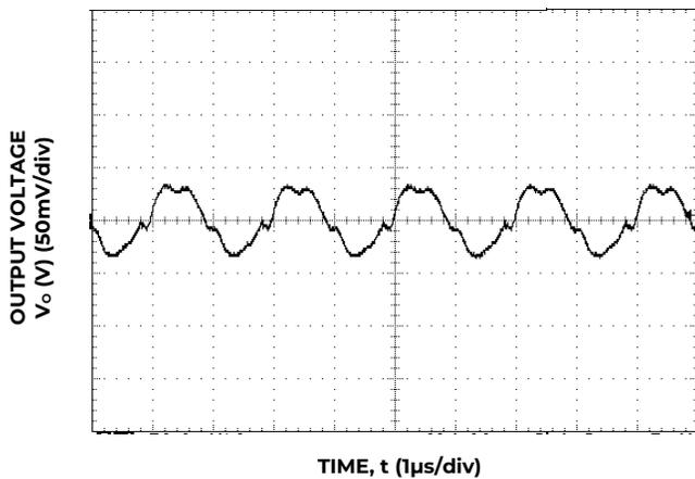
Figure 33. Typical output ripple and noise (C<sub>o</sub>=2x47µF ceramic, V<sub>IN</sub> = 12V, I<sub>o</sub> = I<sub>o,max</sub>).
