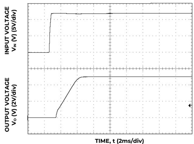
Figure 36. Typical Start-up Using Input Voltage (V<sub>IN</sub> = 12V, I<sub>o</sub> = I<sub>o,max</sub>).
