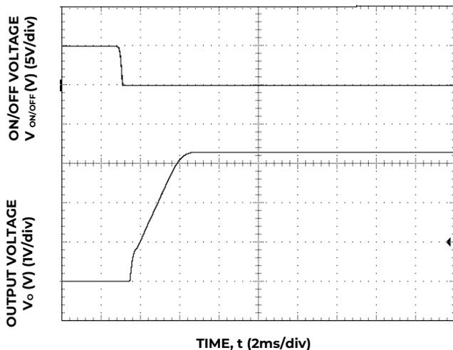
Figure 29. Typical Start-up Using On/Off Voltage (I<sub>o</sub> = I<sub>o,max</sub>).
