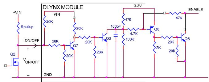
Figure 39. Circuit configuration for using positive On/Off logic.
