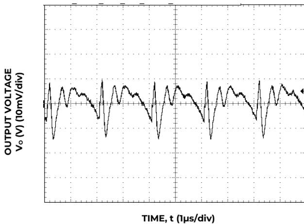
Figure 3. Typical output ripple and noise (C<sub>o</sub>=2x47µF ceramic, V<sub>IN</sub> = 12V, I<sub>o</sub> = I<sub>o,max</sub>).
