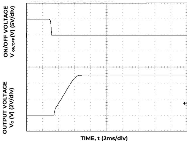
Figure 35. Typical Start-up Using On/Off Voltage (I<sub>o</sub> = I<sub>o,max</sub>).
