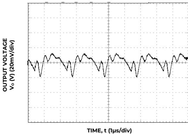
Figure 9. Typical output ripple and noise (C<sub>o</sub>=2x47µF ceramic, V<sub>IN</sub> = 12V, I<sub>o</sub> = I<sub>o,max</sub>).
