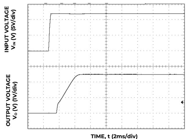
Figure 24. Typical Start-up Using Input Voltage (V<sub>IN</sub> = 12V, I<sub>o</sub> = I<sub>o,max</sub>).
