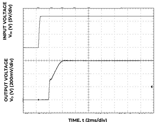
Figure 6. Typical Start-up Using Input Voltage (V<sub>IN</sub> = 12V, I<sub>o</sub> = I<sub>o,max</sub>).
