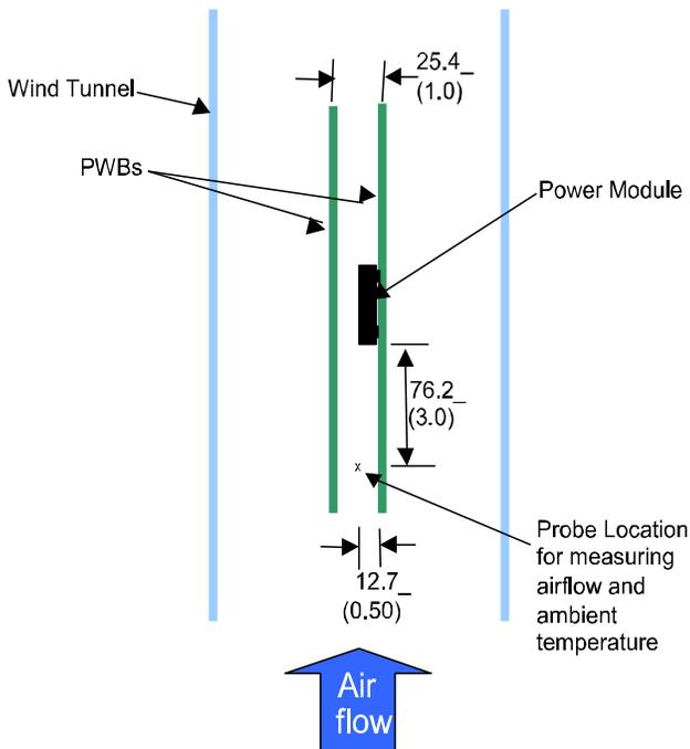
Figure 48. Thermal Test Setup.
