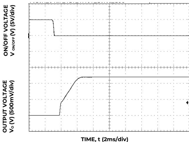
Figure 11. Typical Start-up Using On/Off Voltage (I<sub>o</sub> = I<sub>o,max</sub>).
