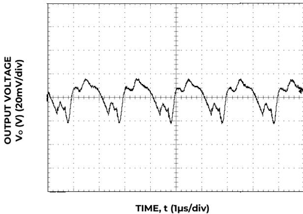
Figure 15. Typical output ripple and noise (C<sub>o</sub>=2x47μF ceramic, V<sub>IN</sub> = 12V, I<sub>o</sub> = I<sub>o,max</sub>).
