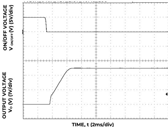
Figure 23. Typical Start-up Using On/Off Voltage (I<sub>o</sub> = I<sub>o,max</sub>).
