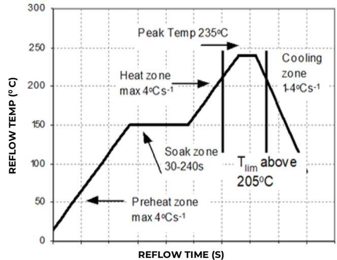
Figure 21. Recommended Reflow Profile for Sn/Pb solder.
