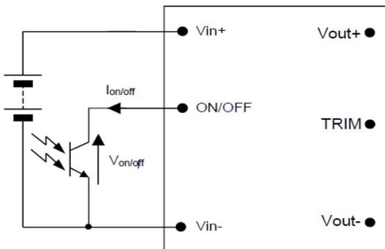
**Figure 10 Circuit configuration for using Remote On/Off Implementation.**
