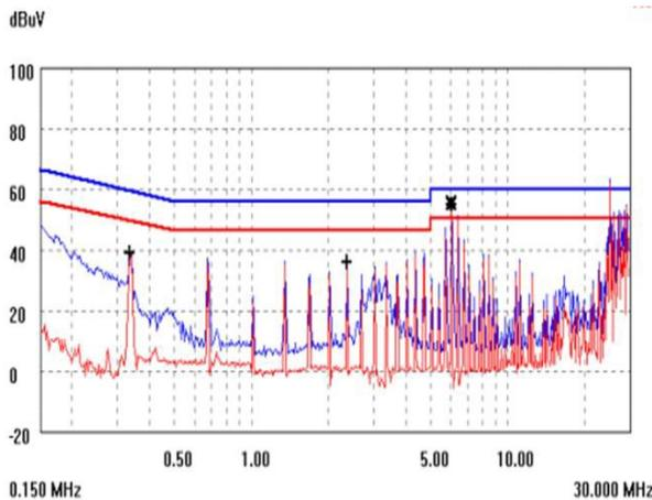
Figure 19. EMC signature using above filter, SSTWA.
