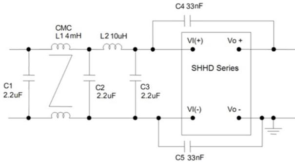
Figure 18. Suggested Configuration for EN55032 Class B.
