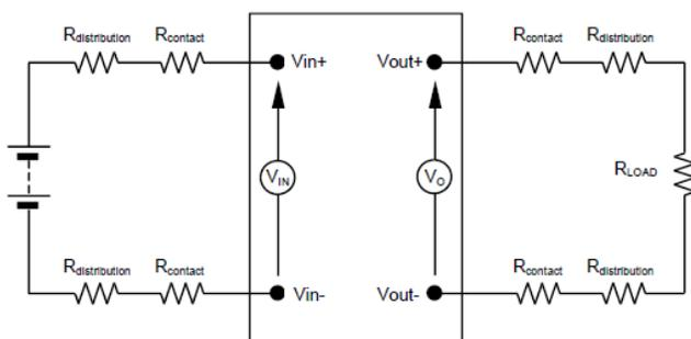
**Figure 9. Output Voltage and Efficiency Test Setup.**
