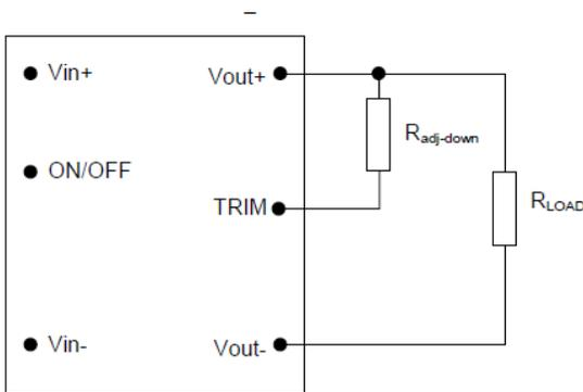
Figure 11. Circuit Configuration to Decrease Output Voltage.
