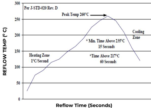
**Figure 23 Recommended linear reflow profile using Sn/Ag/Cu solder.**
