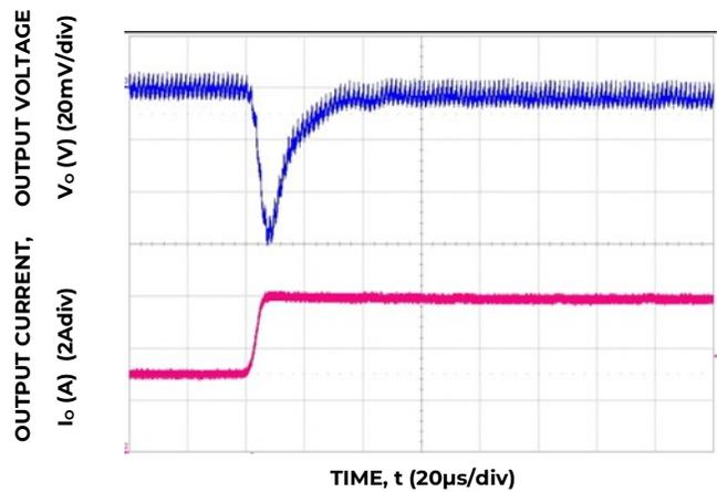
Figure 22. Transient Response to Dynamic Load Change from 50% to 100% at 12V<sub>in</sub>, C<sub>out</sub>-3x47µF, C<sub>Tune</sub>-330nF, R<sub>Tune</sub>-178
