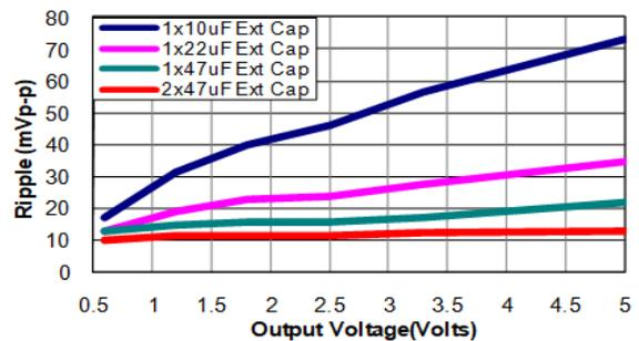
Figure 39. Output ripple voltage for various output voltages with external 1x10  $\mu\text{F}$ , 1x22  $\mu\text{F}$ , 1x47  $\mu\text{F}$  and 2x47  $\mu\text{F}$  ceramic capacitors at the output (6A load). Input voltage is 12V.
