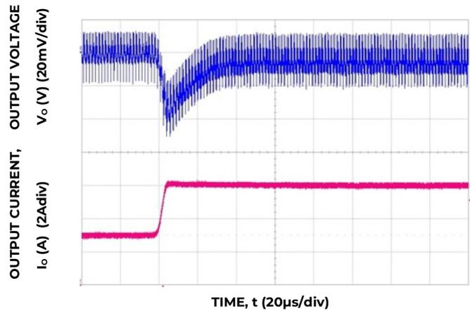
Figure 16. Transient Response to Dynamic Load Change from 50% to 100% at 12V<sub>in</sub>, C<sub>out</sub>-1x47uF+1x330uF, CT<sub>tune</sub>-4700nF, RT<sub>tune</sub>-178
