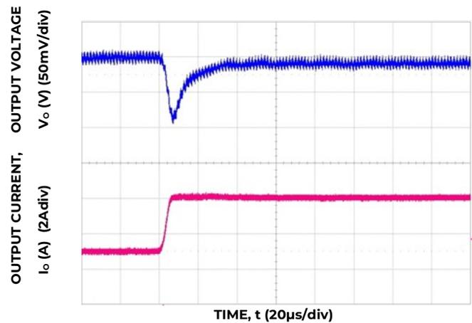
Figure 34. Transient Response to Dynamic Load Change from 50% to 100% at 12Vin, Cout-2x47uF+, CTune-2200 pF & RTune-261
