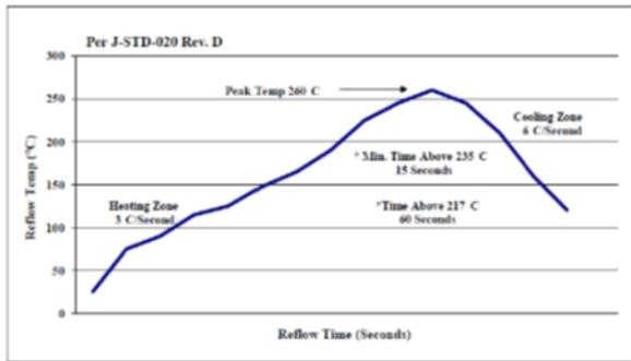
**Figure 48. Recommended linear reflow profile using Sn/Ag/Cu solder.**
