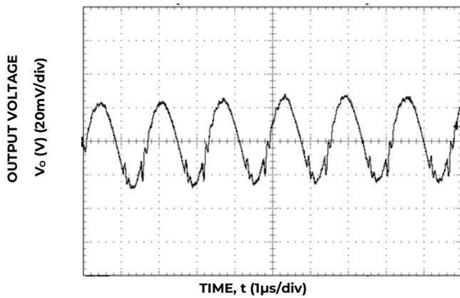
Figure 27. Typical output ripple and noise (C<sub>o</sub>=10µF ceramic, VIN = 12V, Io = Io,max, ).
