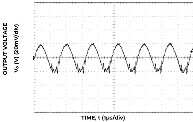
Figure 21. Typical output ripple and noise (C<sub>o</sub>=10µF ceramic, V<sub>IN</sub> = 12V, I<sub>o</sub> = I<sub>o,max</sub>.)
