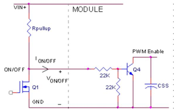
Figure 41. Circuit configuration for using negative On/Off logic.
