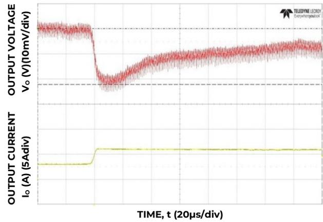
Figure 10. Transient Response to Dynamic Load Change from 50% to 100% at 12V<sub>in</sub>,  $C_{out} = 3x47\mu F + 2x330\mu F$ ,  $C_{Tune}=5600pF$ ,  $R_{Tune}=300\Omega$
