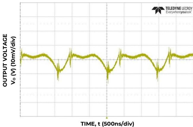
Figure 21. Typical output ripple and noise
