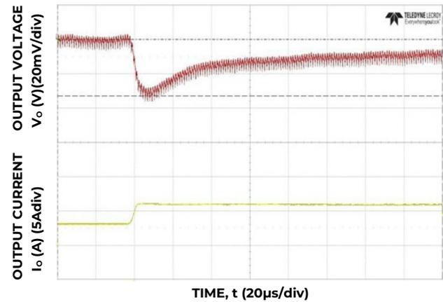
Figure 16. Transient Response to Dynamic Load Change from 50% to 100% at 12V<sub>in</sub>, C<sub>out</sub>= 3x47uF + 1x330uF, C<sub>Tune</sub>=3900pF, R<sub>Tune</sub>=300Ω
