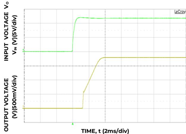
Figure 18. Typical Start-up Using Input Voltage (V<sub>IN</sub> = 12V, I<sub>o</sub> = I<sub>o,max</sub>.)
