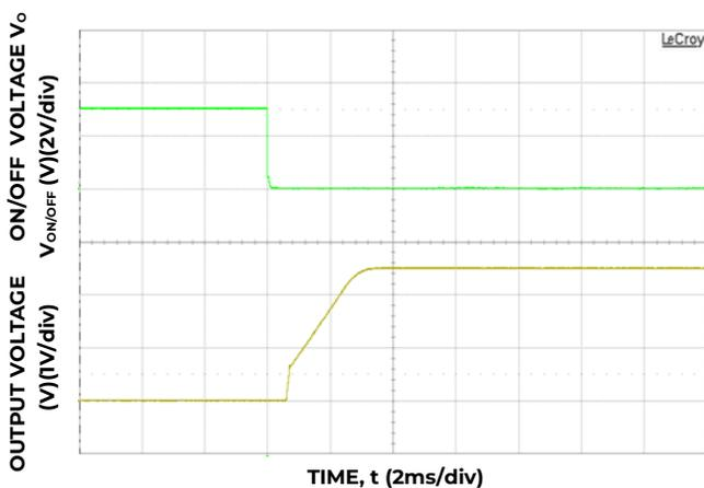
Figure 23. Typical Start-up Using On/Off Voltage
