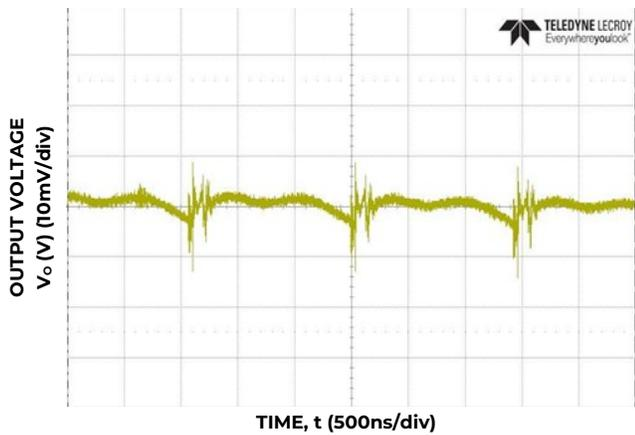
Figure 3. Typical output ripple and noise (C<sub>o</sub>=2x47μF ceramic, V<sub>IN</sub> = 12V, I<sub>o</sub> = I<sub>o,max</sub>).
