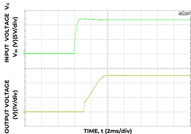
Figure 24. Typical Start-up Using Input Voltage
