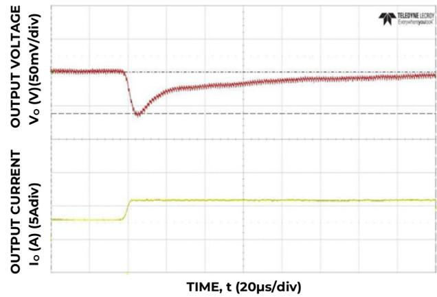
Figure 28. Transient Response to Dynamic Load Change from 50% to 100% at 12V<sub>in</sub>, C<sub>out</sub>= 5x47μF, C<sub>Tune</sub>=1800 pF, R<sub>Tune</sub>=300Ω
