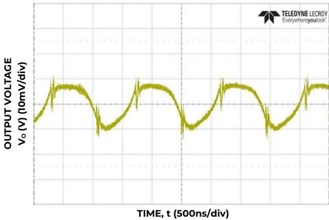
Figure 33. Typical output ripple and noise (C<sub>o</sub>=2x47μF ceramic, V<sub>IN</sub> = 12V, I<sub>o</sub> = I<sub>o,max</sub>.)
