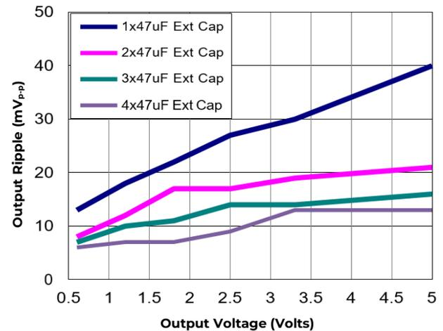
**Figure 38. Output ripple voltage for various output voltages with external 1x47 $\mu\text{F}$ , 2x47  $\mu\text{F}$ , 3x47  $\mu\text{F}$ , or 4x47  $\mu\text{F}$  ceramic capacitors at the output (6A load). Input voltage is 12V. Scope BW Limited to 20MHz**
