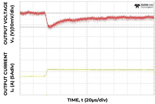
Figure 4. Transient Response to Dynamic Load Change from 50% to 100% at 12V<sub>in</sub>, C<sub>out</sub>= 3x47μF + 3x330μF, C<sub>Tune</sub>=10nF, R<sub>Tune</sub>=300Ω
