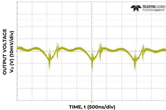
Figure 15. Typical output ripple and noise (C<sub>o</sub>=2x47μF ceramic, V<sub>IN</sub> = 12V, I<sub>o</sub> = I<sub>o,max</sub>.)
