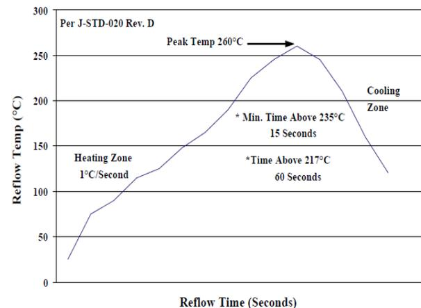
Figure 48. Recommended linear reflow profile using Sn/Ag/Cu solder.
