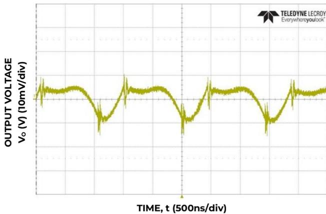
Figure 27. Typical output ripple and noise (C<sub>o</sub>=2x22μF ceramic, V<sub>IN</sub> = 12V, I<sub>o</sub> = I<sub>o,max</sub>.)
