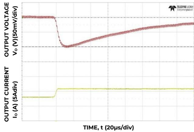
Figure 34. Transient Response to Dynamic Load Change from 50% to 100% at 12V<sub>in</sub>, C<sub>out</sub>= 5x47μF, C<sub>Tune</sub>=1800 pF, R<sub>Tune</sub>=300Ω
