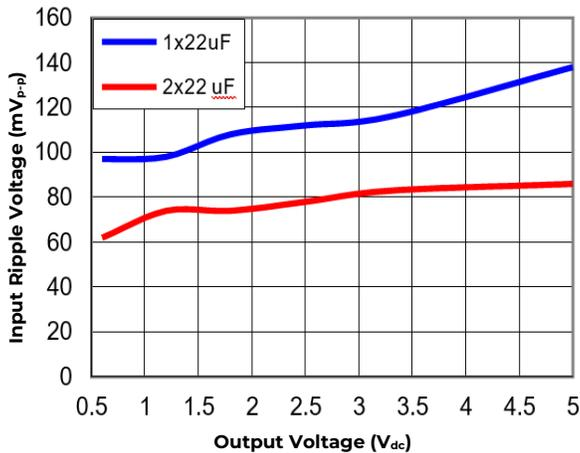
**Figure 37. Input ripple voltage for various output voltages with 1x22  $\mu\text{F}$  or 2x22  $\mu\text{F}$  ceramic capacitors at the input (6A load). Input voltage is 12V. Scope BW Limited to 20MHz**
