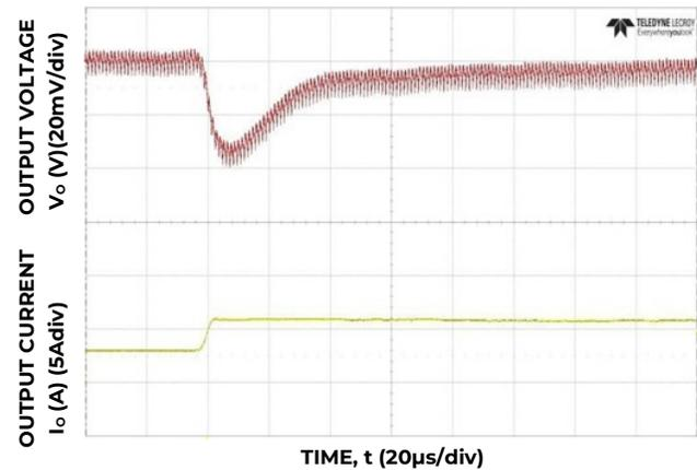
Figure 22. Transient Response to Dynamic Load Change from 50% to 100% at 12V<sub>in</sub>,
