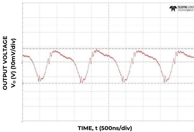
Figure 21. Typical output ripple (C<sub>o</sub>=2x47μF ceramic, V<sub>IN</sub> = 12V, I<sub>o</sub> = I<sub>o,max</sub>, 20MHz BW).
