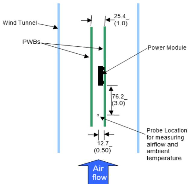
Figure 47. Thermal Test Setup.
