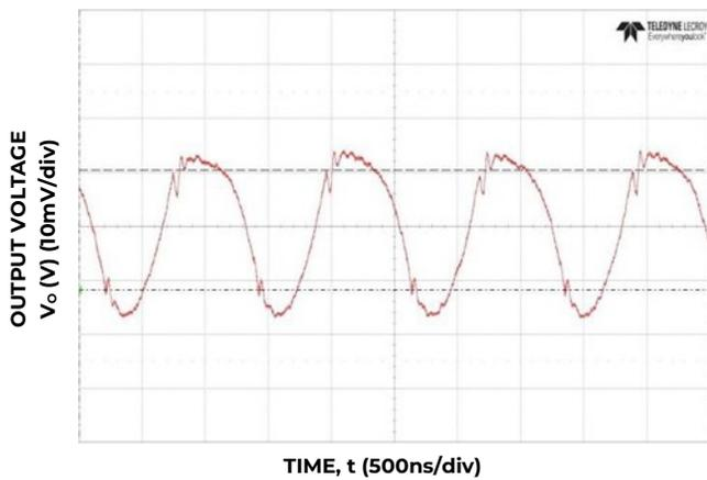
Figure 33. Typical output ripple (C<sub>o</sub>=2x47μF ceramic, V<sub>IN</sub> = 12V, I<sub>o</sub> = I<sub>o,max</sub>, 20MHz BW).
