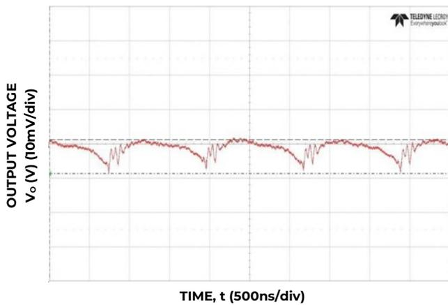
Figure 3. Typical output ripple (C<sub>o</sub>=2x47μF ceramic, V<sub>IN</sub> = 12V, I<sub>o</sub> = I<sub>o,max</sub>, 20MHz BW).
