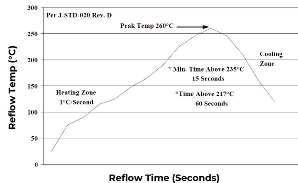
**Figure 49. Recommended linear reflow profile using Sn/Ag/Cu solder**
