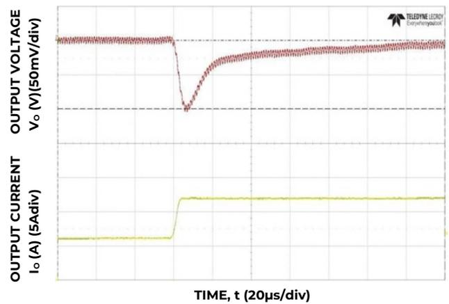
Figure 34. Transient Response to Dynamic Load Change from 50% to 100% at 12V<sub>in</sub>, C<sub>out</sub>=6x47μF, C<sub>Tune</sub>=1200pF, R<sub>Tune</sub>=300
