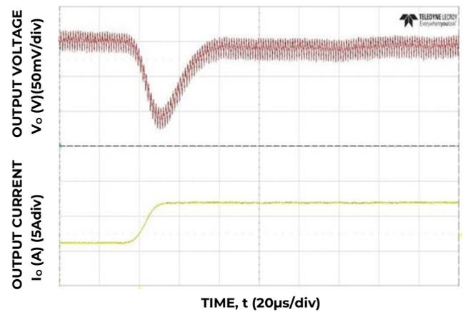
Figure 22. Transient Response to Dynamic Load Change from 50% to 100% at 12V<sub>in</sub>, C<sub>out</sub>=4x47μF+1x330μF, C<sub>Tune</sub>=2700p, R<sub>Tune</sub>=300
