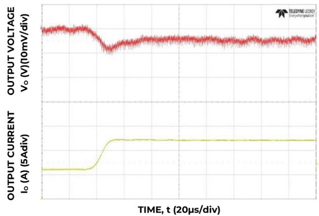
Figure 4. Transient Response to Dynamic Load Change from 50% to 100% at 12V<sub>in</sub>, C<sub>out</sub>=4x47μF+6x330μF, C<sub>Tune</sub>=47nF, R<sub>Tune</sub>=300
