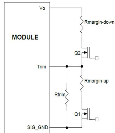
**Figure 42. Circuit Configuration for margining Output voltage.**
