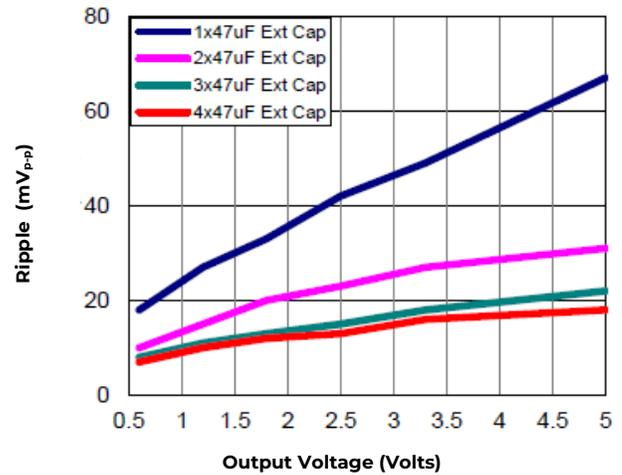
**Figure 38. Output ripple voltage for various output voltages with external 2x47  $\mu\text{F}$ , 4x47  $\mu\text{F}$ , 6x47  $\mu\text{F}$  or 8x47  $\mu\text{F}$  ceramic capacitors at the output (12A load). Input voltage is 12V.**
