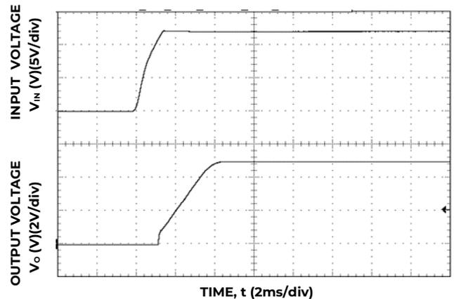
Figure 36. Typical Start-up Using Input Voltage (V<sub>IN</sub> = 12V, I<sub>o</sub> = I<sub>o,max</sub>).
