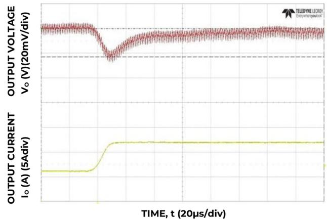
Figure 16. Transient Response to Dynamic Load Change from 50% to 100% at 12V<sub>in</sub>,  $C_{out}=4 \times 47 \mu\text{F} + 2 \times 330 \mu\text{F}$ ,  $C_{Tune}=8.2\text{nF}$ ,  $R_{Tune}=300$
