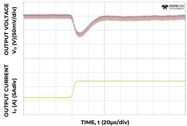
Figure 28. Transient Response to Dynamic Load Change from 50% to 100% at 12V<sub>in</sub>,  $C_{out}=3x47\mu F+1x330\mu F$ ,  $C_{Tune}=1800pF$ ,  $R_{Tune}=30\Omega$
