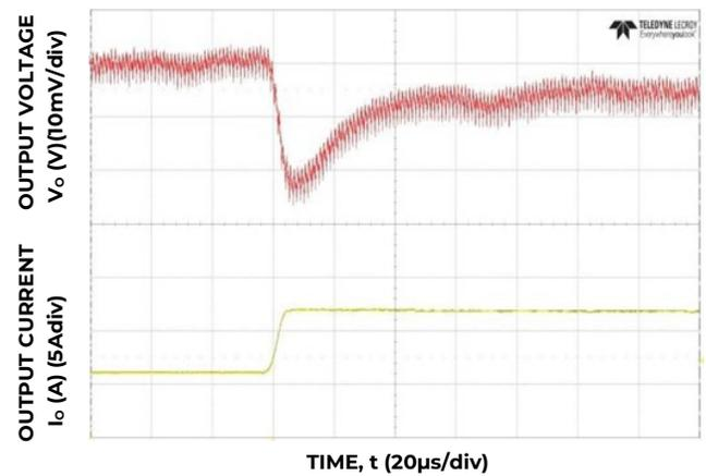
Figure 10. Transient Response to Dynamic Load Change from 50% to 100% at 12V<sub>in</sub>,  $C_{out}=4 \times 47\mu\text{F} + 3 \times 330\mu\text{F}$ ,  $C_{Tune}=10\text{nF}$ ,  $R_{Tune}=300$
