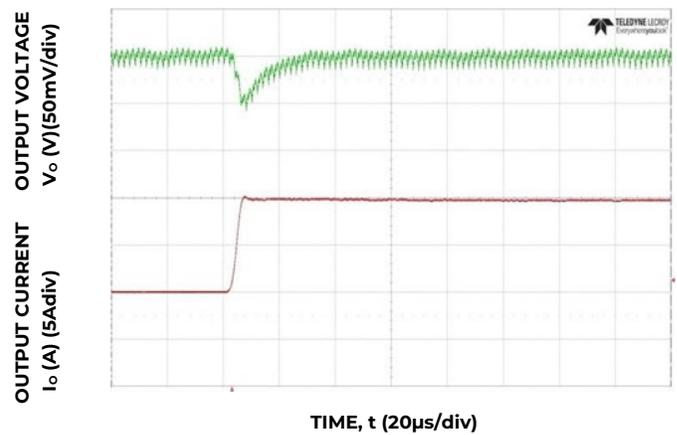
Figure 22. Transient Response to Dynamic Load Change from 50% to 100% at 12V<sub>in</sub>, C<sub>out</sub>= 7x47μF+1x330μF, C<sub>Tune</sub>=2700pF, R<sub>Tune</sub>=300
