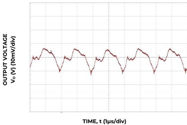
Figure 15. Typical output ripple (C<sub>O</sub>=7x22µF ceramic, V<sub>IN</sub> = 12V, I<sub>o</sub> = I<sub>o,max</sub>).
