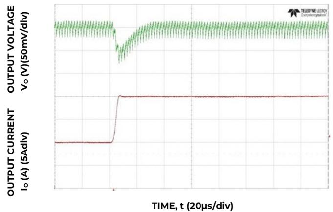
Figure 28. Transient Response to Dynamic Load Change from 50% to 100% at 12V<sub>in</sub>, C<sub>out</sub>= 4x47μF + 1x330μF, C<sub>tune</sub>=1800 pF
