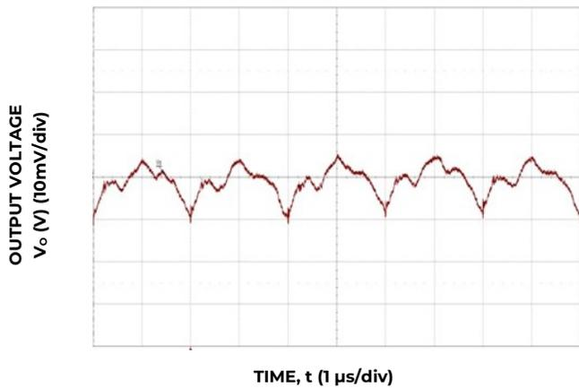
Figure 9. Typical output ripple
