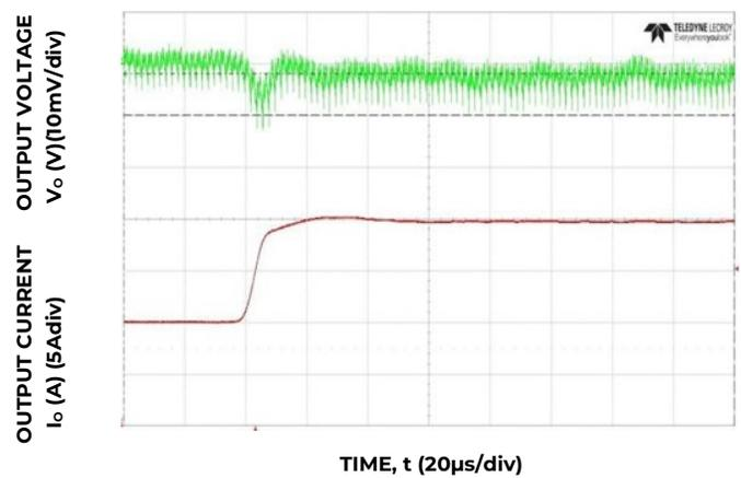
Figure 4. Transient Response to Dynamic Load Change from 50% to 100% at 12V<sub>in</sub>, C<sub>out</sub>= 7x47μF + 9x330μF, C<sub>Tune</sub>=15nF, R<sub>Tune</sub>=300
