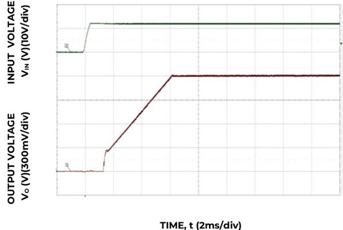
Figure 12. Typical Start-up Using Input Voltage
