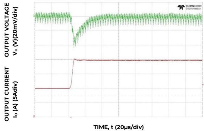
Figure 16. Transient Response to Dynamic Load Change from 50% to 100% at 12V<sub>in</sub>, C<sub>out</sub>= 7x47µF + 2x330µF, C<sub>Tune</sub>=3900pF
