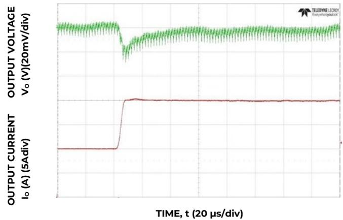
Figure 10. Transient Response to Dynamic Load Change from 50% to 100% at 12V<sub>in</sub>, C<sub>out</sub>= 7x47µF + 4x330 µF, C<sub>Tune</sub>=6800pF, R<sub>Tune</sub>=300
