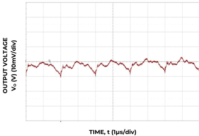
Figure 3. Typical output ripple (C<sub>O</sub>=7x22μF ceramic, V<sub>IN</sub> = 12V, I<sub>o</sub> = I<sub>o,max</sub>).
