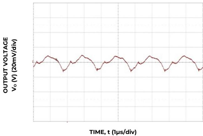
Figure 21. Typical output ripple and noise (C<sub>o</sub>=7x22μF ceramic, V<sub>IN</sub> = 12V, I<sub>o</sub> = I<sub>o,max</sub>.)
