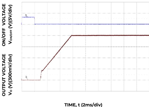
Figure 11. Typical Start-up Using On/Off Voltage
