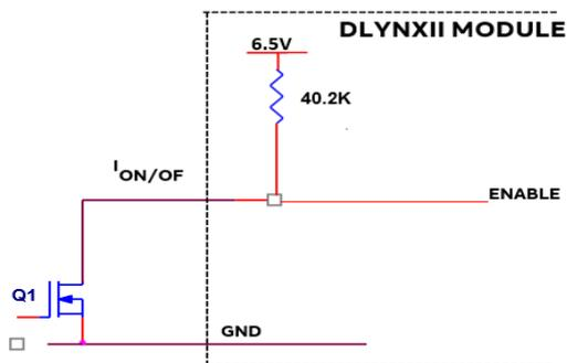
Figure 33. Circuit configuration for using positive On/Off logic.
