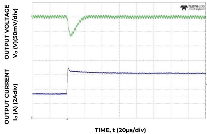
Figure 28. Transient Response to Dynamic Load Change from 50% to 100% at 12V<sub>in</sub>, C<sub>out</sub>= 5x47µF, C<sub>Tune</sub>=1.8 nF, R<sub>Tune</sub>=300Ω
