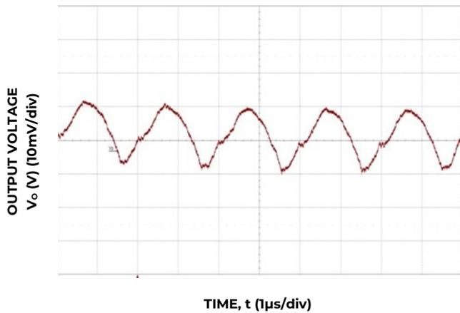
Figure 21. Typical output ripple and noise (C<sub>o</sub>=3x22µF ceramic, V<sub>IN</sub> = 12V, I<sub>o</sub> = I<sub>o,max</sub>.)
