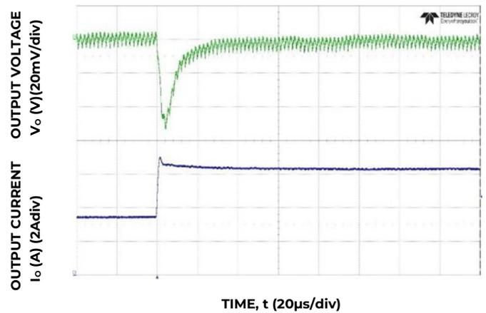
Figure 22. Transient Response to Dynamic Load Change from 50% to 100% at 12V<sub>in</sub>, C<sub>out</sub>= 6x47µF, C<sub>Tune</sub>=3.9nF, R<sub>Tune</sub>=300Ω
