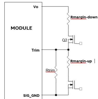
**Figure 43. Circuit Configuration for margining Output voltage.**
