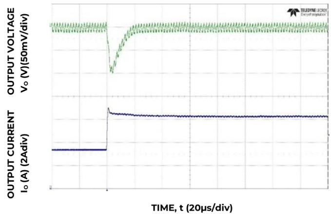
Figure 34. Transient Response to Dynamic Load Change from 50% to 100% at 12V<sub>in</sub>, C<sub>out</sub>= 3x47uF, CTune=1.8 nF, RTune=300Ω
