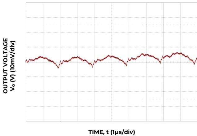
Figure 3. Typical output ripple (C<sub>o</sub>=3-x22µF ceramic, V<sub>IN</sub> = 12V, I<sub>o</sub> = I<sub>o,max</sub>).
