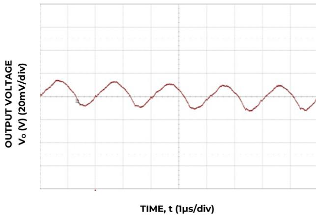
Figure 27. Typical output ripple and noise (C<sub>o</sub>=3x22µF ceramic, V<sub>IN</sub> = 12V, I<sub>o</sub> = I<sub>o,max</sub>).
