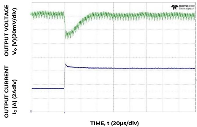
Figure 16. Transient Response to Dynamic Load Change from 50% to 100% at 12V<sub>in</sub>,  $C_{out} = 3x47\mu F + 1x330\mu F$ ,  $C_{Tune}=3.9nF$ ,  $R_{Tune}=300\Omega$
