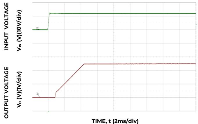
Figure 24. Typical Start-up Using Input Voltage (V<sub>IN</sub> = 12V, I<sub>o</sub> = I<sub>o,max</sub>.)
