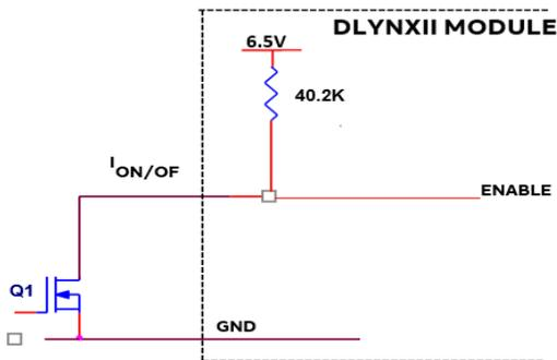
Figure 39. Circuit configuration for using positive On/Off logic.
