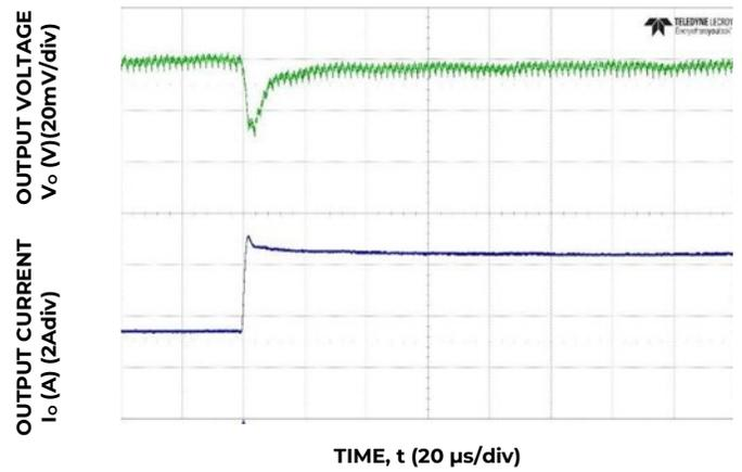
Figure 10. Transient Response to Dynamic Load Change from 50% to 100% at 12V<sub>in</sub>, C<sub>out</sub>= 6x47μF + 1x330 μF, CTune=12 nF, RTune=300 Ω
