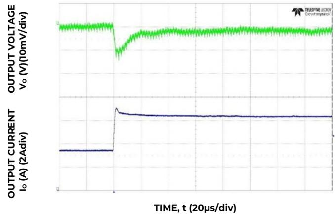
Figure 4. Transient Response to Dynamic Load Change from 50% to 100% at 12V<sub>in</sub>, C<sub>out</sub>= 6x47µF + 4x330µF, CTune=22nF, RTune=237Ω
