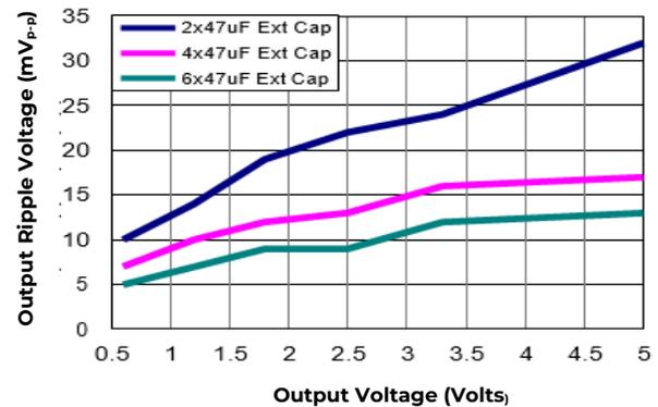
**Figure 38. Output ripple voltage for various output voltages with external 2x47  $\mu\text{F}$ , 4x47  $\mu\text{F}$  or 6x47  $\mu\text{F}$  ceramic capacitors at the output (7A load). Input voltage is 12V.**
