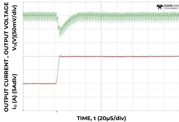
Figure 28. Transient Response to Dynamic Load Change from 50% to 100% at 12V<sub>in</sub>,  $C_{out} = 4 \times 47\mu\text{F} + 1 \times 330\mu\text{F}$   $C_{Tune} = 1800\text{pF}$ ,  $R_{Tune} = 300$
