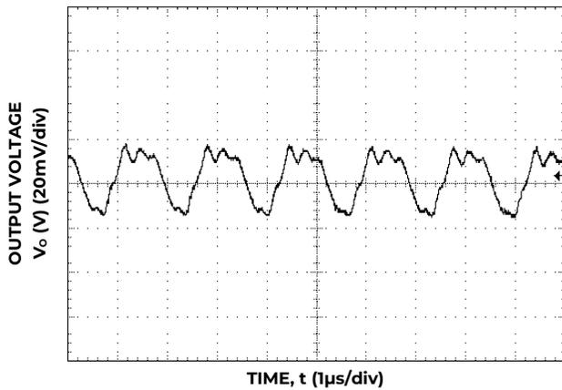
Figure 21. Typical output ripple and noise (C<sub>o</sub>=22µF ceramic, V<sub>IN</sub> = 12V, I<sub>o</sub> = I<sub>o,max</sub>).
