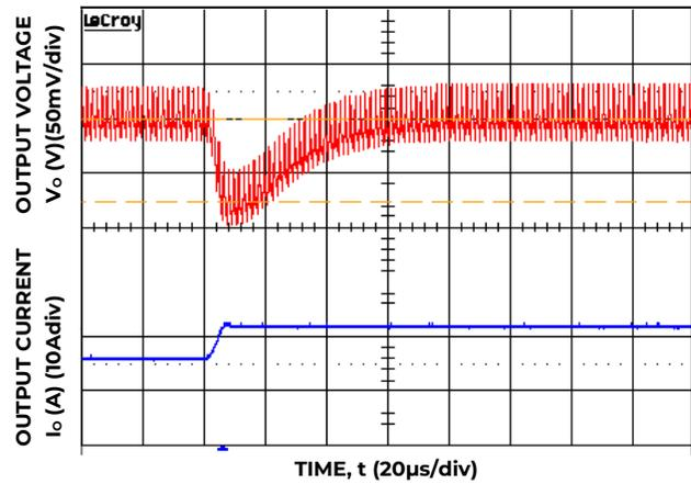
Figure 28. Transient Response to Dynamic Load Change from 50% to 100% at 12V<sub>in</sub>, C<sub>out</sub>=1x47uF+ 1x330uF, C<sub>Tune</sub>=2700pF, R<sub>Tune</sub>=330ohms
