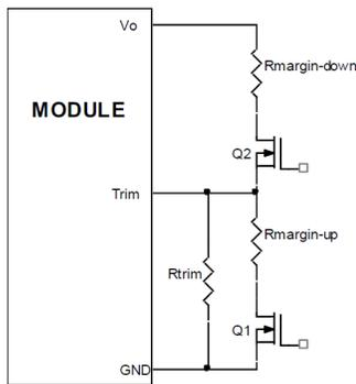
Figure 50. Circuit Configuration for margining Output voltage.
