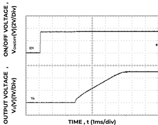
Figure 23. Typical Start-up Using On/Off Voltage (I<sub>o</sub> = I<sub>o,max</sub>).
