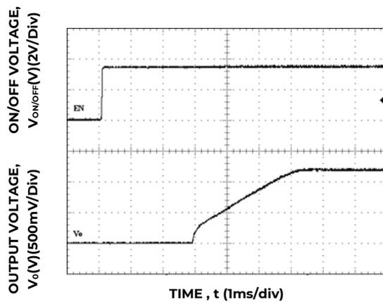
Figure 11. Typical Start-up Using On/Off Voltage (I<sub>o</sub> = I<sub>o,max</sub>).
