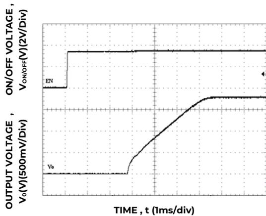
Figure 17. Typical Start-up Using On/Off Voltage (I<sub>o</sub> = I<sub>o,max</sub>).
