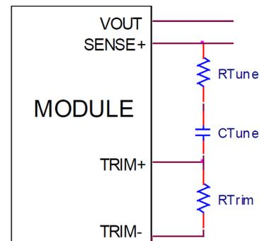
Figure 51. Circuit diagram showing connection of  $R_{TUNE}$  and  $C_{TUNE}$  to tune the control loop of the module.
