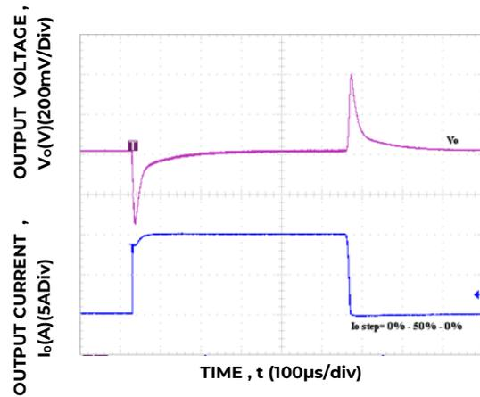
Figure 22. Transient Response to Dynamic Load Change from 0% to 50% to 0% with V<sub>IN</sub>=12V.
