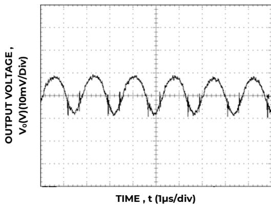
Figure 21. Typical output ripple and noise (V<sub>IN</sub> = 12V, I<sub>o</sub> = I<sub>o,max</sub>).
