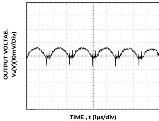
Figure 9. Typical output ripple and noise (V<sub>IN</sub> = 12V, I<sub>o</sub> = I<sub>o,max</sub>).
