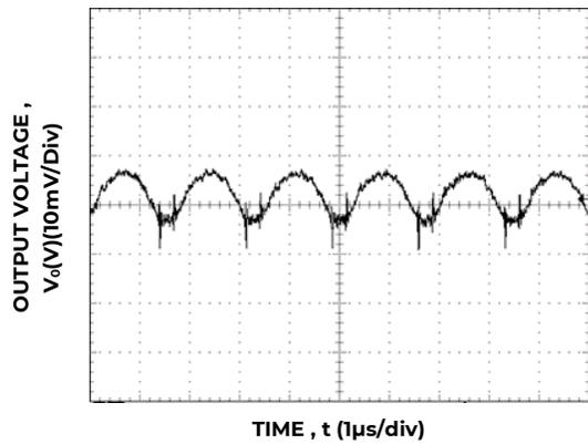
Figure 15. Typical output ripple and noise (V<sub>IN</sub> = 12V, I<sub>o</sub> = I<sub>o,max</sub>).
