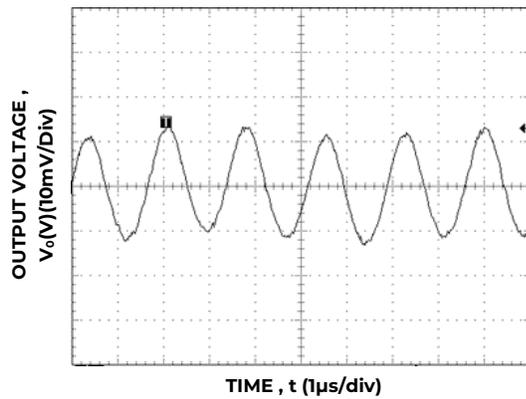
Figure 33. Typical output ripple and noise (V<sub>IN</sub> = 12V, I<sub>o</sub> = I<sub>o,max</sub>).
