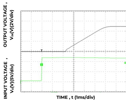
Figure 36. Typical Start-up Using Input Voltage (V<sub>IN</sub> = 12V, I<sub>o</sub> = I<sub>o,max</sub>).
