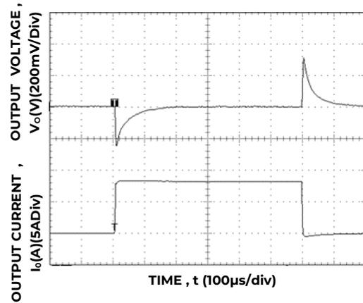
Figure 28. Transient Response to Dynamic Load Change from 0% to 50% to 0% with V<sub>IN</sub>=12V.
