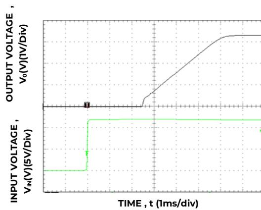
Figure 30. Typical Start-up Using Input Voltage (V<sub>IN</sub> = 12V, I<sub>o</sub> = I<sub>o,max</sub>).
