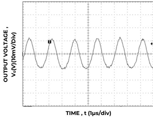
Figure 27. Typical output ripple and noise (V<sub>IN</sub> = 12V, I<sub>o</sub> = I<sub>o,max</sub>).
