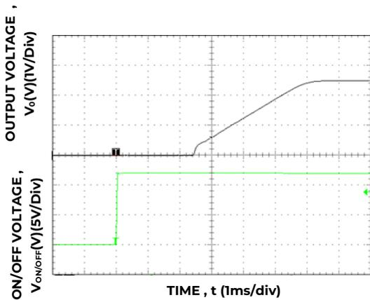
Figure 23. Typical Start-up Using On/Off Voltage ( $I_o = I_{o,max}$ ).
