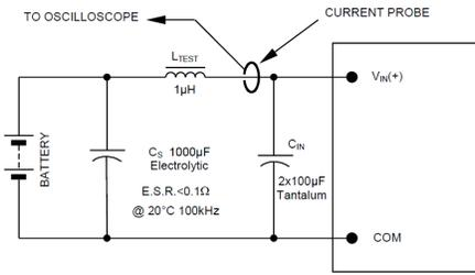
**Figure 43. Input Reflected Ripple Current Test Setup.**
