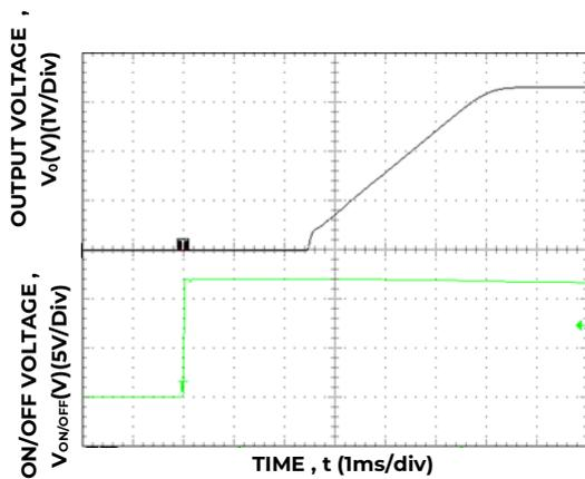
Figure 29. Typical Start-up Using On/Off Voltage (I<sub>o</sub> = I<sub>o,max</sub>).
