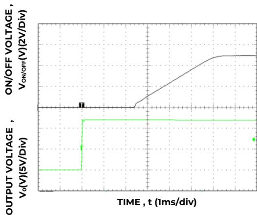
Figure 35. Typical Start-up Using On/Off Voltage (I<sub>o</sub> = I<sub>o,max</sub>).
