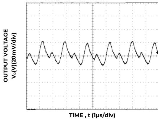
Figure 27. Typical output ripple and noise (V<sub>IN</sub> = 12V, I<sub>o</sub> = I<sub>o,max</sub>).
