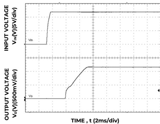
Figure 12. Typical Start-up Using Input Voltage (V<sub>IN</sub> = 9V, I<sub>o</sub> = I<sub>o,max</sub>).
