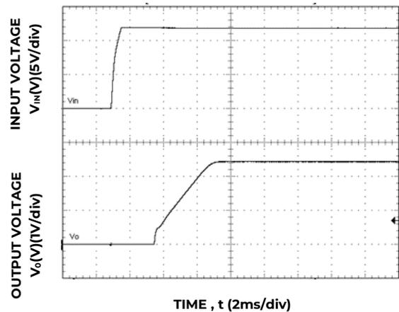
Figure 24. Typical Start-up Using Input Voltage (V<sub>IN</sub> = 12V, I<sub>o</sub> = I<sub>o,max</sub>).
