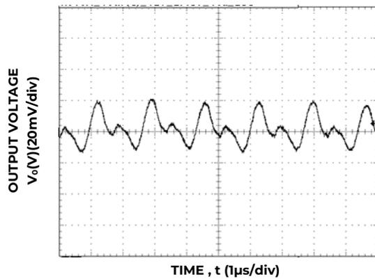
Figure 21. Typical output ripple and noise (V<sub>IN</sub> = 12V, I<sub>o</sub> = I<sub>o,max</sub>).
