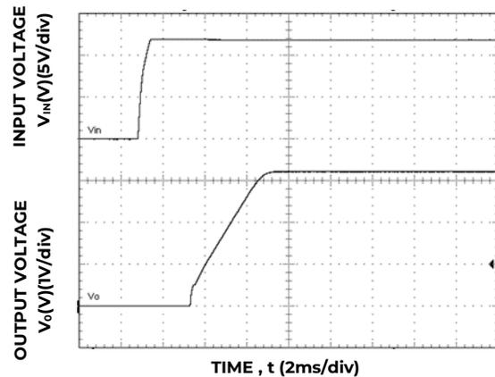
Figure 30. Typical Start-up Using Input Voltage (V<sub>IN</sub> = 12V, I<sub>o</sub> = I<sub>o,max</sub>).
