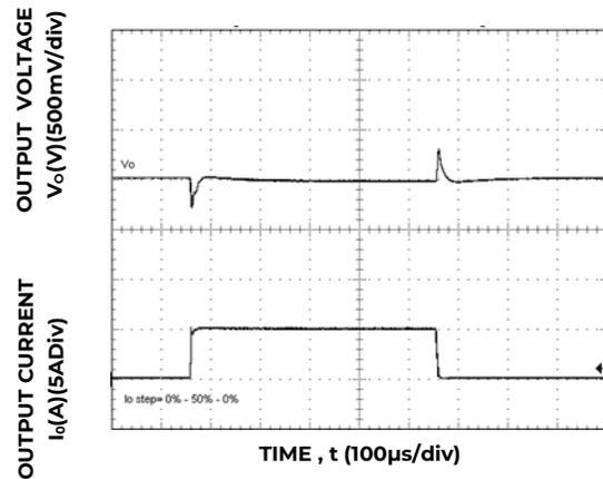
Figure 22. Transient Response to Dynamic Load Change from 0% to 50% to 0% with V<sub>IN</sub>=12V.
