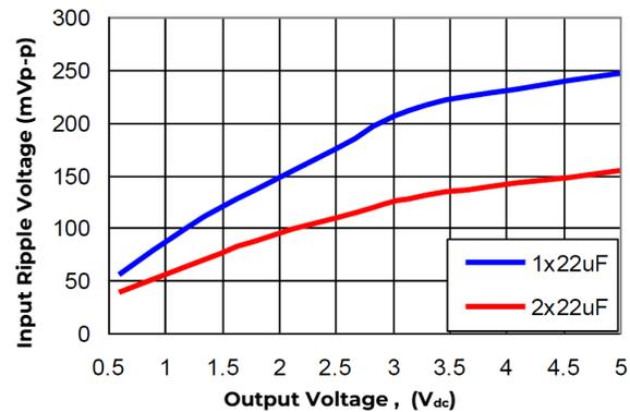
**Figure 4. Input ripple voltage for various output voltages with  $1x22\mu\text{F}$  or  $2x22\mu\text{F}$  ceramic capacitors at the input (10A load). Input voltage is 12V.**
