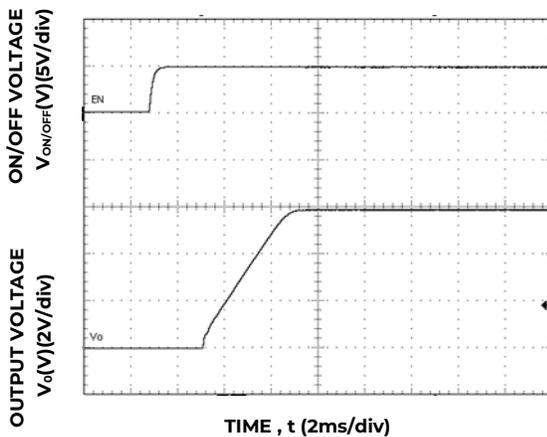
Figure 41. Typical Start-up Using On/Off Voltage ( $I_o = I_{o,max}, V_{in} = 12V$ ).
