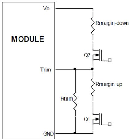
Figure 51. Circuit Configuration for margining Output voltage.
