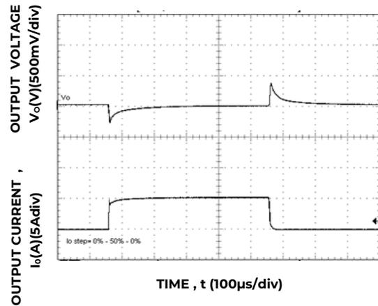
Figure 10. Transient Response to Dynamic Load Change from 0% to 50% to 0% with V<sub>IN</sub>=12V.
