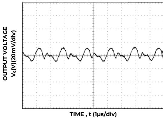
Figure 9. Typical output ripple and noise (V<sub>IN</sub> = 12V, I<sub>o</sub> = I<sub>o,max</sub>).
