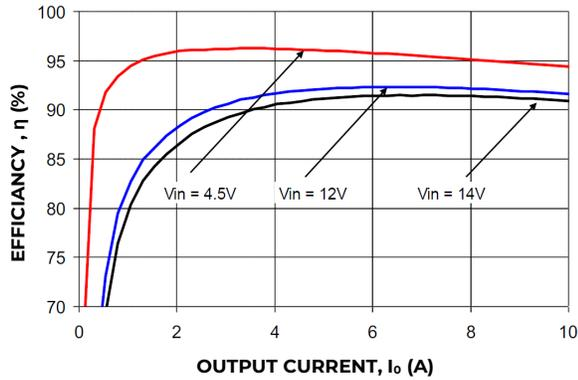
Figure 25. Converter Efficiency versus Output
