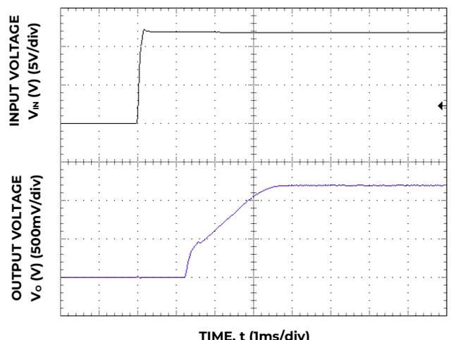
Figure 12. Typical Start-up Using Input Voltage (V<sub>IN</sub> = 12V, I<sub>o</sub> = I<sub>o,max</sub>).
