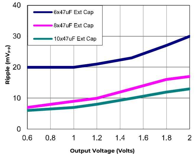
**Figure 20. Output ripple voltage for various output voltages with external 6x47 μF, 8x47 μF or 10x47 μF ceramic capacitors at the output (40A load). Input voltage is 12V. Scope Bandwidth limited to 20MHz**
