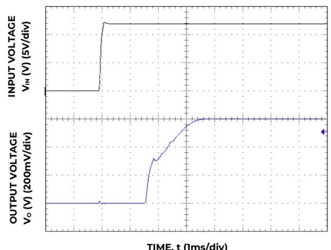
Figure 6. Typical Start-up Using Input Voltage (V<sub>IN</sub> = 12V, I<sub>o</sub> = I<sub>o,max</sub>).
