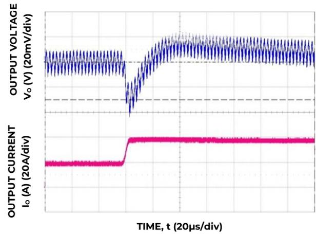
Figure 16. Transient Response to Dynamic Load Change from 50% to 100% at 12V<sub>in</sub>, C<sub>out</sub>= 6x330µF, C<sub>Tune</sub>=5.6nF & R<sub>Tune</sub>=220 ohms.
