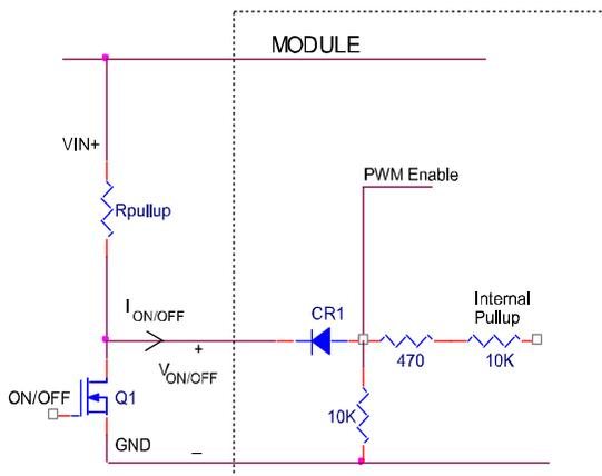
Figure 21. Circuit configuration for using positive On/Off logic.
