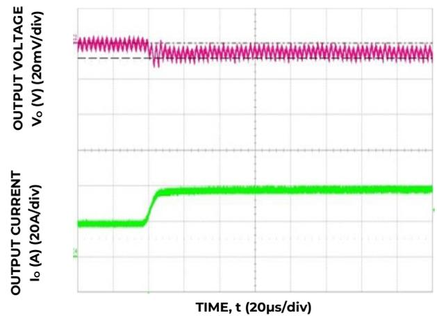
Figure 4. Transient Response to Dynamic Load Change from 50% to 100% at 12V<sub>in</sub>, C<sub>out</sub>= 12x680µF +6x47µF, C<sub>Tune</sub>=47nF, R<sub>Tune</sub>=180 ohms
