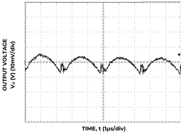
Figure 3. Typical output ripple and noise (C<sub>o</sub>=6x47 µF ceramic, V<sub>IN</sub> = 12V, I<sub>o</sub> = I<sub>o,max</sub>).
