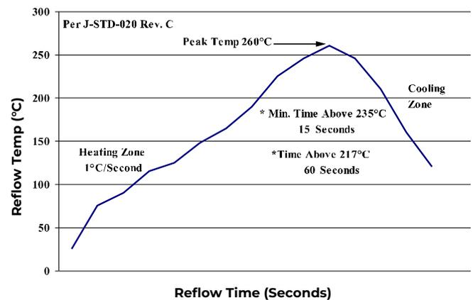
Figure 31. Recommended linear reflow profile using Sn/Ag/Cu solder.
