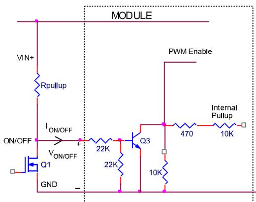
Figure 22. Circuit configuration for using negative On/Off logic.
