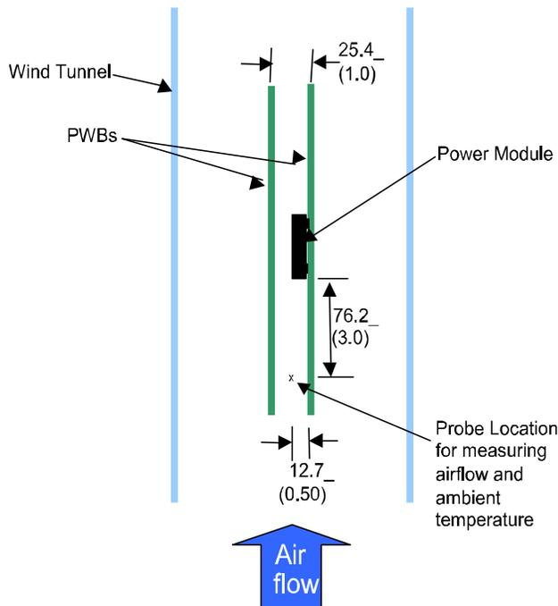
Figure 29. Thermal Test Setup.
