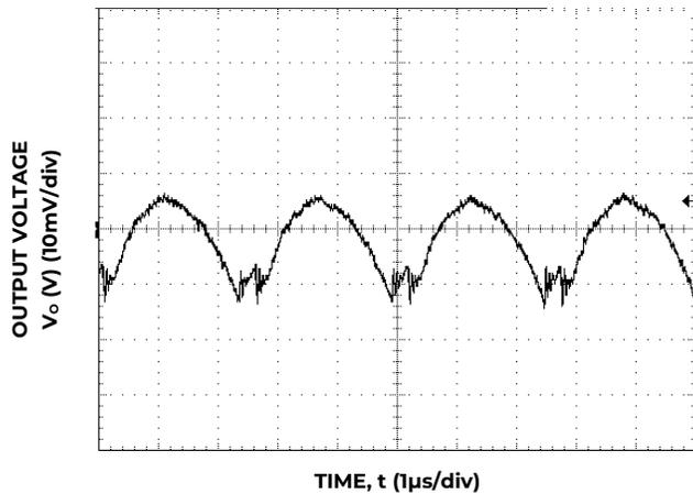
Figure 9. Typical output ripple and noise (C<sub>o</sub>=6x47µF ceramic, V<sub>IN</sub> = 12V, I<sub>o</sub> = I<sub>o,max</sub>).
