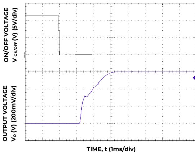
Figure 5. Typical Start-up Using On/Off Voltage (I<sub>o</sub> = I<sub>o,max</sub>).
