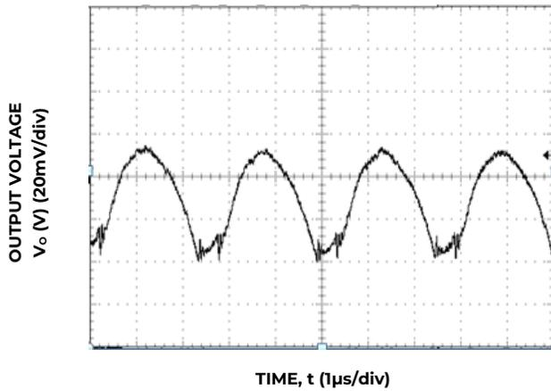
Figure 15. Typical output ripple and noise (C<sub>o</sub>=6x47µF ceramic, V<sub>IN</sub> = 12V, I<sub>o</sub> = I<sub>o,max</sub>).
