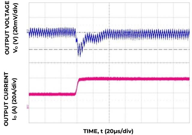
Figure 10. Transient Response to Dynamic Load Change from 50% to 100% at 12V<sub>in</sub>, C<sub>out</sub>= 6x330µF, C<sub>Tune</sub>=12nF, R<sub>Tune</sub>=200 ohms
