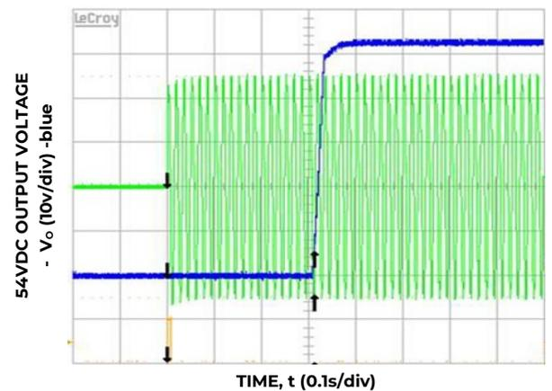
Figure 6. Start up  $V_{IN}$  176 V<sub>AC</sub>
