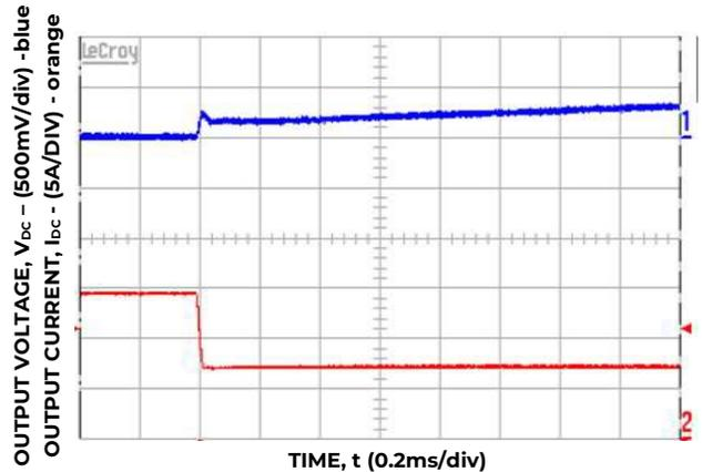
Figure 10. 54V Transient response 50% load step (100 – 50%)
