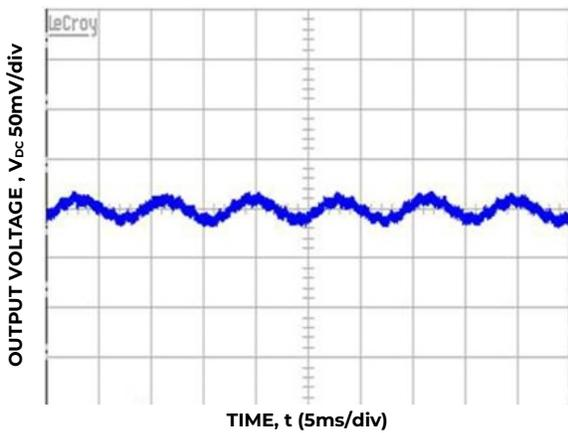
Figure 5. 54V<sub>DC</sub> output PARD, full load,  $V_{IN}$  = 230V<sub>AC</sub>
