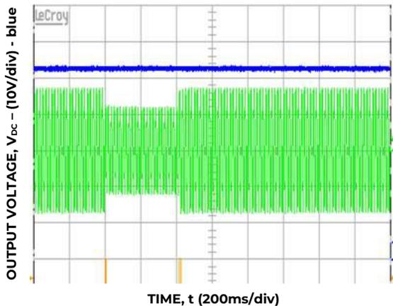
Figure 11. 30% dip ride-through  $V_{IN} 240 V_{AC}$
