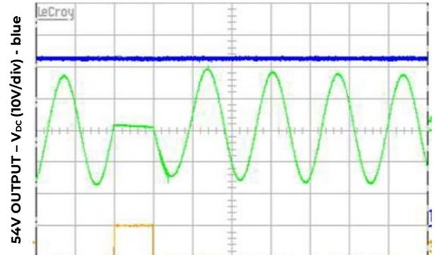
Figure 8.  $\frac{1}{2}$  cycle ride-through  $V_{IN} 240 V_{AC}$
