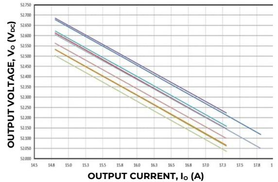
Figure 2. Output current limit profile (0° - 50°C)
