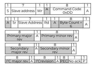
Read\_run\_timer [0xD6]: This command reads back the recorded operational ON state of the rectifier in hours. The operational ON state is accumulated from the time the rectifier is initially programmed at the factory. The rectifier is in the operational ON state both when in standby and when it delivers main output power. Recorded capacity is approximately 10 years of operational state.
