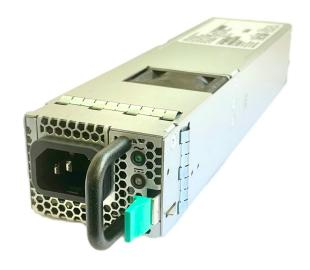
The MPR0812 series is an 850W ACDC power supply with a power density of 27.9W/in³ at a typical efficiency of 94.5% @ 50% Load. The smaller depth of 9" would be conducive for mid plane system architectures and in applications that are limited in space. MPR0812 uses the industry standard PMBus™ compliant I²C communications bus and offers a full range of control and monitoring capabilities. The SMBAlert signal pin automatically alerts customers of any state change within the power supply.
