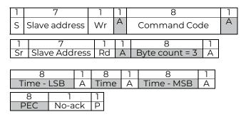
**Restart\_after\_X\_30\_sec [0xF7]:** This command is for customer use for special applications. After writing special value ( $X=1\sim9$ ), the module will turn off and then restart after X\*30 seconds. The default value is 0, which means no action of turn off and restart.
