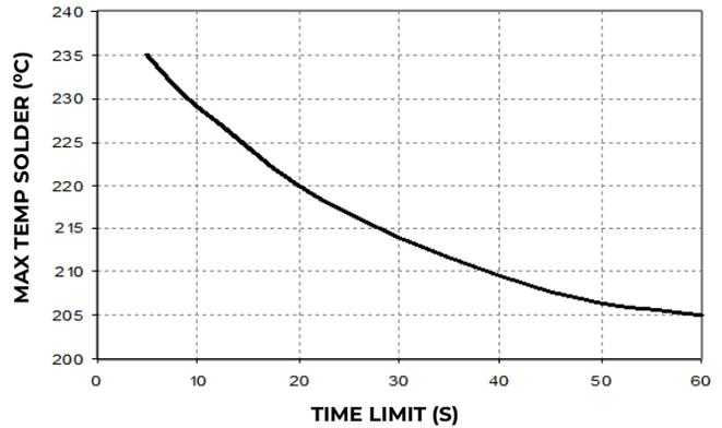
Figure 20. Time Limit, T<sub>lim</sub>, Curve Above 205°C Reflow.
