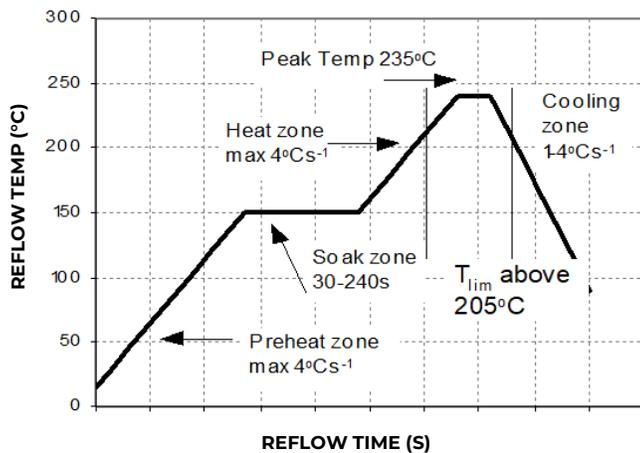
Figure 19. Recommended Reflow Profile for Sn/Pb solder.
