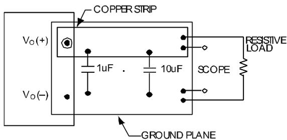
**Figure 8. Output Ripple and Noise Test Setup.**
