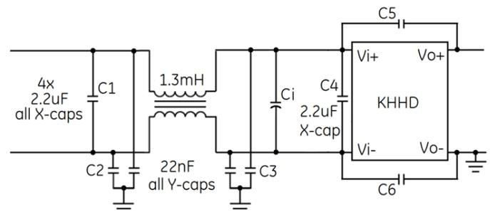
Figure 16. Suggested Configuration for EN55032 Class B.
