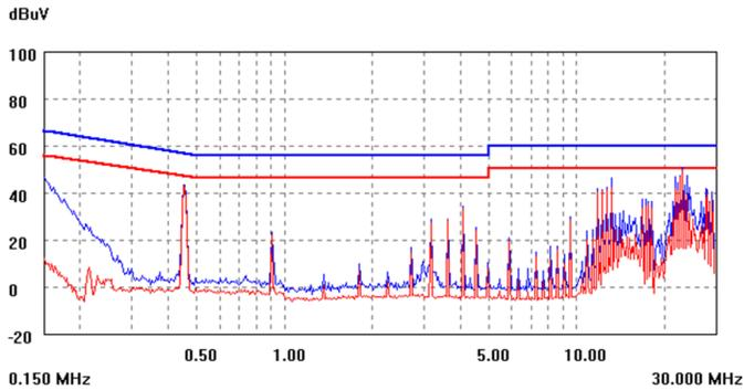
Figure 17. EMC signature using above filter, KSTW015A0F.
