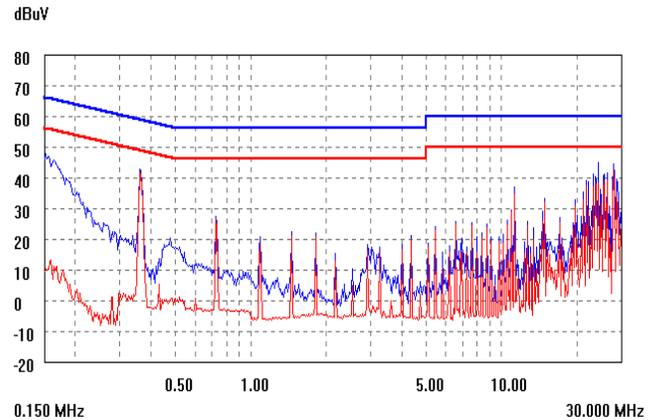
**Figure 18. EMC signature using above filter, KHHD015A0.**
