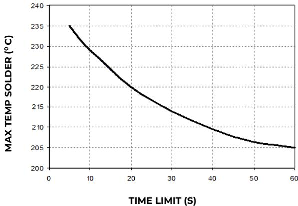
Figure 21. Time Limit, T<sub>lim</sub>, Curve Above 205°C Reflow .
