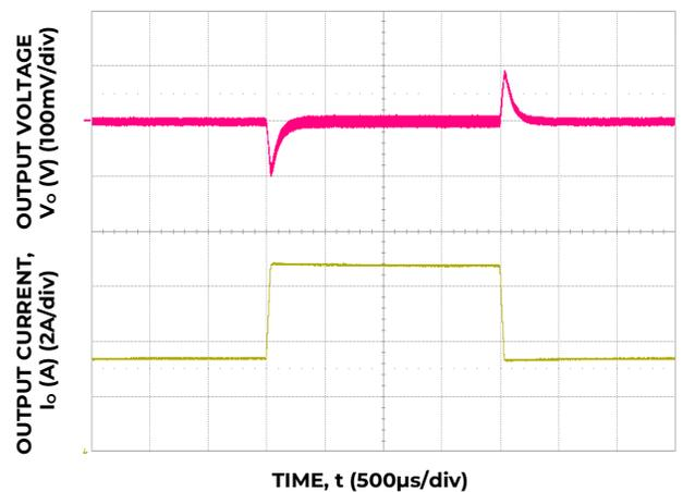
Figure 4. Transient Response to 0.1A/μS Dynamic load Change from 50% to 75% to 50% of full load,  $V_{in}=48V$
