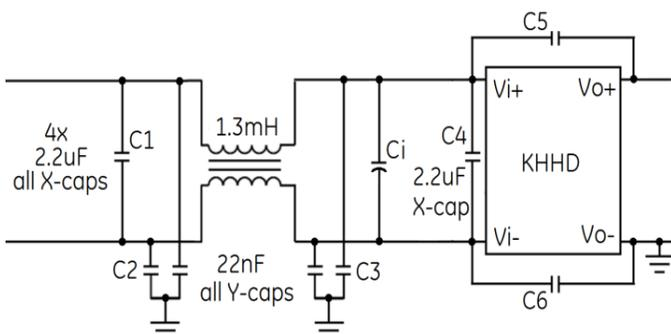
**Figure 17. Suggested Configuration for EN55032 Class B.**
