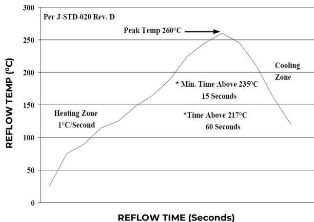
Figure 22. Recommended linear reflow profile using Sn/Ag/Cu solder
