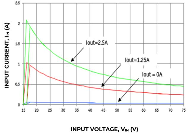
Figure 2. Converter Input Current versus Input Voltage.
