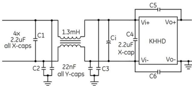
Figure 16. Suggested Configuration for EN55032 Class B.
