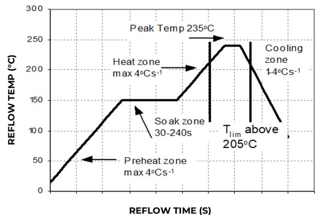
Figure 19. Recommended Reflow Profile for Sn/Pb solder.
