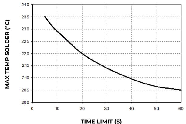
Figure 20. Time Limit,  $T_{lim}$ , Curve Above 205°C Reflow.
