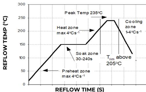
Figure 18. Reflow Profile for Tin/Lead (Sn/Pb) process.
