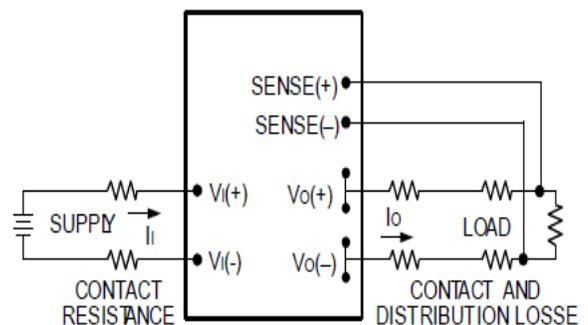
Figure 11. Circuit Configuration for remote sense .
