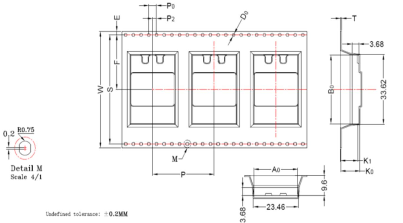
Undefined tolerance:  $\pm 0.2\text{MM}$
