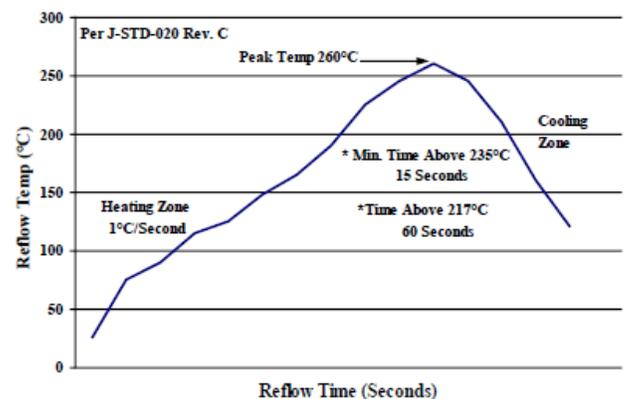
Figure 20. Recommended linear reflow profile using Sn/Ag/Cu solder.
