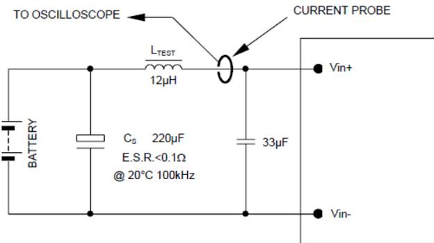
**Figure 7. Input Reflected Ripple Current Test Setup.**
