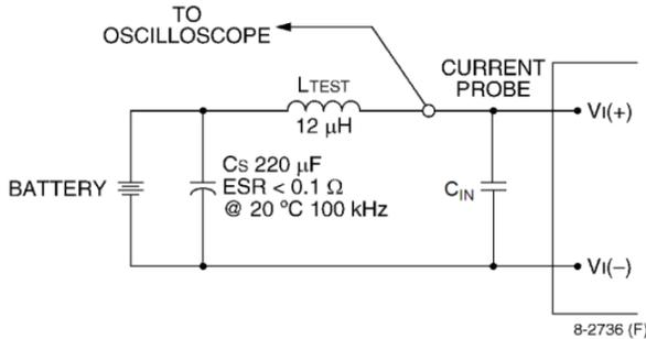
**Figure 7. Input Reflected Ripple Current Test Setup.**
