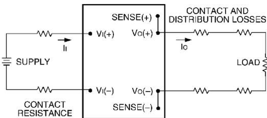
**Figure 9. Output Voltage and Efficiency Test Setup.**
