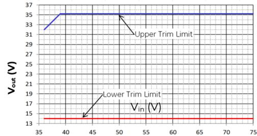
**Figure 12. Output Voltage Trim Limits vs. Input Voltage.**
