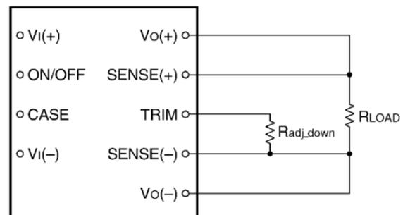
**Figure 13. Circuit Configuration to Decrease Output Voltage.**
