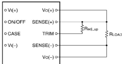
**Figure 14. Circuit Configuration to Increase Output Voltage.**
