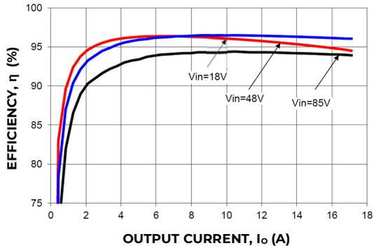
Figure 1. Converter Efficiency versus Output Current for V<sub>out</sub> = 24V.
