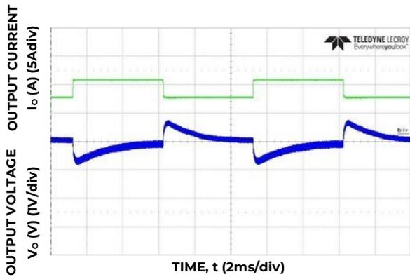
Figure 13. Transient Response to Dynamic Load Change from 50% to 100% at 48V<sub>in</sub>, C<sub>out</sub> = 330 μF electrolytic + 15 x 2.2 μF ceramic.
