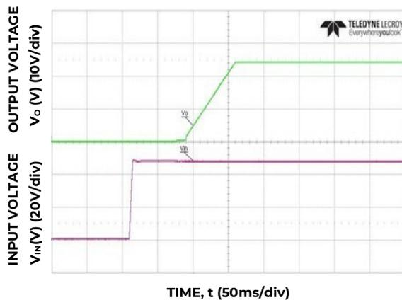
Figure 5. Typical Start-up Using Input Voltage (V<sub>IN</sub> = 48V, I<sub>o</sub> = I<sub>o,max</sub>).
