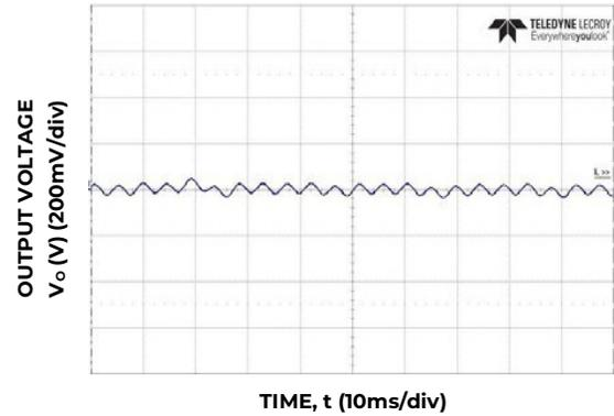
Figure 2. Typical output ripple and noise for V<sub>out</sub> = 24V. Input voltage = 48V, C<sub>out</sub> = 330 μF electrolytic + 15 x 2.2 μF ceramic.
