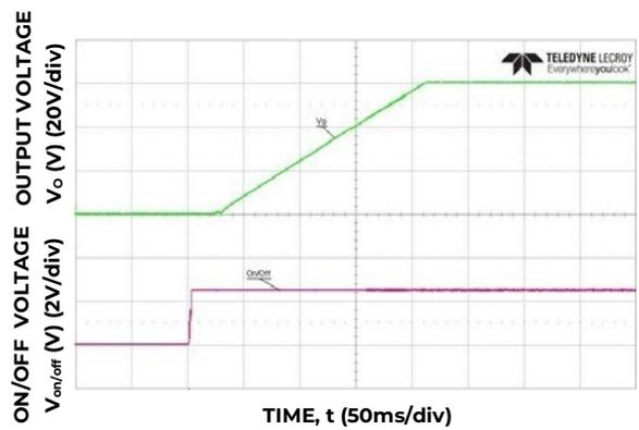
Figure 14. Typical Start-up Using On/Off Voltage (V<sub>IN</sub> = 48V, I<sub>o</sub> = I<sub>o,max</sub>).
