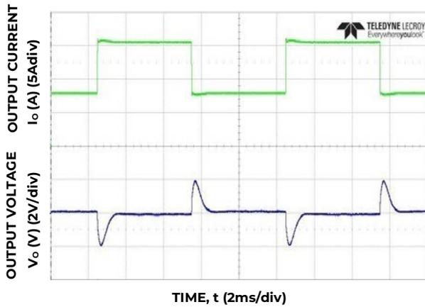
Figure 3. Transient Response to Dynamic Load Change from 50% to 100% at 48V<sub>in</sub>, C<sub>OUT</sub> = 330 μF electrolytic + 15 x 2.2 μF ceramic.
