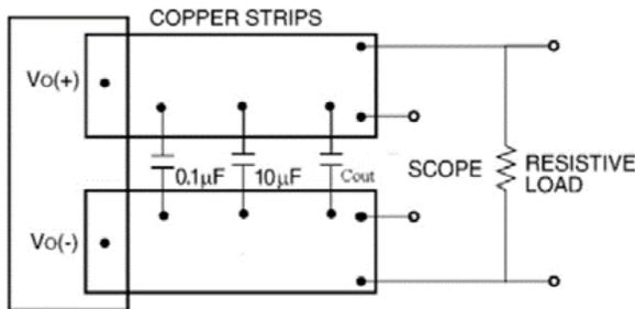
**Figure 24. Output Ripple and Noise Test Setup.**
