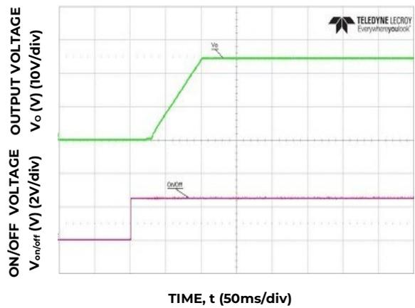
Figure 4. Typical Start-up Using On/Off Voltage (V<sub>IN</sub> = 48V, I<sub>o</sub> = I<sub>o,max</sub>).
