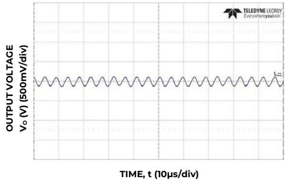
Figure 12. Typical output ripple and noise for V<sub>out</sub> = 60V. Input voltage = 48V, C<sub>OUT</sub> = 330 μF electrolytic + 15 x 2.2 μF ceramic.
