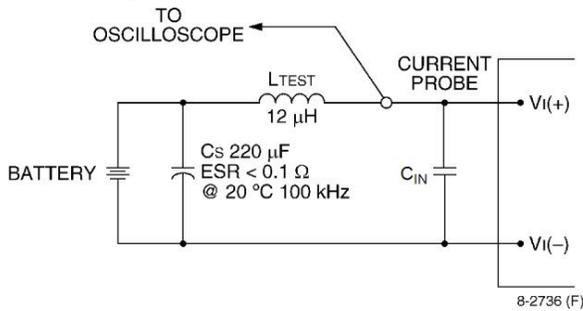
**Figure 23. Input Reflected Ripple Current Test Setup.**
