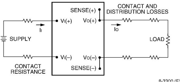
**Figure 25. Output Voltage and Efficiency Test Setup.**
