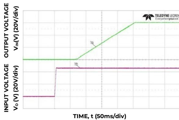
Figure 15. Typical Start-up Using Input Voltage (V<sub>IN</sub> = 48V, I<sub>o</sub> = I<sub>o,max</sub>).
