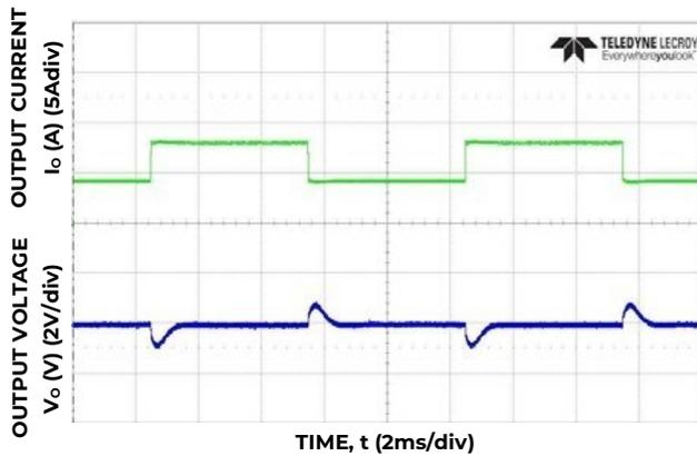
Figure 8. Transient Response to Dynamic Load Change from 50% to 100% at 74V<sub>in</sub>,  $C_{OUT} = 330 \mu F$  electrolytic + 15 x 2.2  $\mu F$  ceramic.
