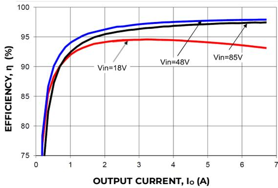
Figure 11. Converter Efficiency versus Output Current for V<sub>out</sub> = 60V.
