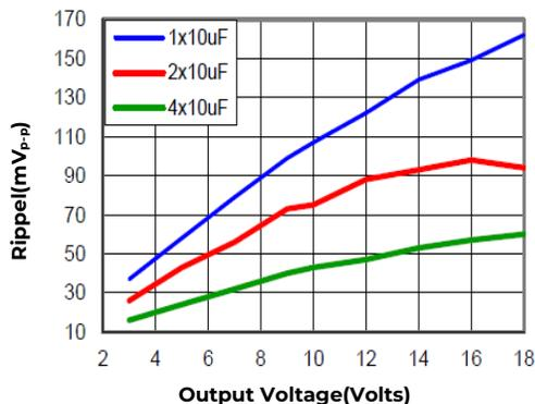
Figure 1. Output Ripple Voltage for various output voltages and external caps @28V<sub>in</sub>. Additional Decoupling cap of 0.01uF used on input and output side
