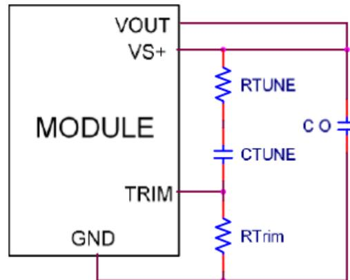
Figure. 3. Circuit diagram showing connection of R<sub>TUNE</sub> and C<sub>TUNE</sub> to tune the control loop of the module
