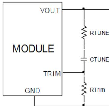
**Figure 3. Circuit diagram showing connection of R<sub>tune</sub> and C<sub>tune</sub> to tune the control loop of the module**
