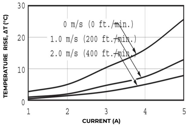
Figure 1. Typical Case Temperature Rise vs. Average Current
