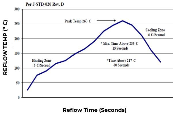
**Figure 48. Recommended linear reflow profile using Sn/Ag/Cu solder.**
