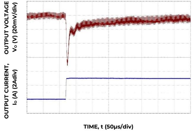
Figure 34. Transient Response to Dynamic Load Change from 50% to 100% at 12V<sub>in</sub>, C<sub>out</sub>-3x100µF, C<sub>tune</sub>-1.5nF, R<sub>tune</sub>-500
