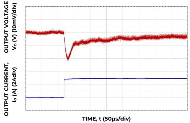
Figure 4. Transient Response to Dynamic Load Change from 5% to 100% at 12 V<sub>in</sub>, C<sub>out</sub>– 2x 330μF, 6x 100μF, C<sub>tune</sub> – 10μF, R<sub>tune</sub>– 500
