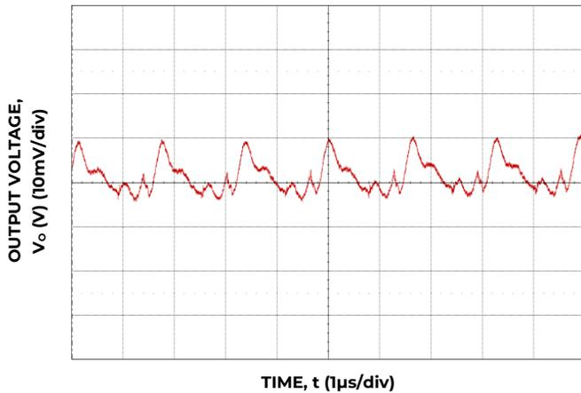
Figure 27. Typical Output Ripple and Noise, (C<sub>o</sub> = 88 μF Ceramic, V<sub>IN</sub> = 12 V, I<sub>o</sub> = I<sub>o, max</sub>.)
