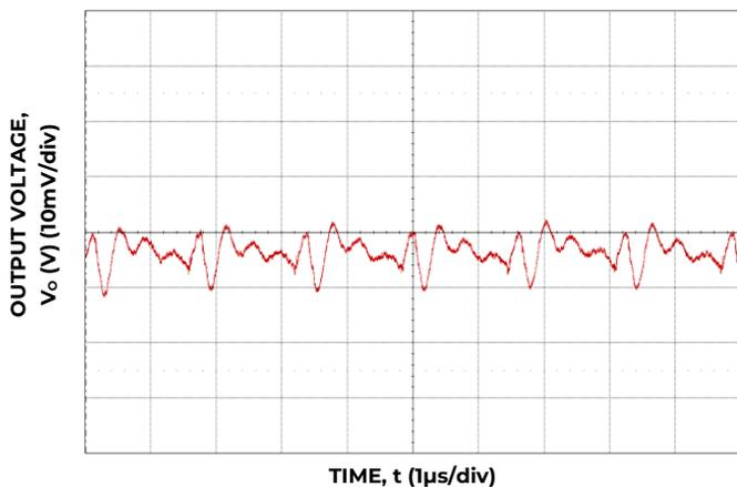
Figure 9. Typical Output Ripple and Noise, (C<sub>o</sub> = 88 μF Ceramic, V<sub>IN</sub> = 12 V, I<sub>o</sub> = I<sub>o, max</sub>.)
