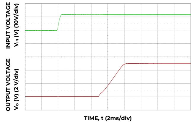
Figure 36. Typical Start-up Using Input Voltage (V<sub>IN</sub> = 12 V, I<sub>o</sub> = I<sub>o, max</sub>.)
