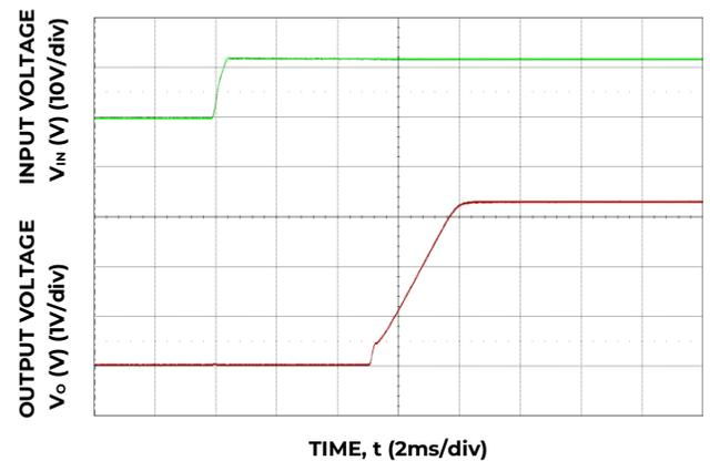
Figure 30. Typical Start-up Using Input Voltage (V<sub>IN</sub> = 12 V, I<sub>o</sub> = I<sub>o, max</sub>.)
