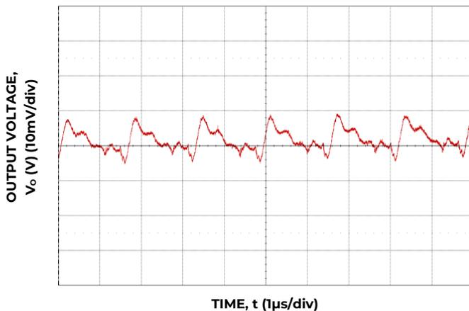
Figure 21. Typical Output Ripple and Noise, (C<sub>o</sub> = 88 μF Ceramic, V<sub>IN</sub> = 12 V, I<sub>o</sub> = I<sub>o, max</sub>.)
