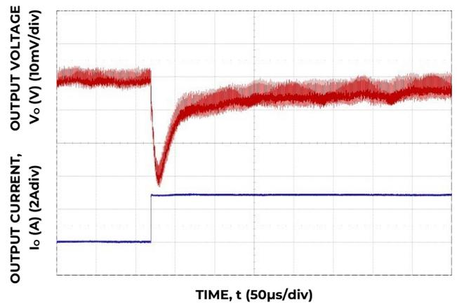
Figure 16. Transient Response to Dynamic Load Change from 50% to 100% at 12V<sub>in</sub>, C<sub>out</sub>-1x330μF, 4x100μF, C<sub>tune</sub>-4.7nF, R<sub>tune</sub>-500
