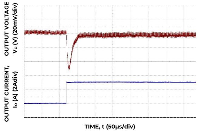
Figure 22. Transient Response to Dynamic Load Change from 50% to 100% at 12V<sub>in</sub>, C<sub>out</sub>-5x100μF, C<sub>tune</sub>-3.3nF, R<sub>tune</sub> - 50Ω
