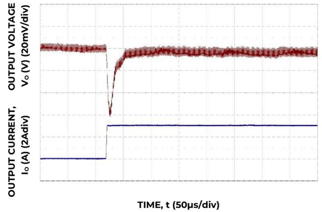
Figure 28. Transient Response to Dynamic Load Change from 50% to 100% at 12V<sub>in</sub>, C<sub>out</sub>-4x100μF, C<sub>tune</sub>-2.2nF, R<sub>tune</sub>-500
