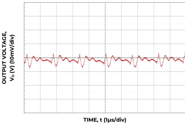
Figure 3. Typical Output Ripple and Noise, (C<sub>o</sub> = 88 μF Ceramic, V<sub>IN</sub> = 12 V I<sub>o</sub> = I<sub>o, max</sub>.)
