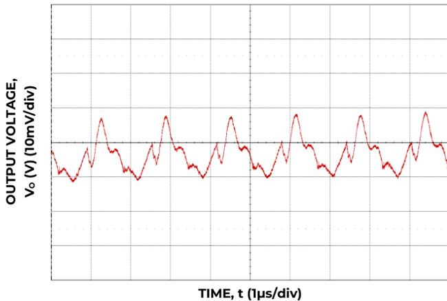
Figure 33. Typical Output Ripple and Noise, (C<sub>o</sub> = 88 µF Ceramic, V<sub>IN</sub> = 12 V, I<sub>o</sub> = I<sub>o, max</sub>.)
