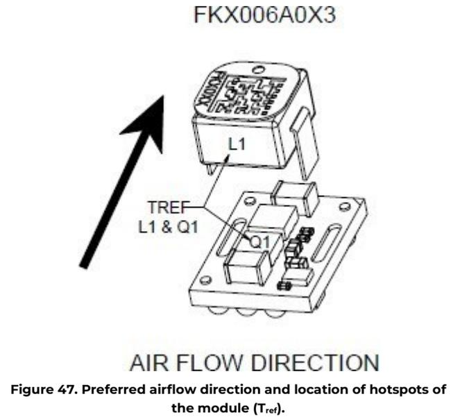
Figure 47. Preferred airflow direction and location of hotspots of the module ( $T_{ref}$ ).
