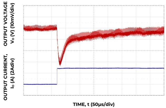
Figure 10. Transient Response to Dynamic Load Change from 50% to 100% at 12V<sub>in</sub>, C<sub>out</sub>-1x330μF, 4x100μF, C<sub>tune</sub>-4.7nF, R<sub>tune</sub>-500
