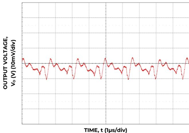
Figure 15. Typical Output Ripple and Noise, (C<sub>o</sub> = 88 μF Ceramic, V<sub>IN</sub> = 12 V, I<sub>o</sub> = I<sub>o, max.</sub>)
