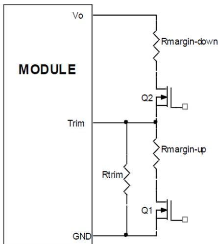
Figure 43. Circuit Configuration for margining Output voltage.
