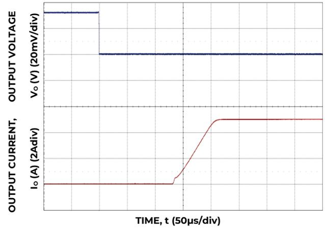
Figure 34. Transient Response to Dynamic Load Change from 5% to 100% at 12 Vin, C<sub>out</sub>- 1x 100µF, C<sub>tune</sub> - 680pF, R<sub>tune</sub>- 500
