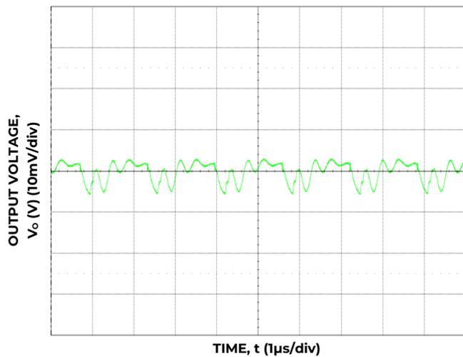
Figure 15. Typical Output Ripple and Noise, (C<sub>o</sub> = 88 µF Ceramic, V<sub>IN</sub> = 12 V, I<sub>o</sub> = I<sub>o,max</sub>.)
