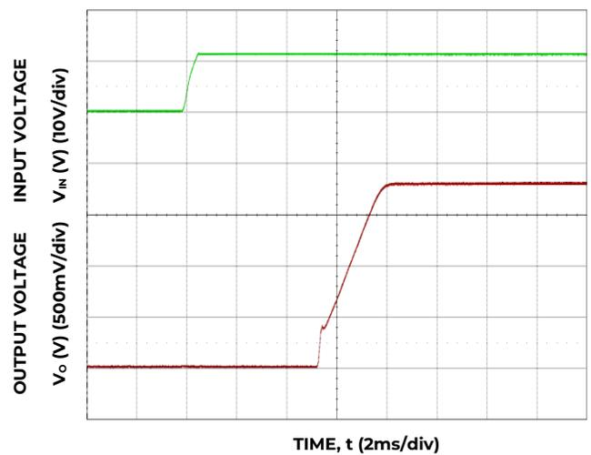
Figure 18. Typical Start-up Using Input Voltage (V<sub>IN</sub> = 12 V, I<sub>o</sub> = I<sub>o,max</sub>.)
