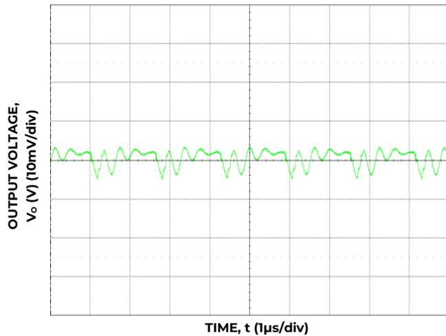
Figure 9. Typical Output Ripple and Noise, (C<sub>o</sub> = 88 µF Ceramic, V<sub>IN</sub> = 12 V I<sub>o</sub> = I<sub>o, max</sub>.)
