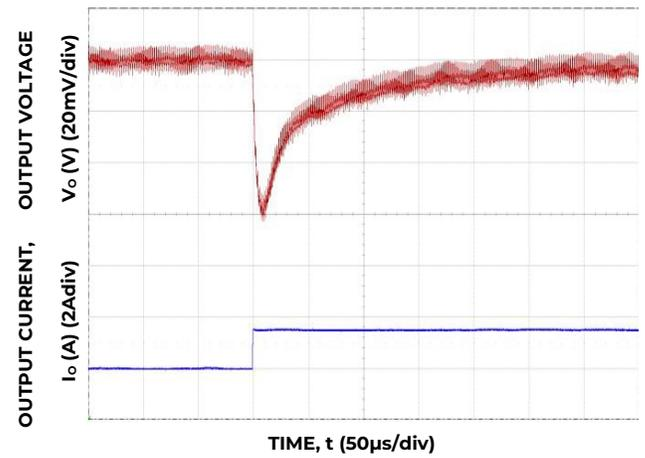
Figure 28. Transient Response to Dynamic Load Change from 5% to 100% at 12 Vin, C<sub>out</sub>–2x 100µF, C<sub>tune</sub> – 1nF, R<sub>tune</sub>– 500
