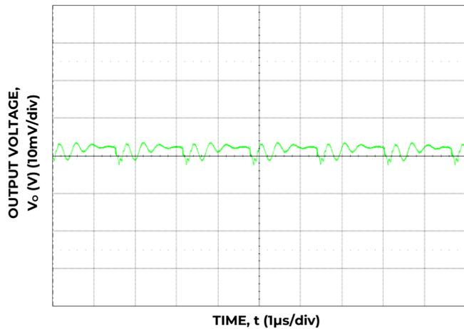
Figure 3. Typical Output Ripple and Noise, (C<sub>o</sub> = 88 µF Ceramic, V<sub>IN</sub> = 12 V I<sub>o</sub> = I<sub>o, max</sub>.)
