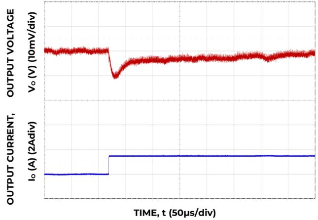
Figure 4. Transient Response to Dynamic Load Change from 5% to 100% at 12 V<sub>in</sub>, C<sub>out</sub>- 2x 330µF, 6x 100µF, C<sub>tune</sub> - 10µF, R<sub>tune</sub>- 500 V<sub>in</sub>=5V.
