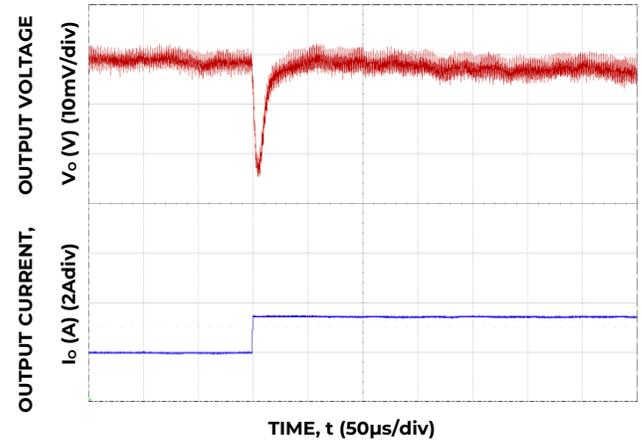
Figure 16. Transient Response to Dynamic Load Change from 5% to 100% at 12 Vin, C<sub>out</sub>- 4x 100µF, C<sub>tune</sub> - 4.7nF, R<sub>tune</sub>- 400
