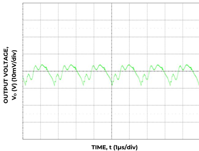
Figure 27. Typical Output Ripple and Noise, (C<sub>o</sub> = 88 µF Ceramic, V<sub>IN</sub> = 12 V, I<sub>o</sub> = I<sub>o, max</sub>.)
