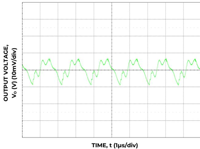
Figure 33. Typical Output Ripple and Noise, ( C<sub>o</sub> = 88 µF Ceramic, V<sub>IN</sub> = 12 V, I<sub>o</sub> = I<sub>o, max</sub>.)
