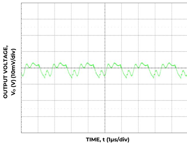
Figure 21. Typical Output Ripple and Noise, ( $C_o = 88 \mu F$  Ceramic,  $V_{IN} = 12 V$ ,  $I_o = I_{o, max.}$ )
