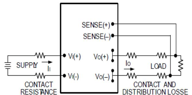
Figure 11. Circuit Configuration for remote sense.
