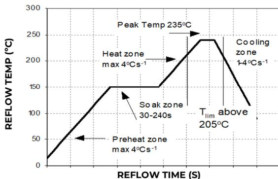
Figure 19. Reflow Profile for Tin/Lead (Sn/Pb) process.
