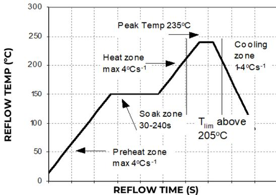
Figure 21. Reflow Profile for Tin/Lead (Sn/Pb) process.
