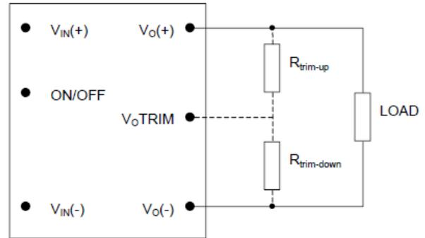
Figure 12. Circuit Configuration to Trim Output Voltage.
