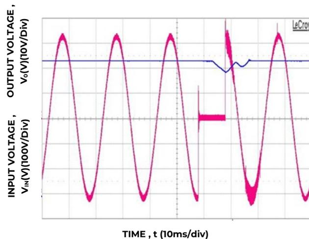
Figure 11. Ride through missing ½ cycle, full load, V<sub>IN</sub> = 230V<sub>AC</sub>.
