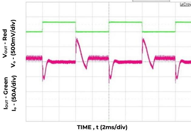
Figure 7. Transient response 52V<sub>DC</sub> load step 10 – 60%, Slew rate: 1A/μs, V<sub>IN</sub> = 230V<sub>AC</sub>
