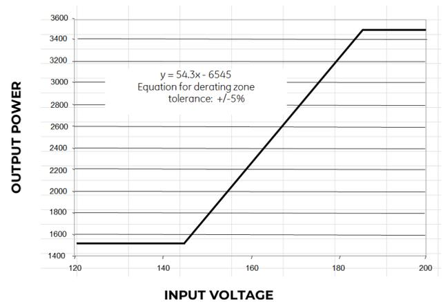
Figure 18. Output power derating below  $V_{IN}$  of 185V<sub>AC</sub>
