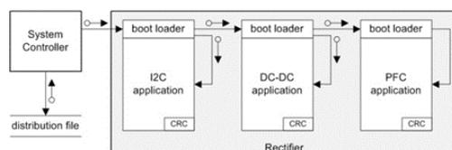
Each of the  $\mu$ Controllers contains a **boot loader** section and an **application** section in memory. The purpose of the boot loader section is to facilitate the upgrading capability described here. All the commands for upgrading and memory space
