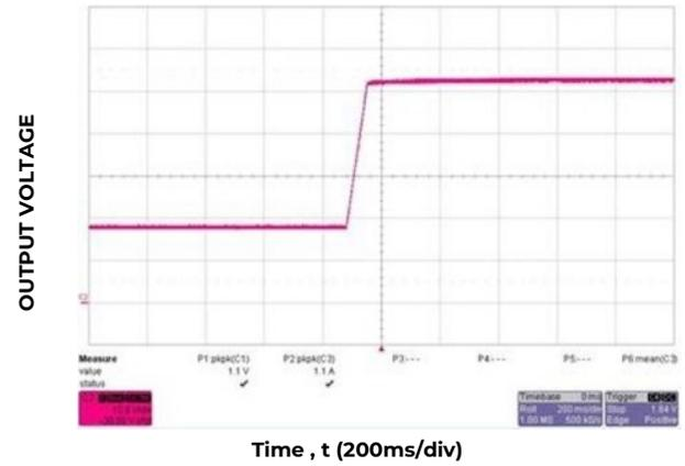
Figure 4. Main output: Output changed from 18V to 52V; commanded via I<sup>2</sup>C
