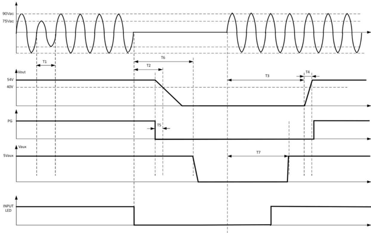
T1 – ride through time – 0.5 to 1 cycles [ 10 – 20ms]  $V_{OUT}$  remains within regulation – load dependent
