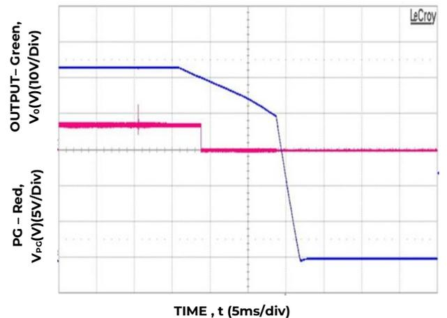
Figure 12 . PG# alarmed 10ms prior to V<sub>o</sub> < 40V, V<sub>IN</sub> = 230V<sub>AC</sub>, Output at Full load
