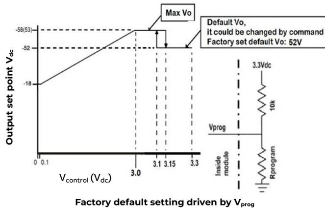
The  $V_{prog}$  pin voltage level, which is referenced to Logic\_GRD, is configured by the user as shown in the graph above. It must be set in order for the rectifier to know what its swtting should be.
