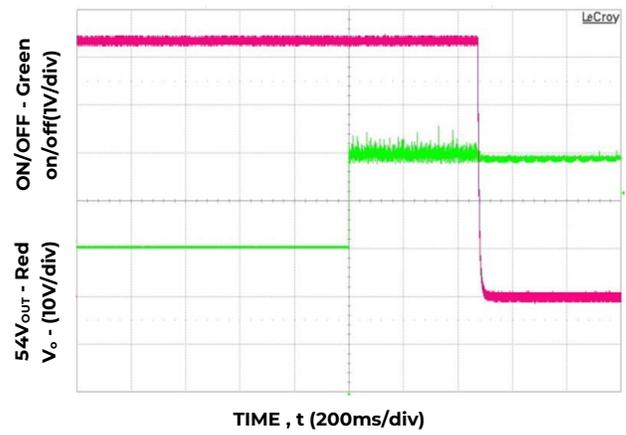
Figure 16. 52V<sub>DC</sub> turn-OFF delay when ON/OFF is di-asserted,  $V_{IN}=230V_{AC}$  - I<sup>2</sup>C mode.
