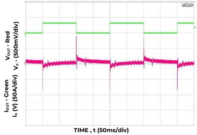
Figure 8. Transient response 52V<sub>DC</sub> load step 10 – 60%, Slew rate: 1A/μs, V<sub>IN</sub> = 230V<sub>AC</sub>
