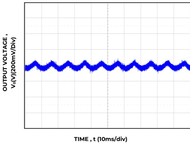
Figure 5. 52V<sub>DC</sub> output ripple and noise, full load,  $V_{IN} = 185V_{AC}$ , 20MHz bandwidth
