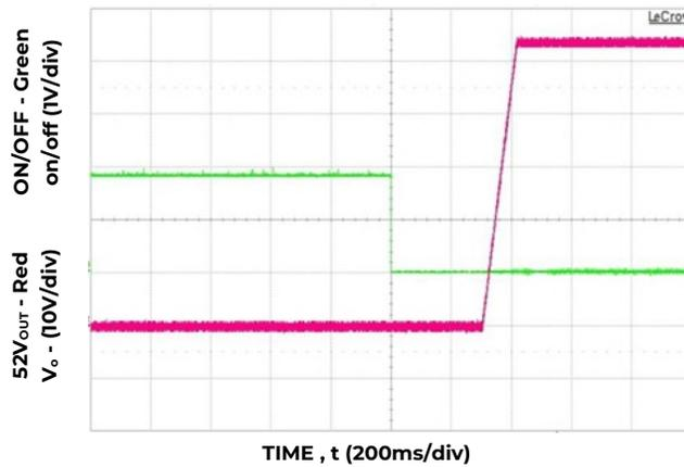
Figure 9. 52V<sub>DC</sub> soft start delay when ON/OFF is asserted, V<sub>IN</sub>=230V<sub>AC</sub> - I<sup>2</sup>C mode.
