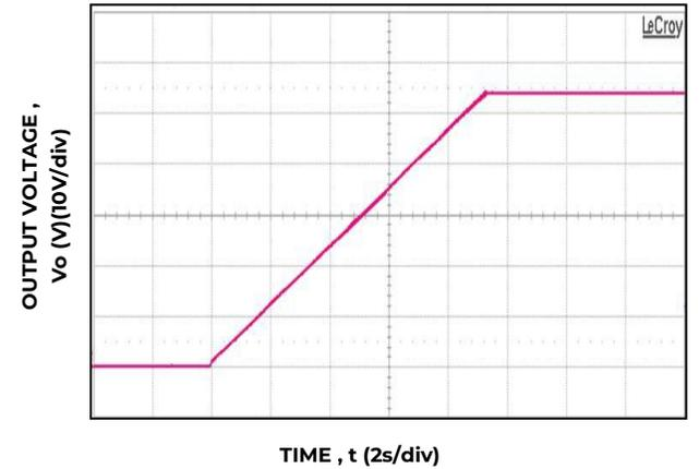
Figure 10. 52V<sub>DC</sub> soft start, full load, V<sub>IN</sub> = 230V<sub>AC</sub> - RS485 mode with 4700μf external capacitance.
