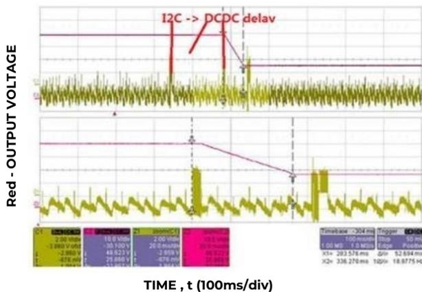
Figure 17. Time delay from sending the I<sup>2</sup>C command and executing the output voltage change.
