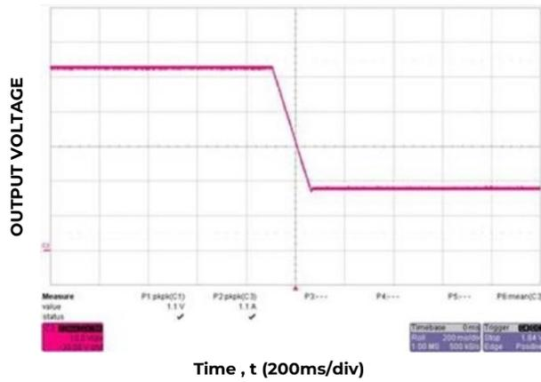
Figure 3. Main output: Output changed from 52V to 18V; commanded via I<sup>2</sup>C.
