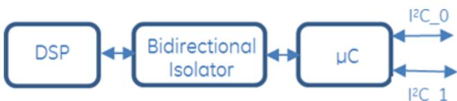
The secondary micro controller is designed to default to I<sup>2</sup>C\_0 when powered up. If only a single system controller is utilized, it should be connected to I<sup>2</sup>C\_0. In this case the I<sup>2</sup>C\_1 line is totally transparent as if it does not exist.
