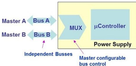
**Figure 2: Diagram showing conceptual representation of the dual I<sup>2</sup>C bus system.**
