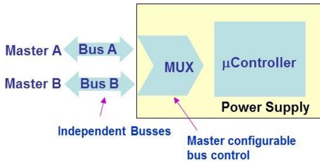
Diagram showing the dual I<sup>2</sup>C bus system.
