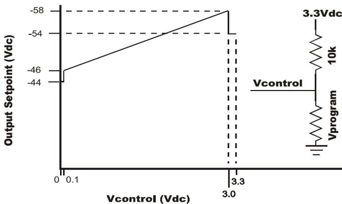
An open circuit on this pin reverts the voltage level back to the original setting..
