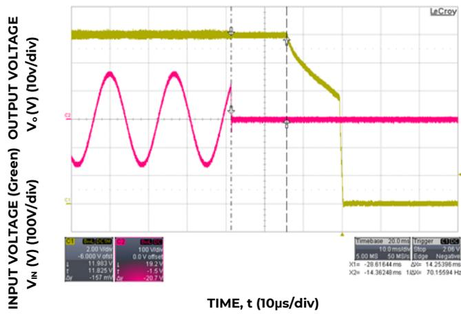
Figure 6. Typical Hold-up Waveforms (V<sub>IN</sub> = 115V<sub>ac</sub>, 100% Load)
