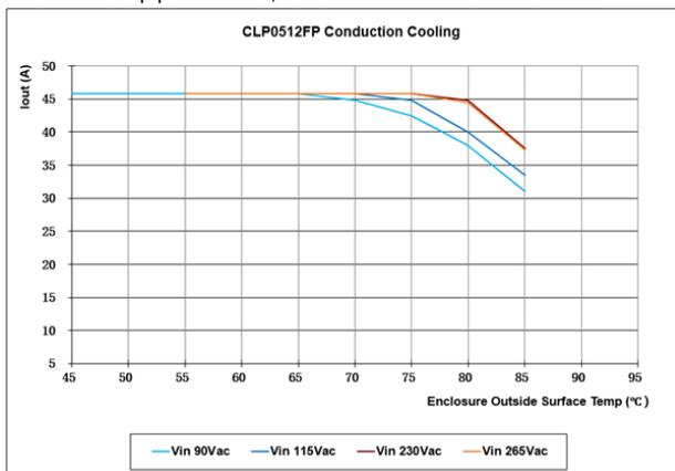
Enclosure Application; with 420W resistive load inside enclosure
