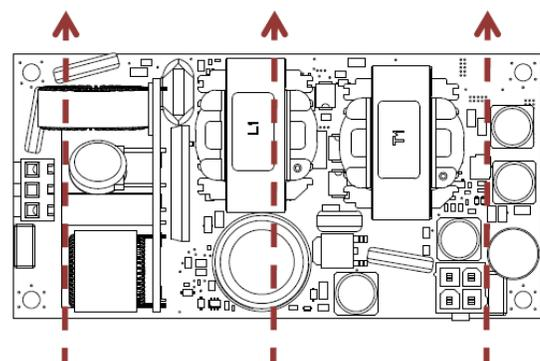
**Fig. 12. Preferred airflow direction for cooling.**
