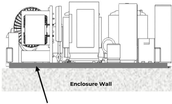
Fig. 13. Example arrangement of the CLP0224 for sealed enclosure applications.
