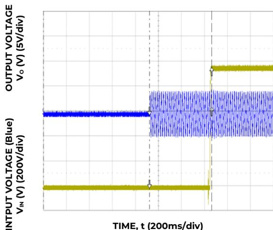
Figure 5. Typical Start-up ( $V_{IN} = 115V_{ac}$ , Full Load).
