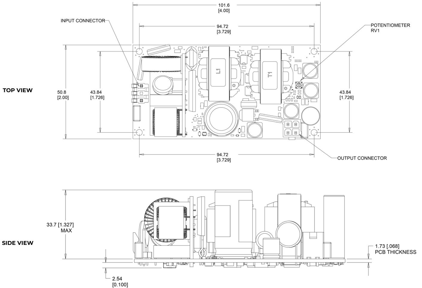
Minimum clearance of 6mm required on bottom of the unit.
