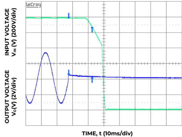
Figure 8. Typical Hold-up waveforms ( $V_{IN} = 230V$ , 100% load).
