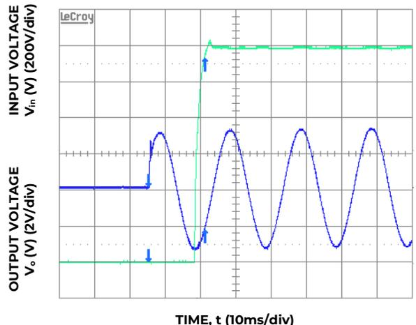
Figure 6. Typical Start-up (V<sub>IN</sub> = 230V<sub>ac</sub>)
