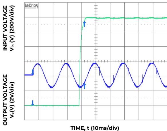
Figure 5. Typical Start-up (V<sub>IN</sub> = 115V<sub>ac</sub>).
