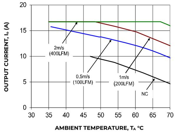
Figure 2. Derating Output Current versus Ambient Temperature and Airflow. Data shown for 115V<sub>AC</sub> in, at 230V<sub>AC</sub> in derating is the same or better. For derating at other input voltages, consult the OmniOn Technical representative.
