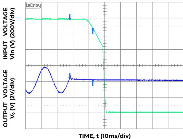
Figure 7. Typical Hold-up waveforms ( $V_{IN} = 115V$ , 100% load).
