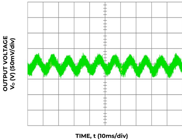
Figure 3. Typical output ripple and noise (V<sub>IN</sub> = 230V<sub>ac</sub>, 100% load).
