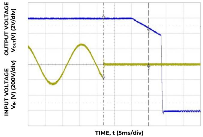
Figure 10. Hold-up ( $V_{IN} = 230V$ ,  $I_o = 80\% I_{o,max}$ ).
