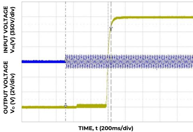
Figure 7. Start-up ( $V_{IN} = 90V$ ,  $I_o = I_{o,max}$ ).
