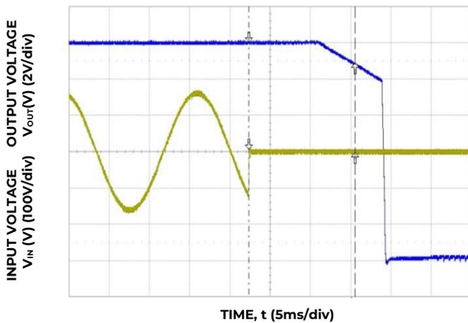
Figure 9. Hold-up ( $V_{IN} = 115V$ ,  $I_o = 80\% I_{o,max}$ ).
