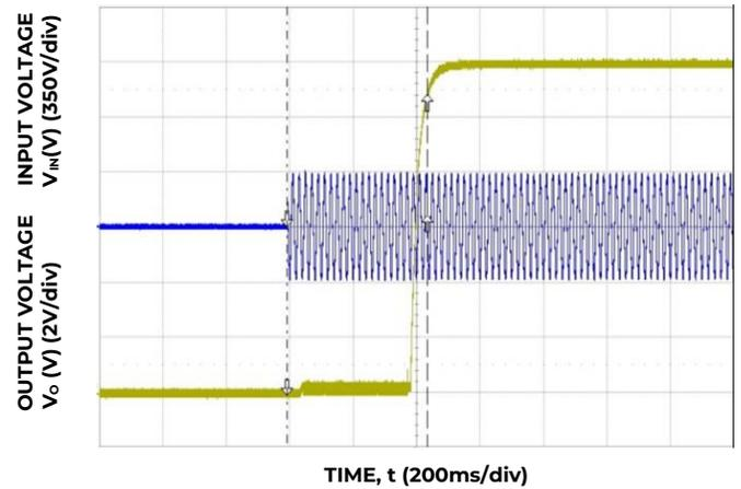
Figure 8. Start-up ( $V_{IN} = 264V$ ,  $I_o = I_{o,max}$ ).
