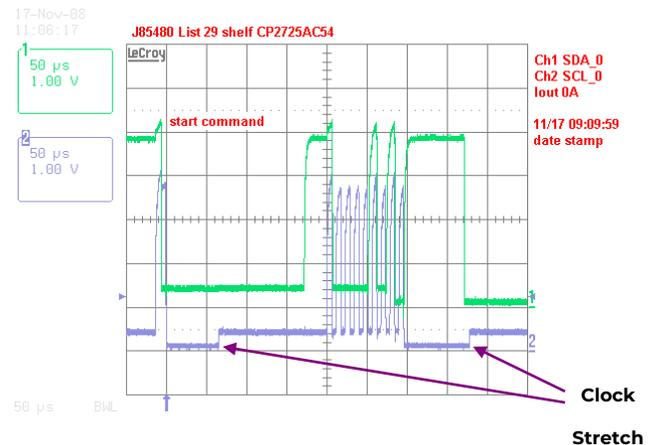
Figure 1. Example waveforms showing clock stretching.
