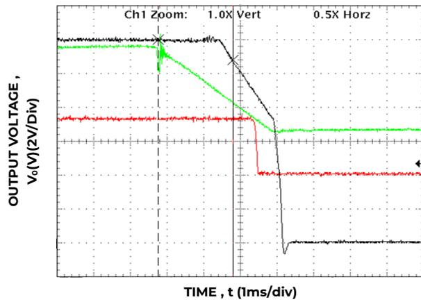
Figure 9. 12V holdup time , full load ,  $V_{IN} = -48V_{DC}$
