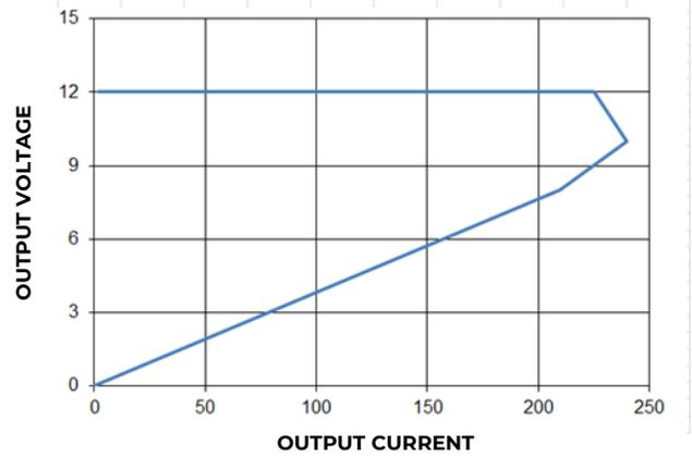
Figure 2. 12V output : Current limit profile ( $V_{in} : -48V_{DC}$ )
