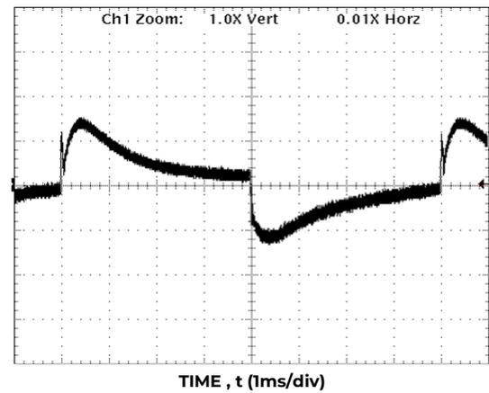
Figure 8. 12V Transient response 100 – 200A,  $V_{IN} = -48V_{DC}$
