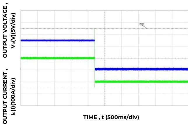
Figure 11. Overload: output short circuit performance,
