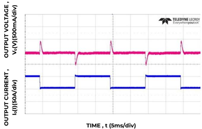
Figure 8. Transient response 12V<sub>DC</sub> output load step
