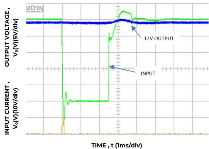
Figure 12. Ride through: full load V<sub>in</sub> = -48V<sub>DC</sub>
