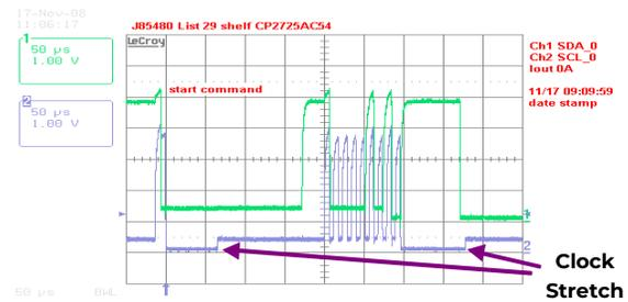
Figure 1 . Example waveforms showing clock stretching
