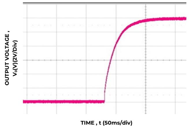
Figure 4. 12V start-up ( $V_{in} : -48V_{DC}$ , full load)
