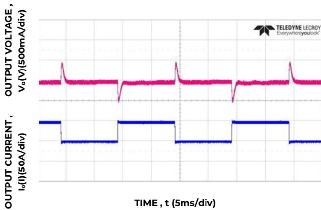
Figure 7. Transient response 12V<sub>DC</sub> output load step
