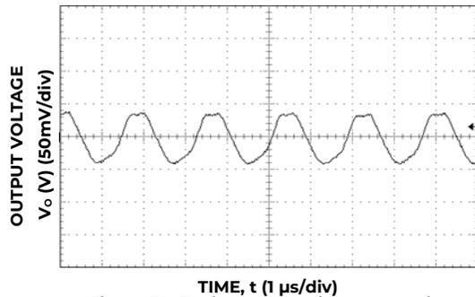
Figure 39. Typical output ripple and noise (V<sub>IN</sub> = 12V, I<sub>o</sub> = I<sub>o,max</sub>).
