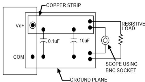
**Figure 50. Output Ripple and Noise Test Setup.**
