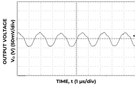
Figure 33. Typical output ripple and noise (V<sub>IN</sub> = 12V, I<sub>o</sub> = I<sub>o,max</sub>).
