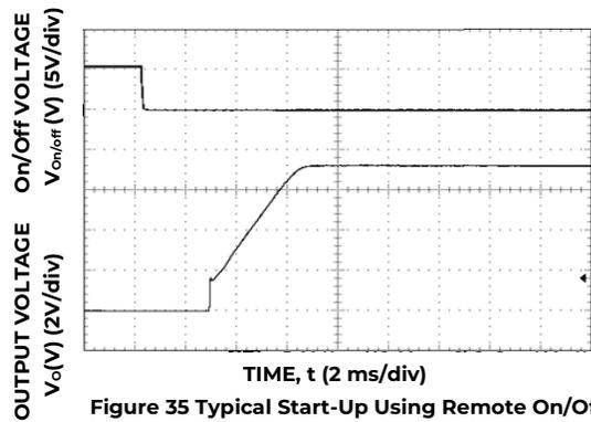
Figure 35 Typical Start-up Using Remote On/Off Voltage (I<sub>o</sub> = I<sub>o,max</sub>).
