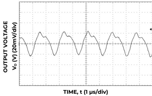
Figure 21. Typical output ripple and noise (V<sub>IN</sub> = 12V, I<sub>o</sub> = I<sub>o,max</sub>).
