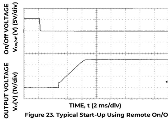
Figure 23. Typical Start-up Using Remote On/Off Voltage (I<sub>o</sub> = I<sub>o,max</sub>).
