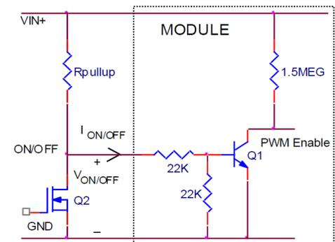
**Figure 55. Circuit configuration for using negative On/Off logic**
