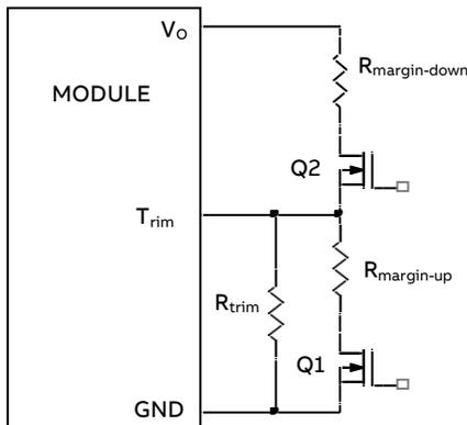
Figure 58. Circuit configuration for margining output voltage
