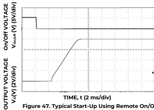
Figure 47. Typical Start-up Using Remote On/Off Voltage (Io = Io,max).
