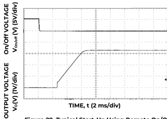
Figure 29. Typical Start-Up Using Remote On/Off Voltage (I<sub>o</sub> = I<sub>o,max</sub>).
