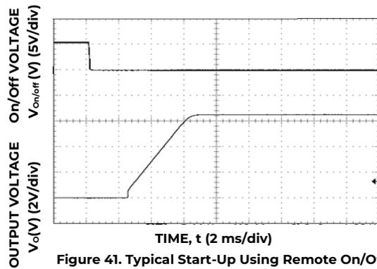
Figure 41. Typical Start-up Using Remote On/Off Voltage (I<sub>o</sub> = I<sub>o,max</sub>).
