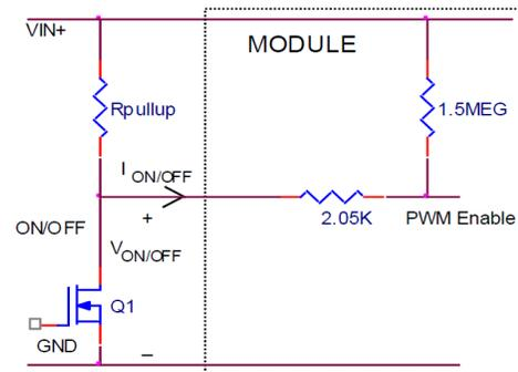
**Figure 54. Circuit configuration for using positive On/Off logic**
