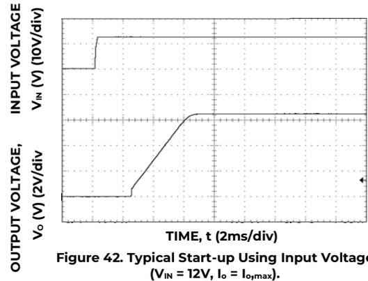
Figure 42. Typical Start-up Using Input Voltage (V<sub>IN</sub> = 12V, I<sub>o</sub> = I<sub>o,max</sub>).
