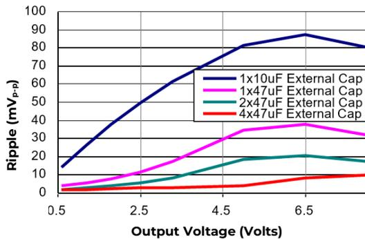
**Figure 53. Output ripple voltage for various output voltages with 1x10  $\mu$ F, 1x47  $\mu$ F or 2x47  $\mu$ F or 4x47  $\mu$ F ceramic capacitors at the output (4A load). Input voltage is 12V.**
