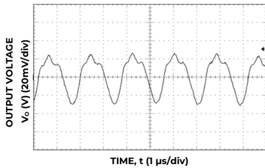
Figure 27. Typical output ripple and noise (V<sub>IN</sub> = 12V, I<sub>o</sub> = I<sub>o,max</sub>).
