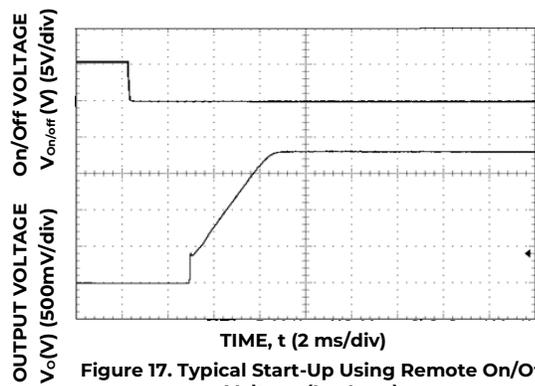
Figure 17. Typical Start-Up Using Remote On/Off Voltage (I<sub>o</sub> = I<sub>o,max</sub>).
