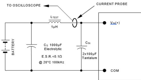
**Figure 49. Input Reflected Ripple Current Test Setup.**
