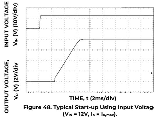
Figure 48. Typical Start-up Using Input Voltage (VIN = 12V, Io = Io,max).
