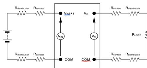
**Figure 51. Output Voltage and Efficiency Test Setup.**
