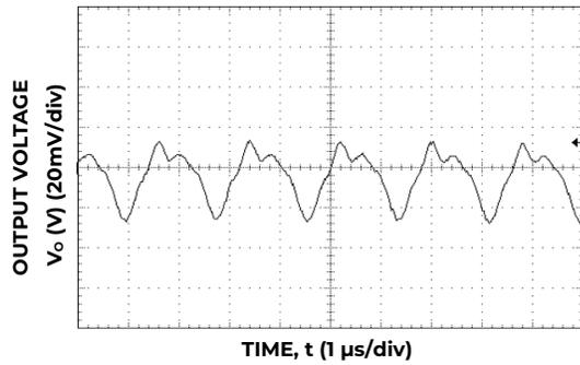
Figure 15. Typical output ripple and noise (V<sub>IN</sub> = 12V, I<sub>o</sub> = I<sub>o,max</sub>).
