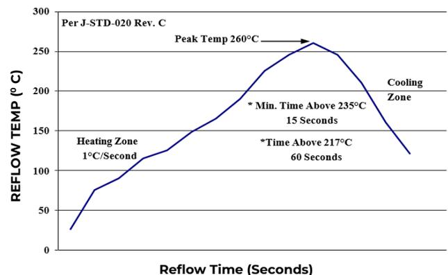
Figure 50. Recommended linear reflow profile using Sn/Ag/Cu solder.
