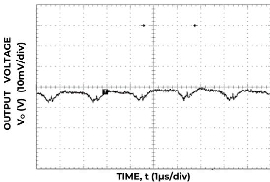
Figure 3. Typical Output Ripple and noise, V<sub>IN</sub> = 12 V ( I<sub>o</sub> = I<sub>o,max</sub> )
