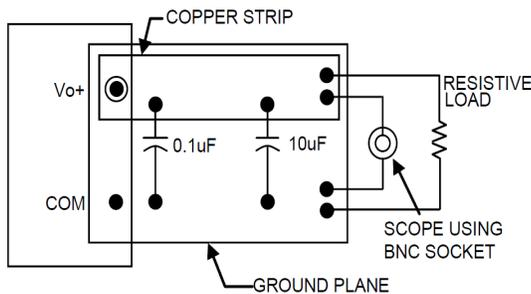
**Figure 38. Output Ripple and Noise Test Setup.**
