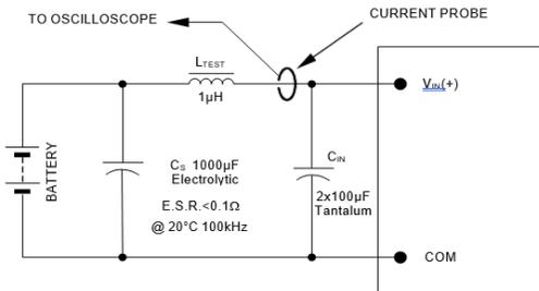
**Figure 37. Input Reflected Ripple Current Test Setup.**
