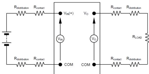
**Figure 39. Output Voltage and Efficiency Test Setup.**
