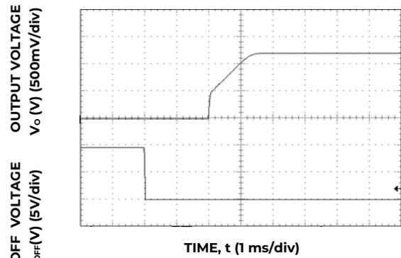
Figure 11. Typical Start-up Using On/Off Voltage (I<sub>o</sub> = I<sub>o, max</sub>).
