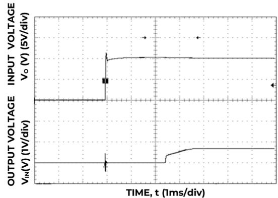
Figure 6. Typical Start-up Using Input Voltage ( V<sub>IN</sub> = 10V, I<sub>o</sub> = I<sub>o,max</sub> )
