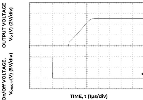
Figure 33. Typical Start-up Using On/Off Voltage (I<sub>o</sub> = I<sub>o, max</sub>).
