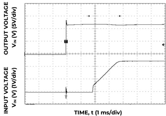
Figure 24. Typical Start-up Using Input Voltage (V<sub>IN</sub> = 12V, Io = Io, max.)
