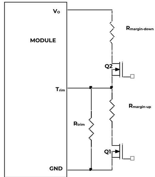
Figure 46. Circuit configuration for margining output voltage
