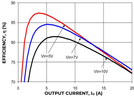
Figure 1. Converter Efficiency versus Output Current .
