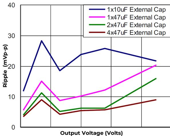
**Figure 41. Output ripple voltage for various output voltages with external 1x10  $\mu$ F, 1x47  $\mu$ F, 2x47  $\mu$ F or 4x47  $\mu$ F ceramic capacitors at the output (20A load). Input voltage is 12V**
