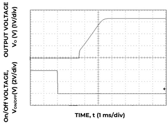
Figure 29. Typical Start-up Using On/Off Voltage (I<sub>o</sub> = I<sub>o, max</sub>).
