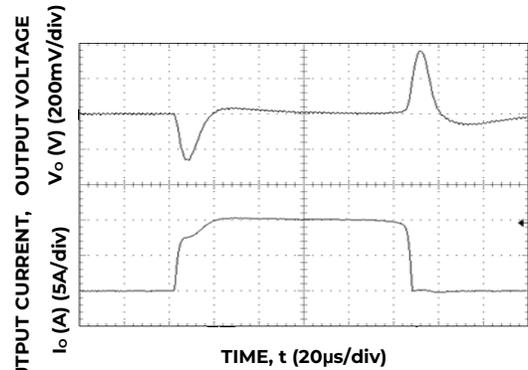
Figure 10. Transient Response to Dynamic Load Change from 50% to 100% of I<sub>o</sub>.
