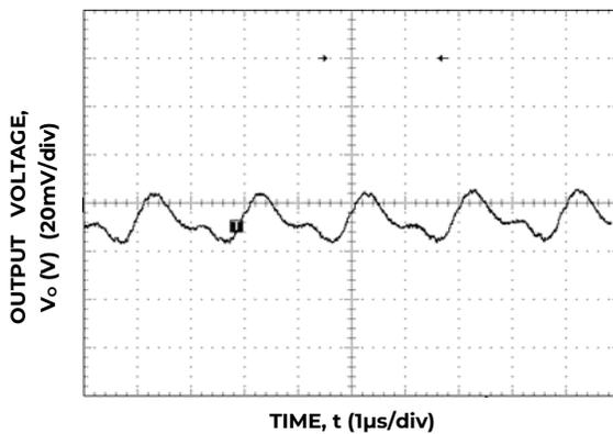
Figure 21. Typical Output ripple and noise, V<sub>IN</sub> = 12 V Io = Io, max.
