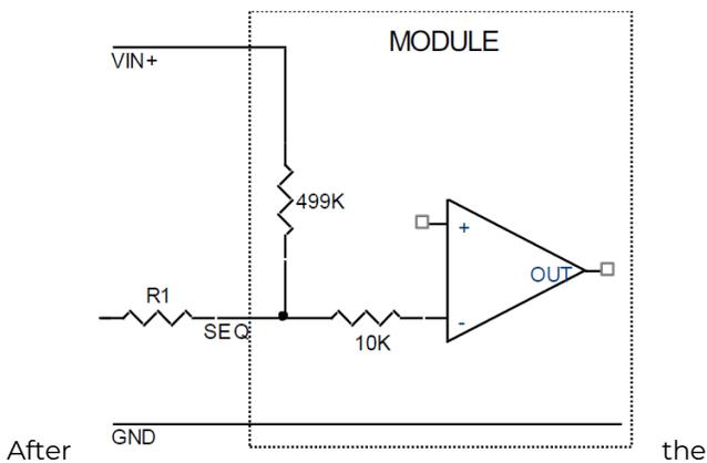
After the **Figure 47. Circuit showing connection of the sequencing signal to the SEQ pin.**
