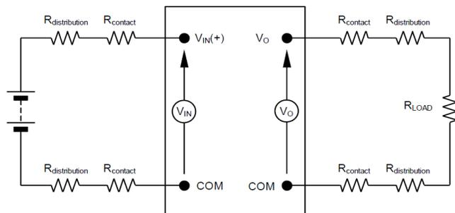
**Figure 39. Output Voltage and Efficiency Test Setup.**
