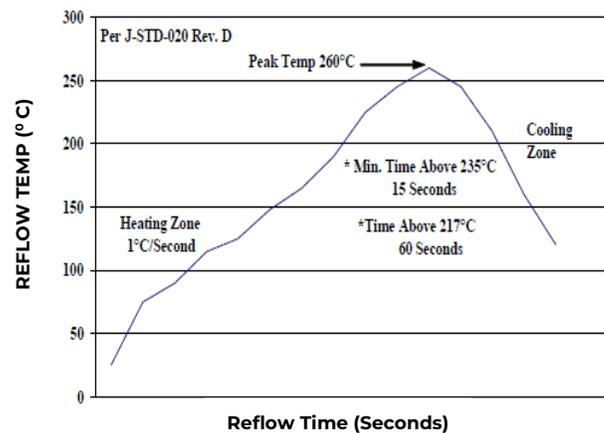
Figure 51. Recommended linear reflow profile using Sn/Ag/Cu solder.
