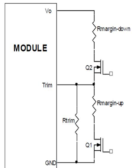
Figure 46. Circuit Configuration for margining Output voltage.
