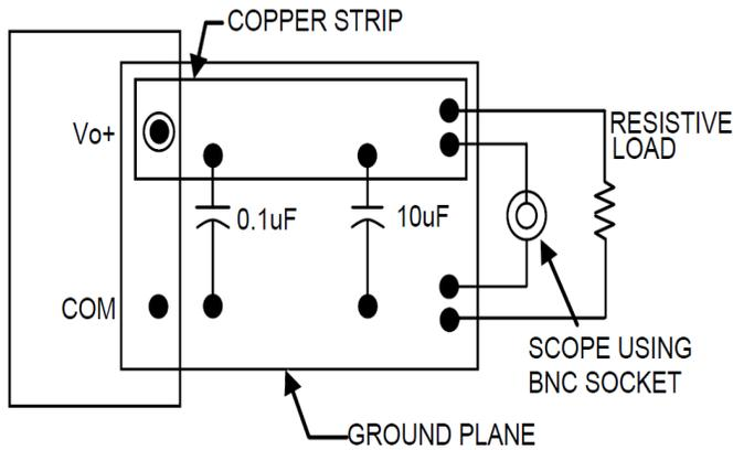
**Figure 38. Output Ripple and Noise Test Setup.**
