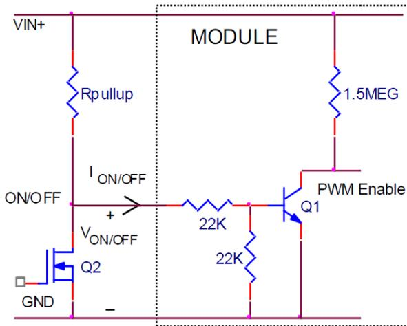
**Figure 43. Circuit configuration for using negative On/Off logic.**
