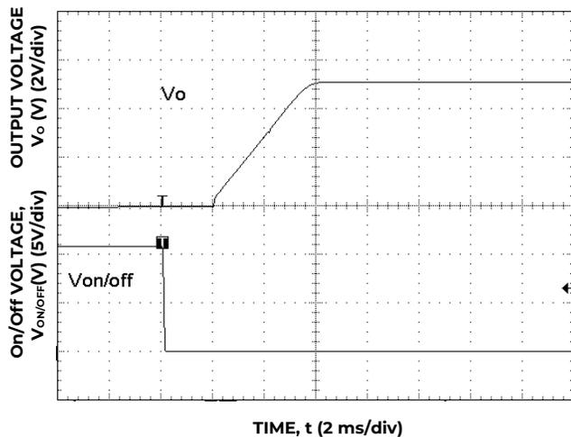
Figure 33. Typical Start-up Using On/Off Voltage (I<sub>o</sub> = I<sub>o, max</sub>).
