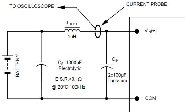
**Figure 37. Input Reflected Ripple Current Test Setup.**
