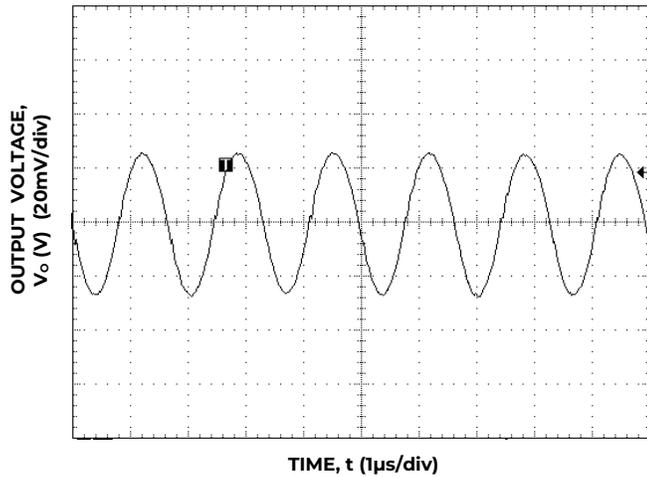
Figure 32. Typical Output Ripple and Noise, V<sub>IN</sub> = 12 V I<sub>o</sub> = I<sub>o, max</sub>.
