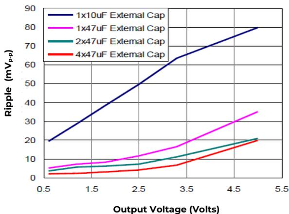
**Figure 41. Output ripple voltage for various output voltages with external 1x10  $\mu$ F, 1x47  $\mu$ F, 2x47  $\mu$ F or 4x47  $\mu$ F ceramic capacitors at the output (6A load). Input voltage is 12V.**
