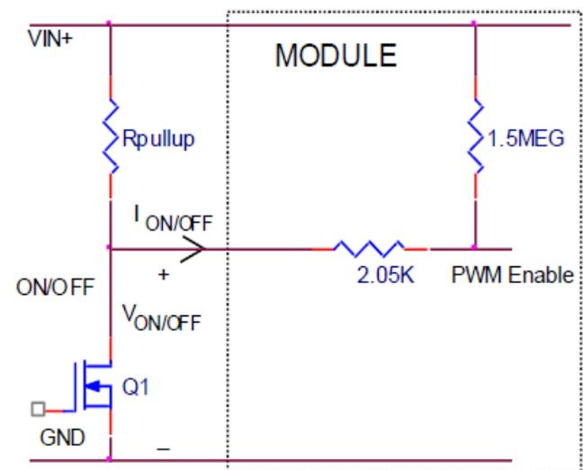
**Figure 42. Circuit configuration for using positive On/Off logic.**
