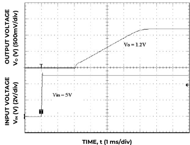
Figure 12. Typical Start-up Using Input Voltage ( $V_{IN} = 5V$   $I_o = I_{o,max}$ ).
