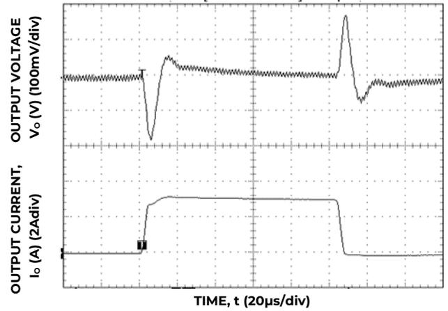
Figure 16. Transient Response to Dynamic Load Change from 0% to 50% to 0% with V<sub>IN</sub> = 5V
