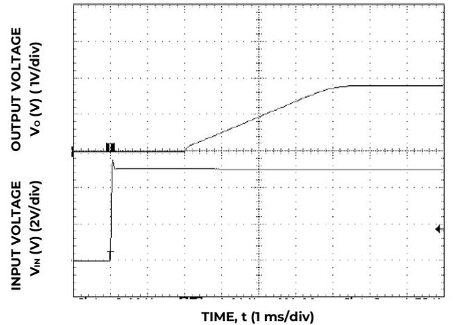
Figure 18. Typical Start-up Using Input Voltage (V<sub>IN</sub> = 5V I<sub>o</sub> = I<sub>o, max</sub>).
