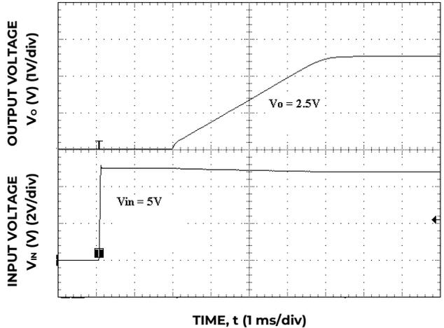
Figure 24. Typical Start-up Using Input Voltage (V<sub>IN</sub> = 5 V, I<sub>o</sub> = I<sub>o, max</sub>).
