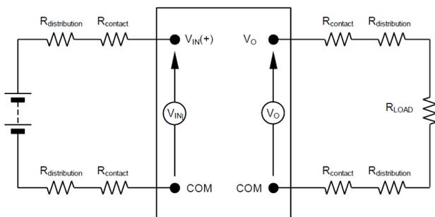
**Figure 33. Output Voltage and Efficiency Test Setup.**
