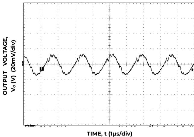
Figure 21. Typical Output ripple and noise, V<sub>IN</sub> = 5 V I<sub>o</sub> = I<sub>o, max</sub>.
