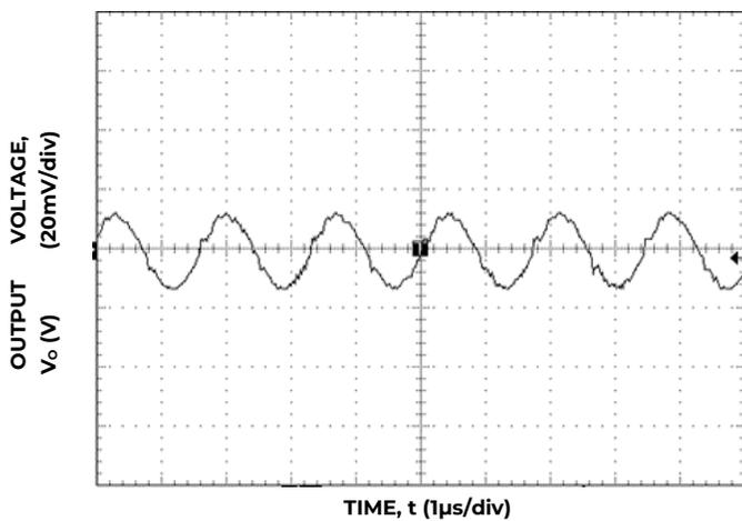
Figure 15. Typical Output ripple and noise, V<sub>IN</sub> = 5V I<sub>o</sub> = I<sub>o, max</sub>.
