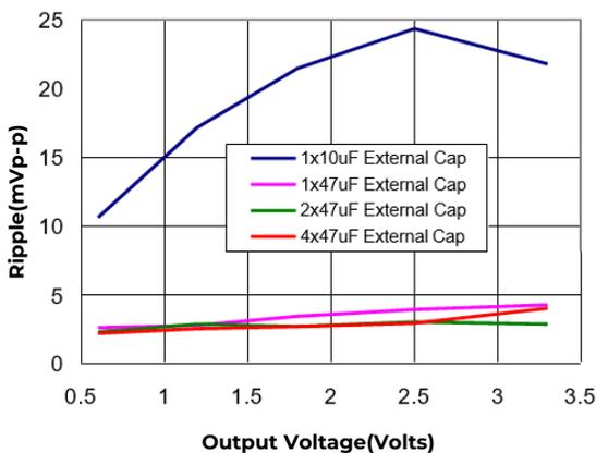
**Figure 36. Output ripple voltage for various output voltages with external 1x10  $\mu\text{F}$ , 1x47  $\mu\text{F}$ , 2x47  $\mu\text{F}$  or 4x47  $\mu\text{F}$  ceramic capacitors at the output (6A load). Input voltage is 5V.**
