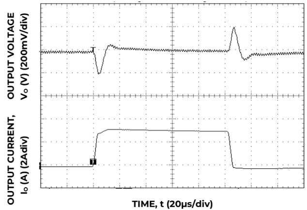
Figure 22. Transient Response to Dynamic Load Change from 0% to 50% to 0% with V<sub>IN</sub>=5V
