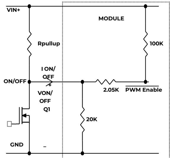
Figure 39. Circuit configuration for using negative On/Off logic.
