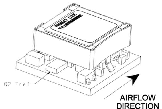
**Figure 46. Preferred airflow direction and location of hotspot of the module (T<sub>ref</sub>).**
