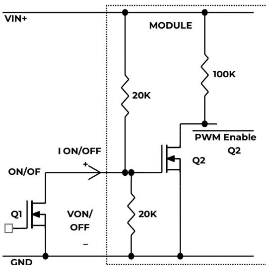
Figure 38. Circuit configuration for using positive On/Off logic.
