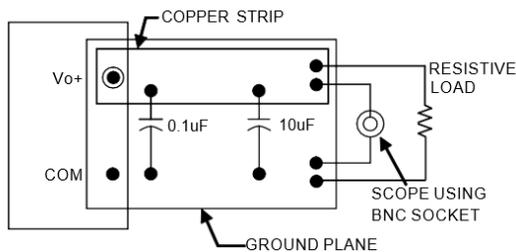
**Figure 32. Output Ripple and Noise Test Setup.**
