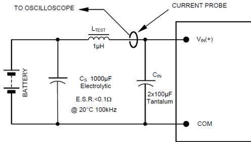
**Figure 31. Input Reflected Ripple Current Test Setup.**
