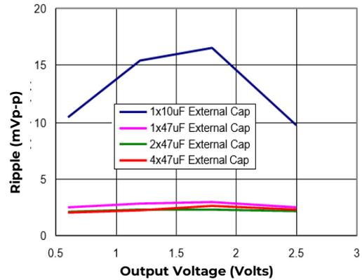
**Figure 37. Output ripple voltage for various output voltages with external 1x10  $\mu\text{F}$ , 1x47  $\mu\text{F}$ , 2x47  $\mu\text{F}$  or 4x47  $\mu\text{F}$  ceramic capacitors at the output (6A load). Input voltage is 3.3V.**
