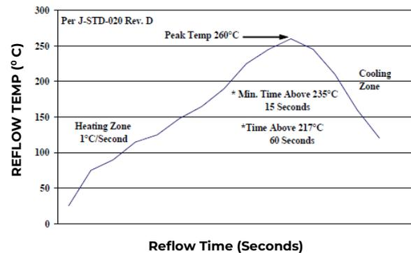
Figure 47. Recommended linear reflow profile using Sn/Ag/Cu solder.
