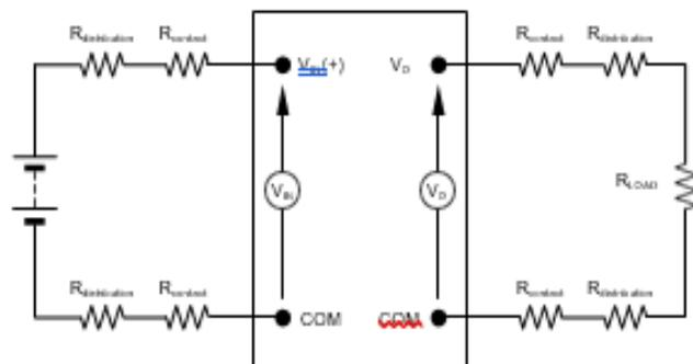
**Figure 33. Output Voltage and Efficiency Test Setup.**
