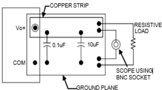
**Figure 32. Output Ripple and Noise Test Setup.**
