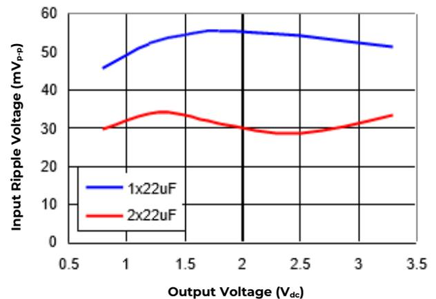
**Figure 34. Input ripple voltage for various output voltages with  $1 \times 22\mu F$  or  $2 \times 22\mu F$  ceramic capacitors at the input (3A load). Input voltage is 5V.**
