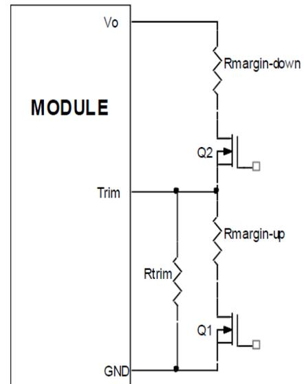
Figure 41. Circuit Configuration for margining Output voltage
