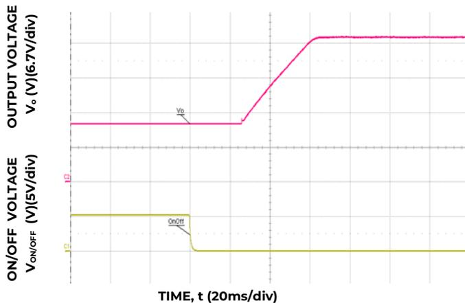
Figure 17. Typical Start-up Using On/Off Voltage (I<sub>o</sub> = I<sub>o,max</sub>)
