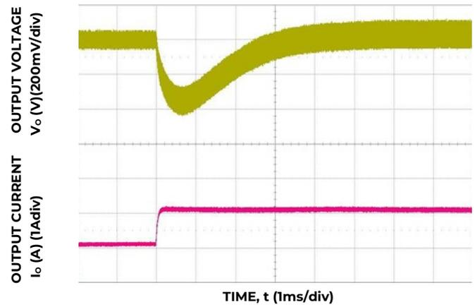
Figure 16. Transient Response to Dynamic Load Change from 50% to 100% at 12V<sub>in</sub>, C<sub>OUT</sub> = 9x10uF, C<sub>Tune</sub>=3300pF, R<sub>Tune</sub>=30.1Ω
