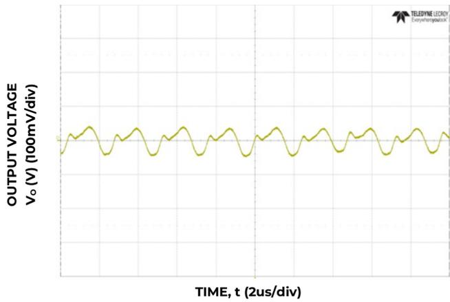
Figure 3. Typical output ripple (C<sub>o</sub>=66μF ceramic, V<sub>IN</sub> = 12V, I<sub>o</sub> = I<sub>o, max</sub>)
