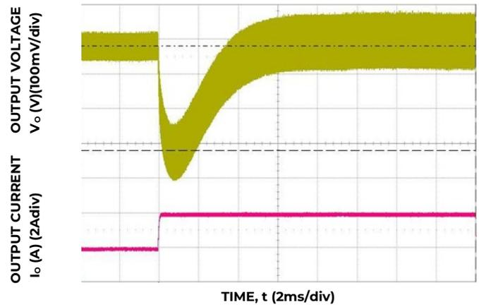
Figure 4. Transient Response to Dynamic Load Change from 50% to 100% at 12V<sub>IN</sub>, C<sub>OUT</sub>= 3x10uF+220uF, CTune=6800pF, RTune=30.1Ω
