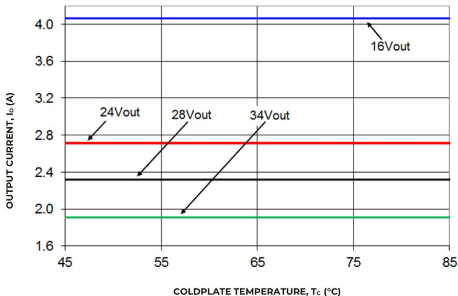
Figure 34. Output Current versus ColdWall Temperature;  $V_{IN}=12V$ .
