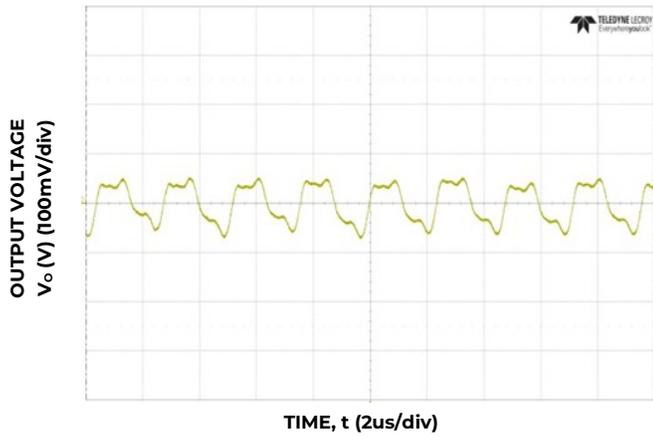
Figure 9. Typical output ripple
