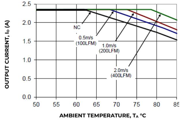
Figure 14. Derating Output Current versus Ambient Temperature and Airflow. V<sub>IN</sub> = 12V
