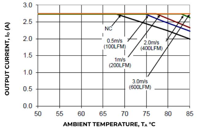
Figure 8. Derating Output Current versus Ambient Temperature and Airflow, V<sub>IN</sub>=12V
