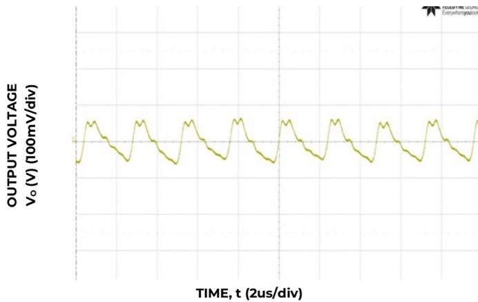
Figure 21. Typical output ripple and noise (C<sub>O</sub>=66µF ceramic, V<sub>IN</sub> = 12V, I<sub>o</sub> = I<sub>o,max</sub>)
