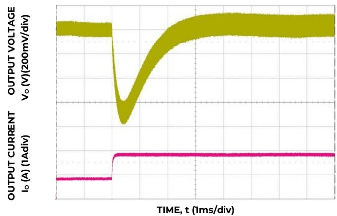
Figure 22. Transient Response to Dynamic Load Change from 0.9 to 1.9A at 12V<sub>IN</sub>, C<sub>OUT</sub>= 9x10uF CTune=1000pF, RTune=30.1Ω
