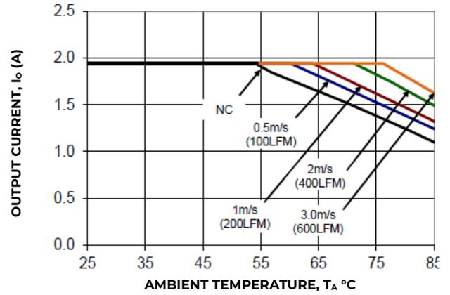
Figure 20. Derating Output Current versus Ambient Temperature and Airflow. V<sub>IN</sub> = 12V
