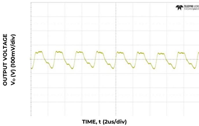
Figure 15. Typical output ripple (C<sub>o</sub>=66μF ceramic, V<sub>IN</sub> = 12V, I<sub>o</sub> = I<sub>o,max</sub>)
