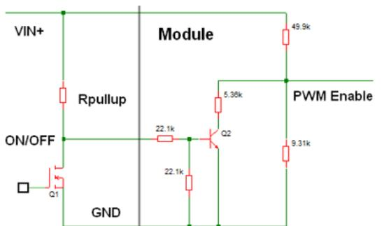
Figure 27. Circuit configuration for using negative On/Off logic.
