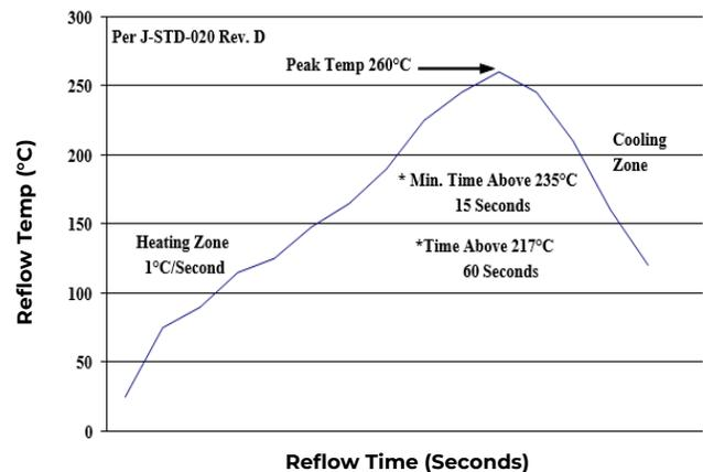
Figure 35. Recommended linear reflow profile using Sn/Ag/Cu solder.
