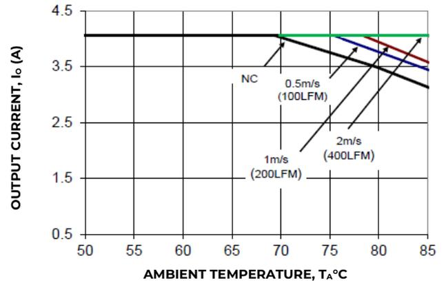
Figure 2. Derating Output Current versus Ambient Temperature and Airflow, V<sub>IN</sub> = 10V
