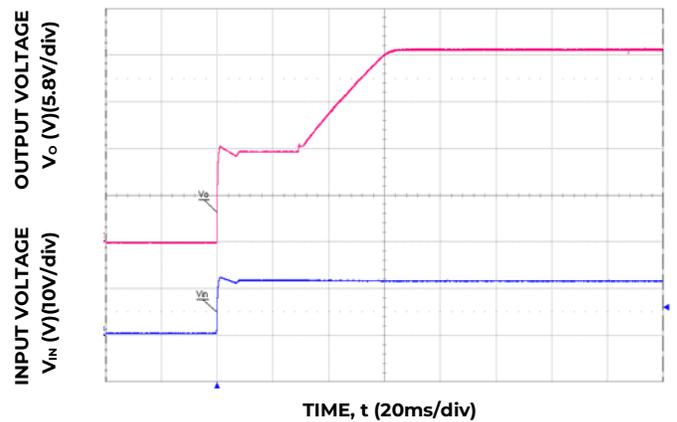
Figure 12. Typical Start-up Using Input Voltage (V<sub>IN</sub> = 12V, I<sub>o</sub> = I<sub>o,max</sub>)
