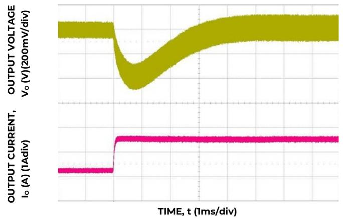
Figure 10. Transient Response to Dynamic Load Change from 50 % to 100% at 12V<sub>IN</sub>, C<sub>OUT</sub> = 3x10uF+220uF, CTune=3300pF, RTune=30.1kΩ
