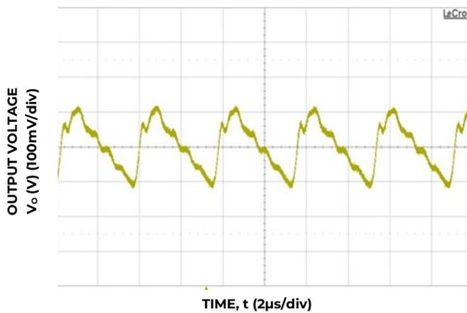
Figure 9. Typical output ripple and noise (C<sub>o</sub>=66µF ceramic, V<sub>IN</sub>=12V, I<sub>o</sub> = I<sub>o,max</sub>).
