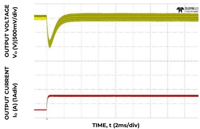
Figure 10. Transient Response to Dynamic Load Change from 0.6 to 1.6A at 12Vin, C<sub>out</sub>=10x4.7µF, C<sub>Tune</sub>=560pF, R<sub>Tune</sub>=40.2k
