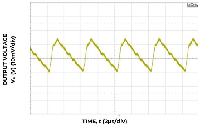
Figure 15. Typical output ripple and noise (C<sub>o</sub>=66µF ceramic, V<sub>IN</sub> = 12V, I<sub>o</sub> = I<sub>o,max</sub>).
