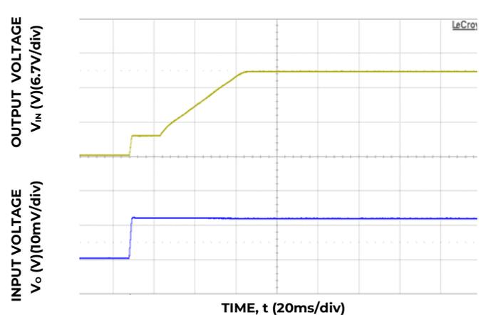
Figure 18. Typical Start-up Using Input Voltage (V<sub>IN</sub> = 12V, I<sub>o</sub> = I<sub>o,max</sub>).
