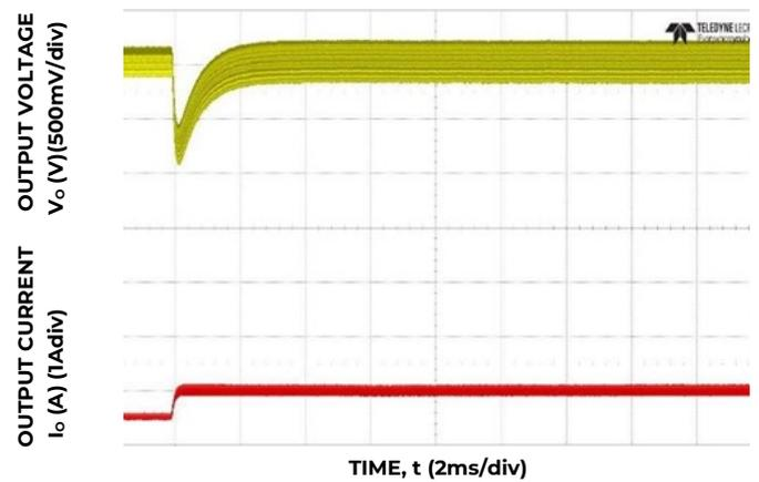
Figure 22. Transient Response to Dynamic Load Change from 0.6 to 1.1A at 12V<sub>in</sub>, C<sub>out</sub>= 7x4.7μF C<sub>Tune</sub>=82pF, R<sub>Tune</sub>=40.2Ω
