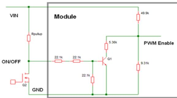
Figure 28. Circuit configuration for using negative On/Off logic.
