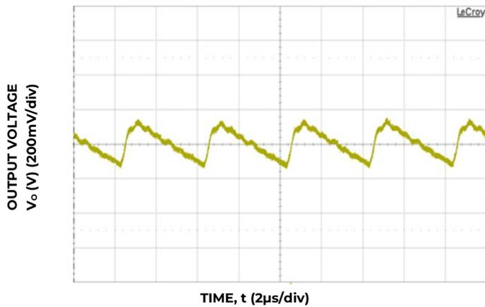
Figure 21. Typical output ripple and noise (C<sub>o</sub>=66μF ceramic, V<sub>IN</sub> = 12V, I<sub>o</sub> = I<sub>o,max</sub>).
