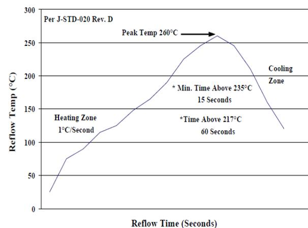
Figure 35. Recommended linear reflow profile using Sn/Ag/Cu solder.
